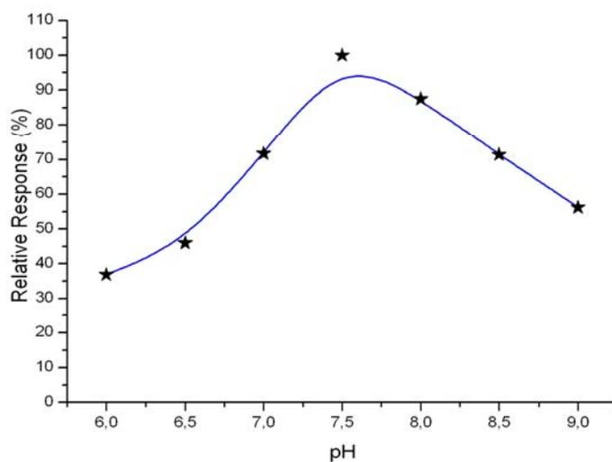
**Fig. 5.** Influence of pH values on the activity of the enzyme electrode in the presence of 10 mM H<sub>2</sub>O<sub>2</sub> in PBS solution. Data collected with freshly prepared enzyme electrodes refer to the average of three experiments
