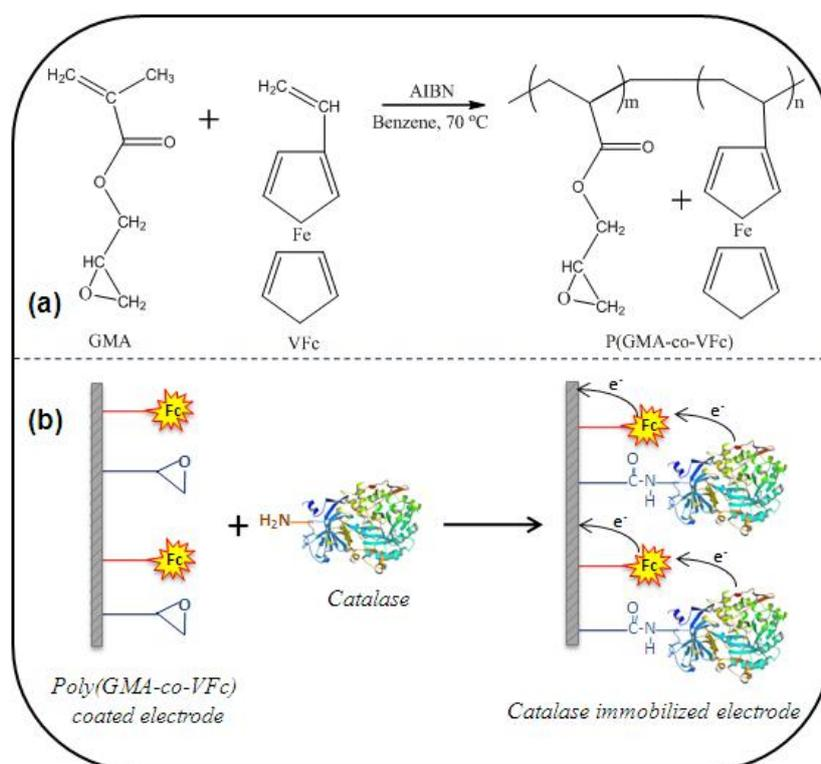
**Fig. 1.** (a) Preparation of poly (GMA-co-VFc) and (b) immobilization of enzyme via amine group onto Poly (GMA-co-VFc) film electrode
