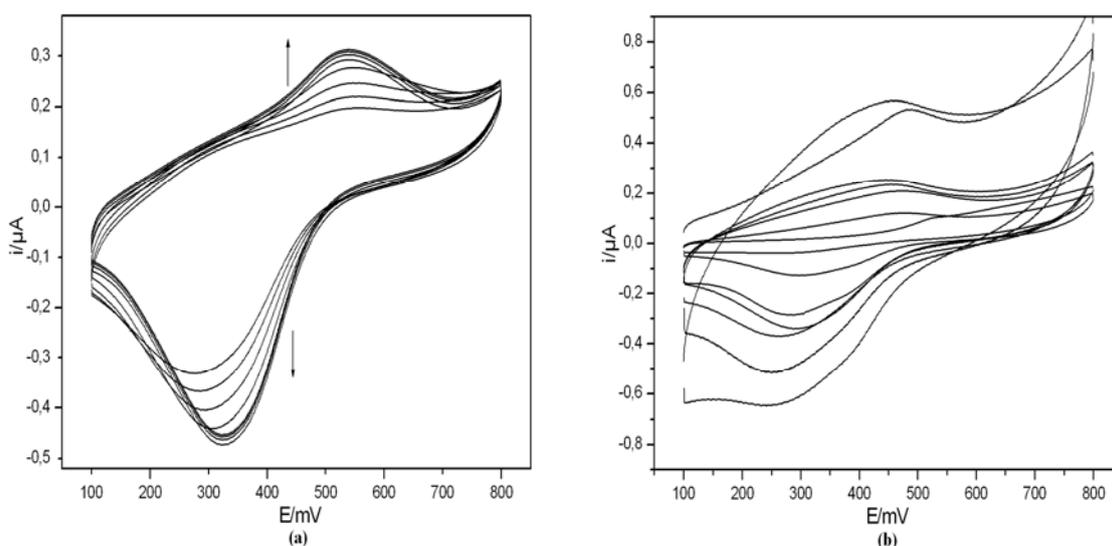
**Fig. 2.** Cyclic Voltammogram of poly(GMA-co-VFc) in 0.1 M PBS (pH 7.5) (a) at scan rate 5 mV/s (b) at scan rate of 1, 2.5, 5, 7.5, 10, 15 and 20 mV/s (from internal to external)
