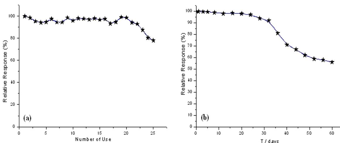
**Fig. 7.** (a) Reusability of the Cat immobilized electrode. Each data point represents the average of data collected by three electrodes (pH 7.5; ~25°C). (b) Storage stability of Cat immobilized electrode. The amperometric responses of these enzyme electrodes are regularly checked during 50 days (pH 7.5; ~25°C).
