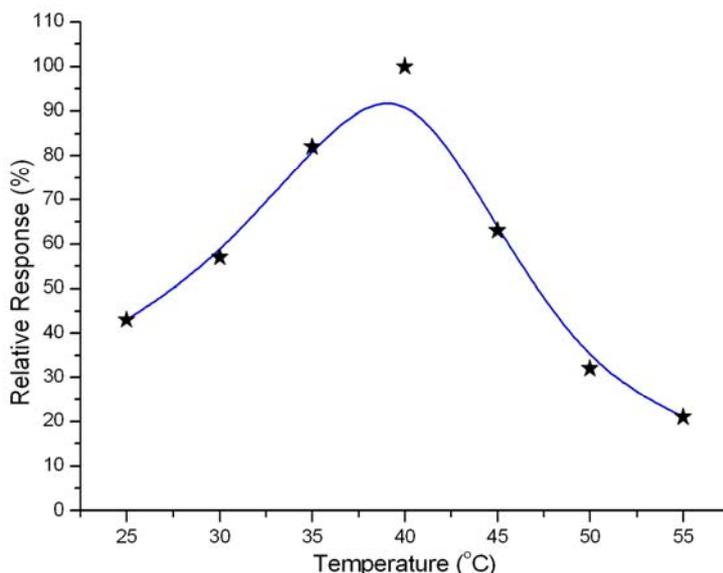
**Fig. 6.** The effect of temperature on the response of the Cat immobilized electrodes in the presence of 10 mM H<sub>2</sub>O<sub>2</sub> in PBS solution. Data collected with freshly prepared enzyme electrodes refer to the average of three experiments
