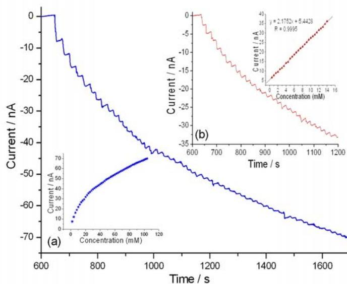
**Fig. 4.** Amperometric response of the enzyme electrode at an applied potential +0.35 V pH 7.5 10 mM PBS, (a) successive addition of 2 mM and (b) 0.5 mM: inset plot of amperometric current vs. H<sub>2</sub>O<sub>2</sub> concentration and linear calibration curve for determination of  $K_m$
