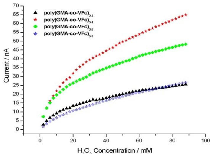
**Fig. 3.** Comparison of amperometric responses of the enzyme electrode at an applied potential +0.35 V fabricated with (a) GMA-co-VFc0.2, (b) GMA-co-VFc0.4, (c) GMA-co-VFc0.6, (d) GMA-co-VFc0.8 to successive addition of H<sub>2</sub>O<sub>2</sub> at constant potential pH 7.5 10 mM PBS
