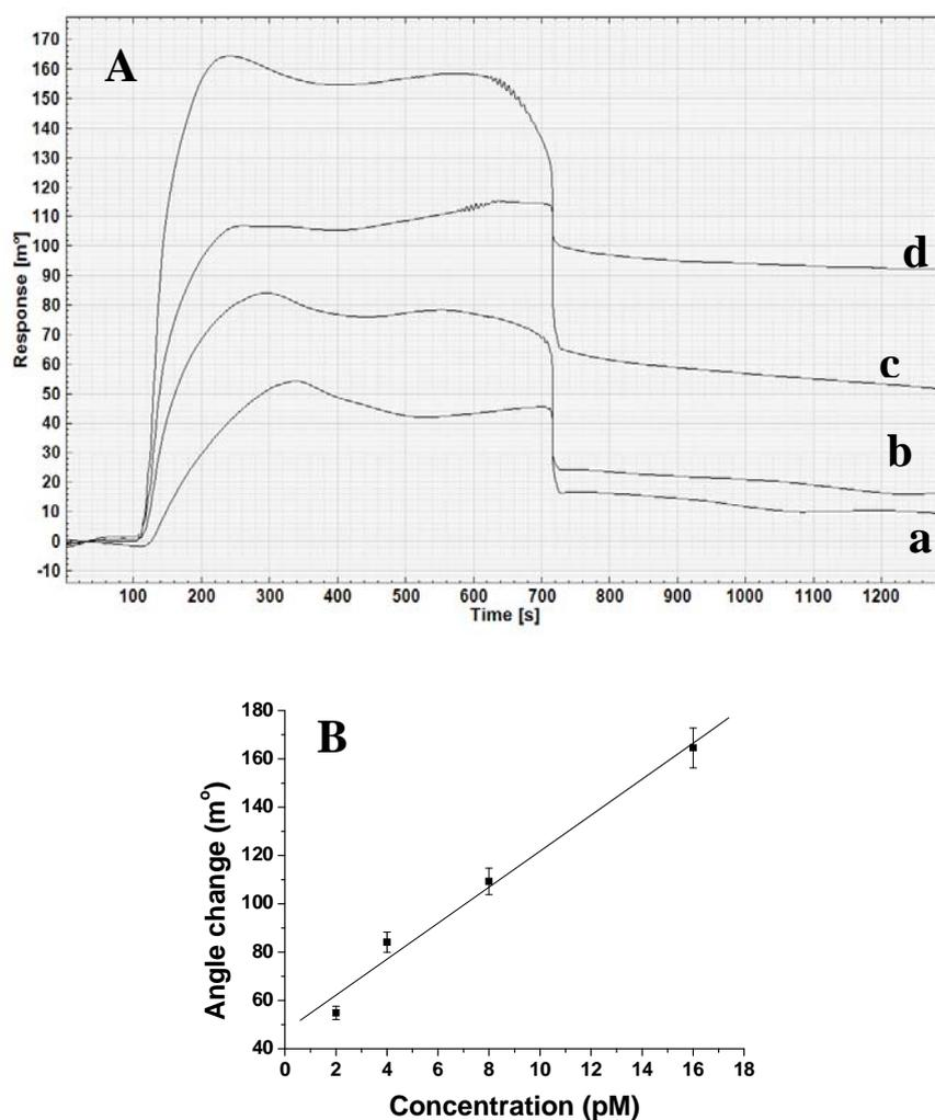
**Fig. 2.** (A) SPR sensor response for the interaction of different concentration of *B. abortus* CSP-31 antigen with immobilized antibody (a) 2.0 pM, (b) 4.0 pM, (c) 8.0 pM and (d) 16.0 pM and (B) Calibration plot for the interaction of *B. abortus* CSP-31 antigen with immobilized antibody
