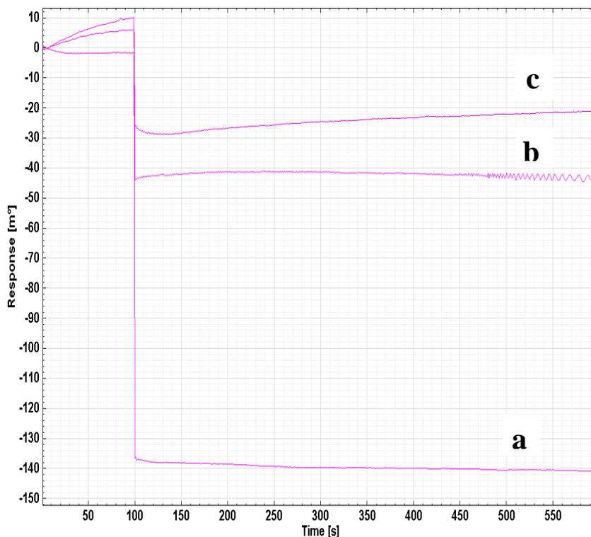
**Fig. 5.** SPR sensor response for the interference of different concentration (a) 3.0 nM, (b) 30.0 nM and (c) 300.0 nM of *B. abortus* CE antigen with immobilized *B. abortus* CSP-31 antibody
