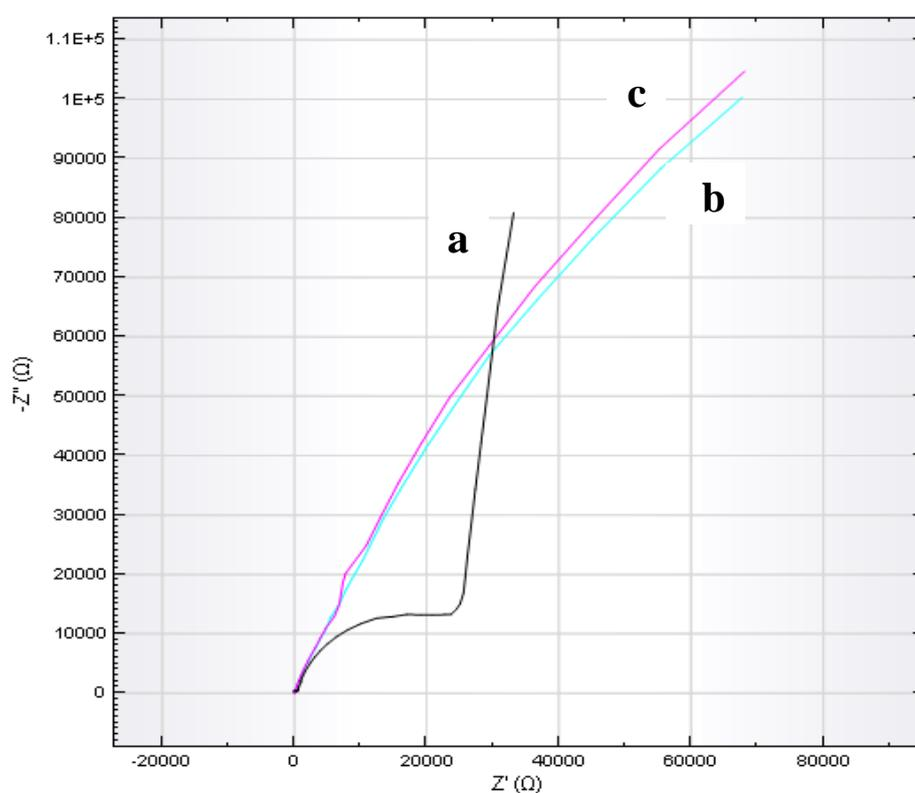
**Fig. 4.** Electrochemical impedance spectrum (EIS) for (a) carboxymethyl dextran modified gold disc (b) modified gold disc immobilized with *B. abortus* CSP-31 and (c) *B. abortus* CSP-31 antigen interaction with immobilized antibody. pH 7.5, temperature: 25°C and concentration: 16.0 pM
