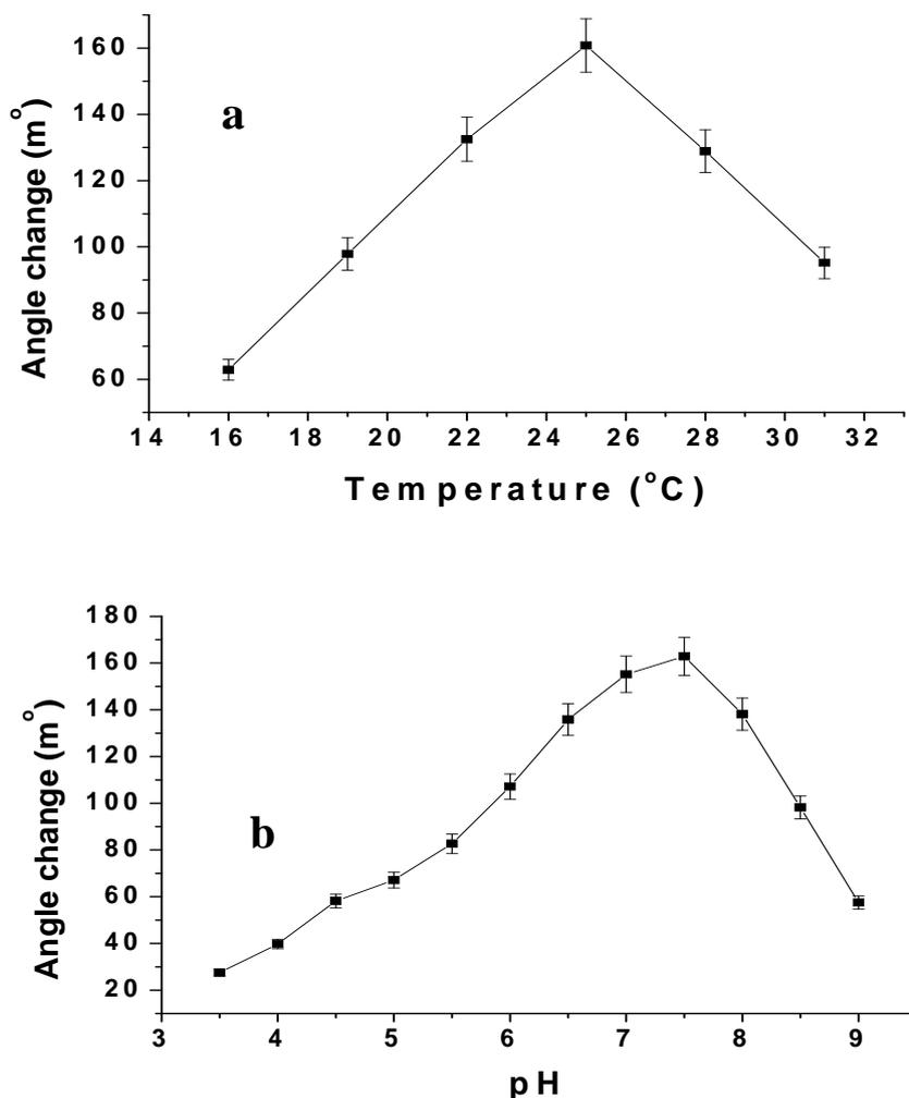
**Fig.3.** (a) Effect of temperature for the interaction of *B. abortus* CSP-31 antigen with the immobilized *B. abortus* CSP-31 antibody. Temperature range: 16 °C-31 °C, pH: 7.5 and concentration: 16.0 pM and (b) Effect of pH for the interaction of *B. abortus* CSP-31 antigen with immobilized *B. abortus* CSP-31 antibody. pH range: 3.5-9.0, temperature: 25°C and concentration: 16.0 pM
