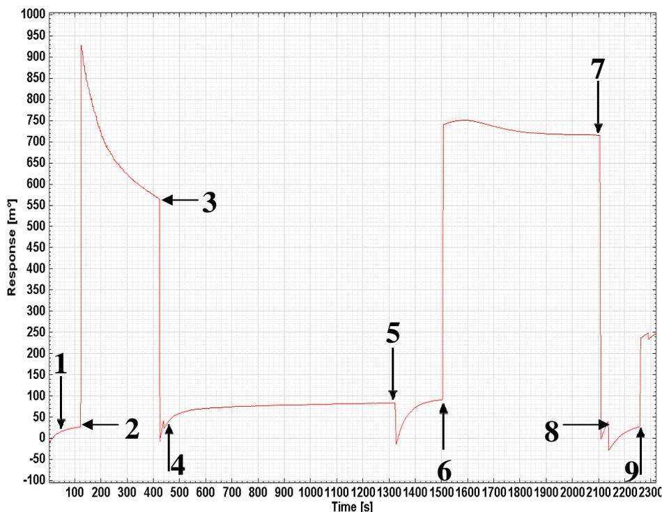
**Fig. 1.** Sensorgram showing different steps [(1) Baseline (2) EDC-NHS activation (3) Washing (4) Antibody coupling (5) Washing (6) Deactivation (7) Washing (8) Regeneration and (9) Back to baseline] involved in the immobilization of *B. abortus* CSP-31 antibody (1: 1000 dilution) on carboxymethyl dextran modified gold disc
