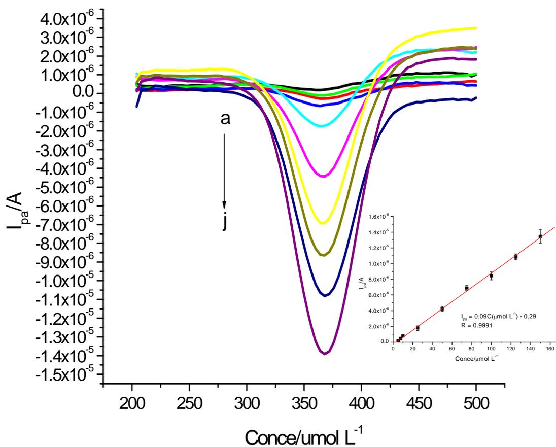
**Fig. 6.** Differential pulse voltammograms of solution containing (aj) 2.5, 5.0, 7.5, 10, 25, 50, 75, 100, 125 and 150  $\mu\text{mol L}^{-1}$  standard paracetamol. The inset shows the calibration curve for various concentrations of paracetamol. (Background subtracted)
