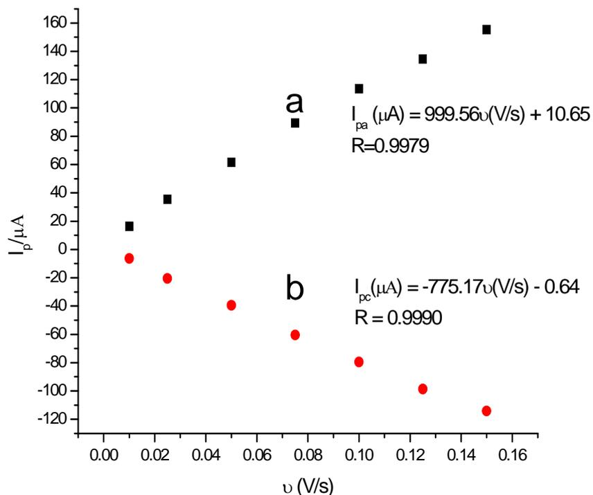
**Fig. 3.** Plot of peak current versus scan rate for the electrochemical oxidation of paracetamol at the PEDOT modified GC electrode: (a) anodic current peak and (b) cathodic current peak
