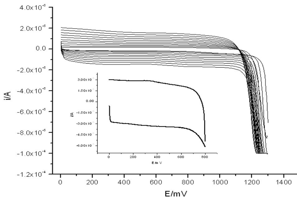
**Fig. 1.** Formation of PEDOT film onto GC electrode. The inset is the cyclic voltammetry of the PEDOT modified electrode in phosphate buffer solution
