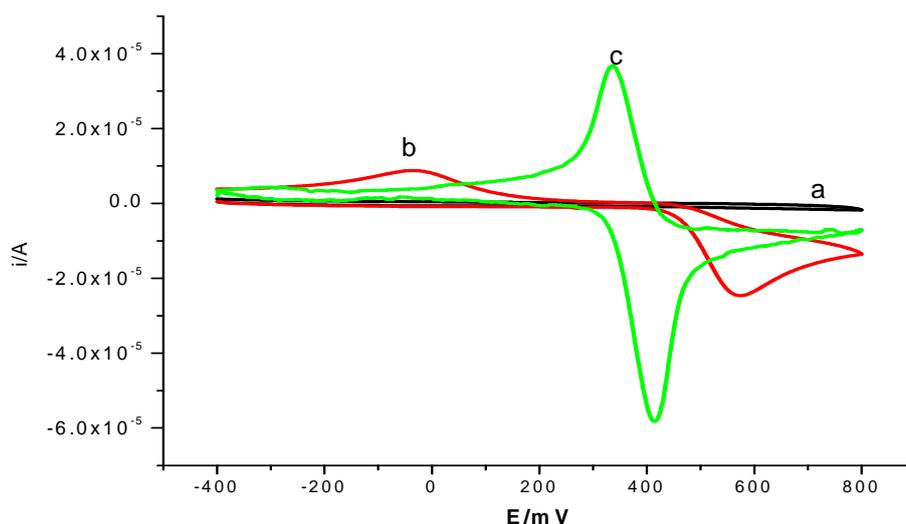
**Fig. 2.** Cyclic voltammogram (CV) at scan rate of  $0.1 \text{ Vs}^{-1}$  obtained at: (a) GC electrode for  $0.1 \text{ mol L}^{-1}$  phosphate buffer supporting electrolyte, (b) bare GC with  $1 \text{ mmol L}^{-1}$  paracetamol in phosphate buffer and (c) PEDOT modified GC electrode with  $1 \text{ mmol L}^{-1}$  paracetamol in phosphate buffer (Background subtracted)
