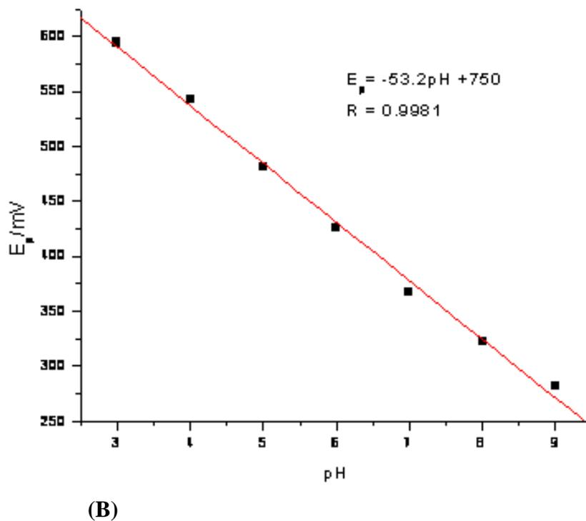
**Fig. 4.** The relation between (A) peak current  $I_p$  and pH, and (B) peak potential  $E_p$  and pH. Scan rate 0.1 V s<sup>-1</sup>
