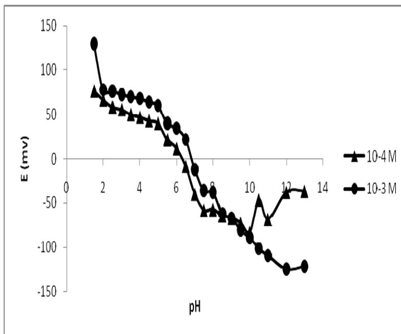
Fig. 4. Effect of pH on the response of sensor 3
