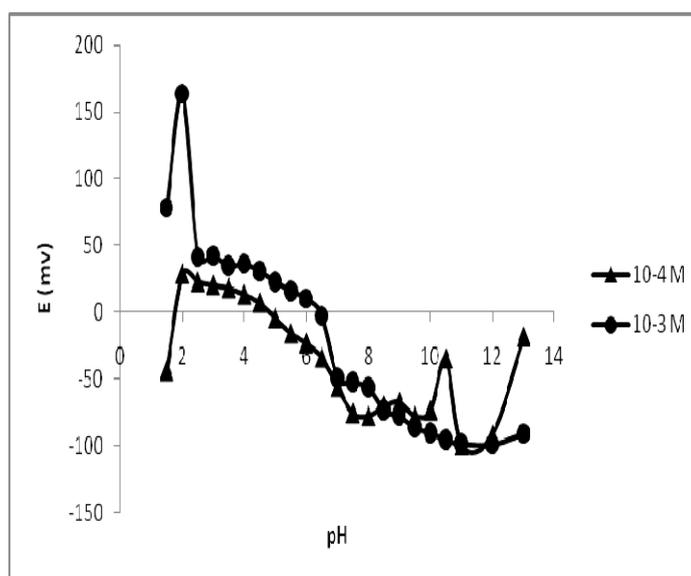
**Fig. 3.** Effect of pH on the response of sensor 2
