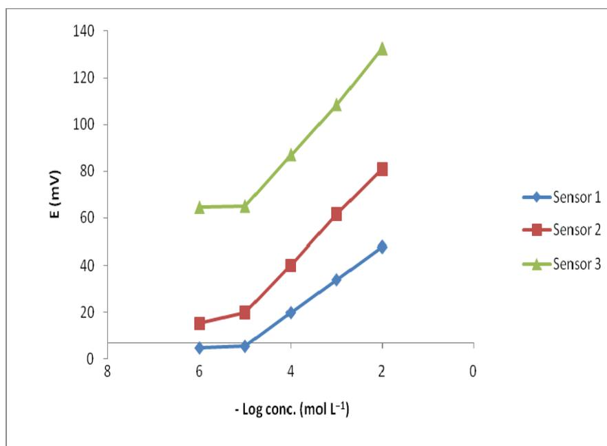
**Fig. 5.** Profile of the potential in mV vs.  $-\log$  concentrations of GM in  $\text{mol L}^{-1}$  obtained with sensors 1, 2 and 3
