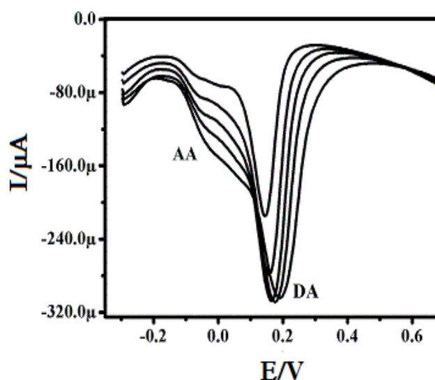
**Fig. 7.** Differential pulse voltammogram for simultaneous detection of AA and DA in 0.1 M phosphate buffer solution of pH 7.0 at ZVNISDSMCPE with the scan rate of  $50 \text{ mV s}^{-1}$
