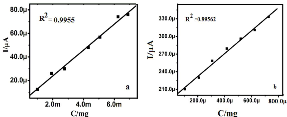
**Fig. 8.** (a) Differential pulse voltammogram for simultaneous detection of DA and AA with different concentrations in presence of 0.1 M PBS at pH7.0 with a scan rate of  $50 \text{ mVs}^{-1}$  of DA concentration from 1.04 mM to 7.27 mM; (b) graph of peak current Vs AA concentration from 1 mM to 6.85 mM in pH7.0 with the scan rate of  $50 \text{ mVs}^{-1}$
