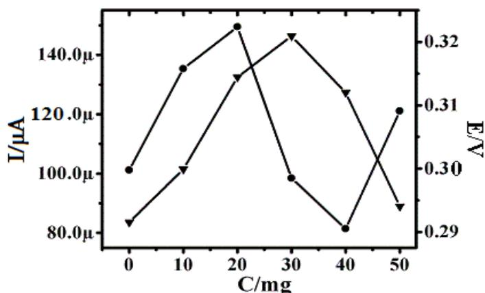
**Fig. 2.** Relationship between anodic peak current ( $I_{pa}$ ) vs. Concentration of ZVNI and anodic peak potential ( $E_{pa}$ ) in 1 mM AA with carbon paste electrode
