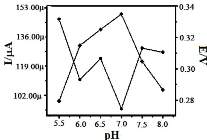
**Fig. 5.** Effect of pH on the peak current (A) and peak potentials for the oxidation of 0.1 mM AA with a scan rate of  $50 \text{ mVs}^{-1}$  in presence of 0.1 M PBS
