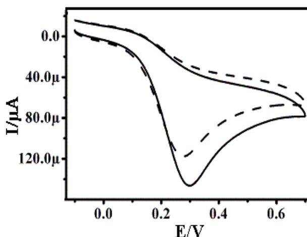
**Fig. 3.** Cyclic voltammograms of AA at the bare carbon paste electrode and ZVNI in presence of 0.1 M PBS
