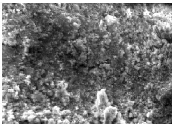
**Fig. 1.** SEM image of synthesized ZVNI particles
