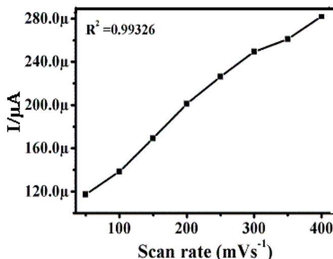
**Fig. 4.** Anodic peak current vs. square root of scan rate for 1 mM AA at ZVNI in presence of 0.1 M PBS at pH-7.0
