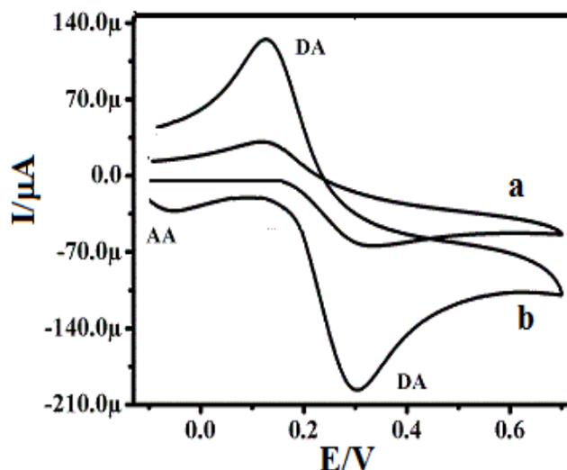
**Fig. 6.** Cyclic voltammograms for simultaneous determination of AA in presence of DA with 0.1 M phosphate buffer solution of pH 7.0 at (a) ZVNI MCPE and (b) ZVNISDSMCPE with the scan rate of  $50 \text{ mVs}^{-1}$
