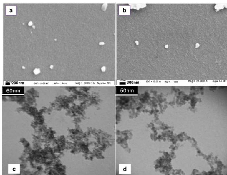
**Fig. 10.** SEM (a and b) and TEM (c and d) images of the prepared Ni(OH)<sub>2</sub> and NiO nanoparticles, respectively
