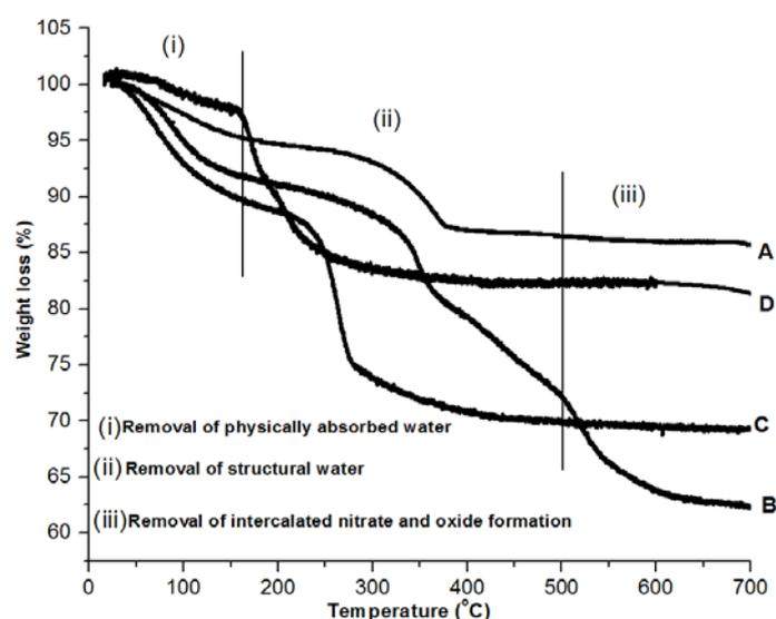
**Fig. 6.** TG analysis of the prepared (A) La(OH)<sub>3</sub>, (B) Gd(OH)<sub>3</sub>, (C) Ni(OH)<sub>2</sub> and (D) Co(OH)<sub>2</sub> nanoparticles
