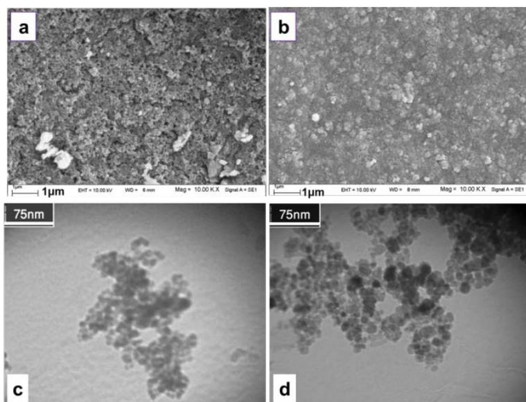
**Fig. 8.** SEM (a and b) and TEM (c and d) images of the prepared  $\text{La}(\text{OH})_3$  and  $\text{La}_2\text{O}_3$  nanoparticles, respectively
