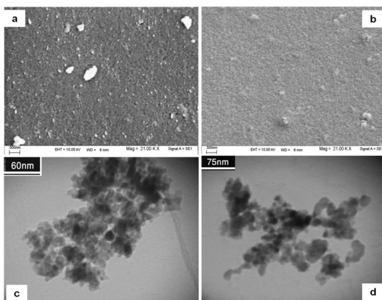
**Fig. 11.** SEM (a and b) and TEM (c and d) images of the prepared Co(OH)<sub>2</sub> and Co<sub>3</sub>O<sub>4</sub> nanoparticles, respectively
