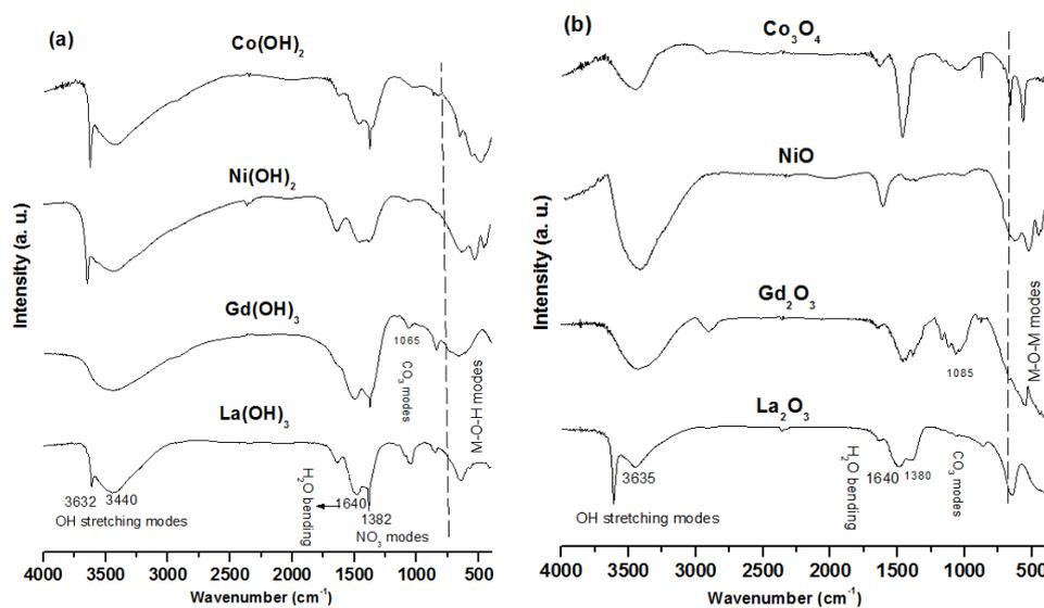
**Fig. 7.** IR spectra of the prepared (a) hydroxides and (b) oxides nanoparticles
