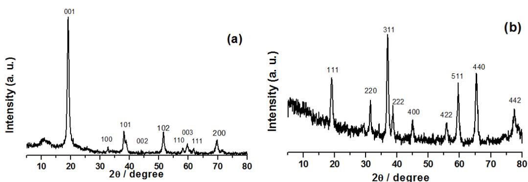
**Fig. 4.** XRD patterns of the prepared (a) Co(OH)<sub>2</sub> and (b) Co<sub>3</sub>O<sub>4</sub> nanoparticles
