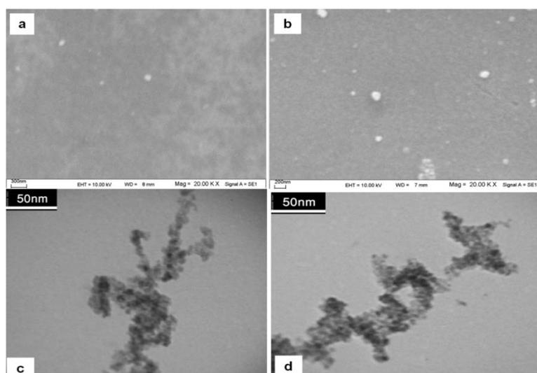
**Fig. 9.** SEM (a and b) and TEM (c and d) images of the prepared  $\text{Gd}(\text{OH})_3$  and  $\text{Gd}_2\text{O}_3$  nanoparticles, respectively
