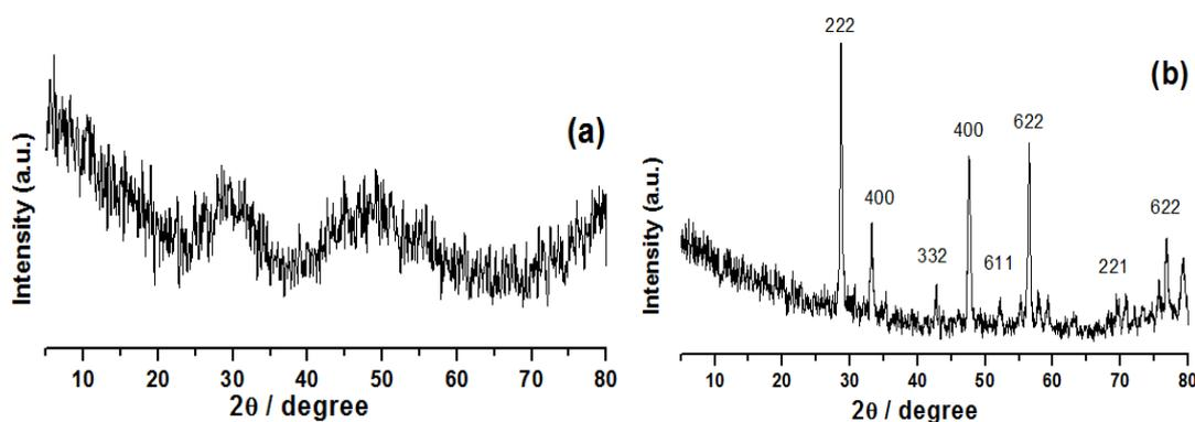
**Fig. 5.** XRD patterns of the prepared (a)  $\text{Gd}(\text{OH})_3$  and (b)  $\text{Gd}_2\text{O}_3$  nanoparticles
