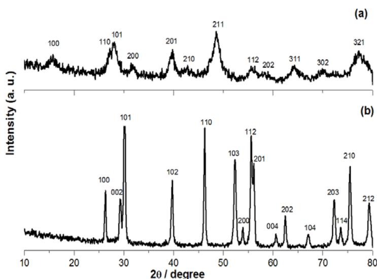
**Fig. 2.** XRD patterns of the prepared (a)  $\text{La}(\text{OH})_3$  and (b)  $\text{La}_2\text{O}_3$  nanoparticles
