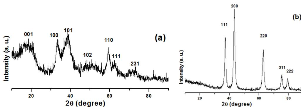
**Fig. 3.** XRD patterns of the prepared (a) Ni(OH)<sub>2</sub> and (b) NiO nanoparticles
