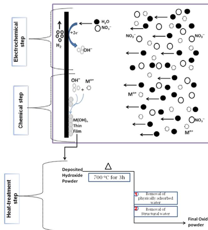
**Fig. 1.** A schematic view of hydroxide and oxide formation via cathodic electrodeposition-heat treatment
