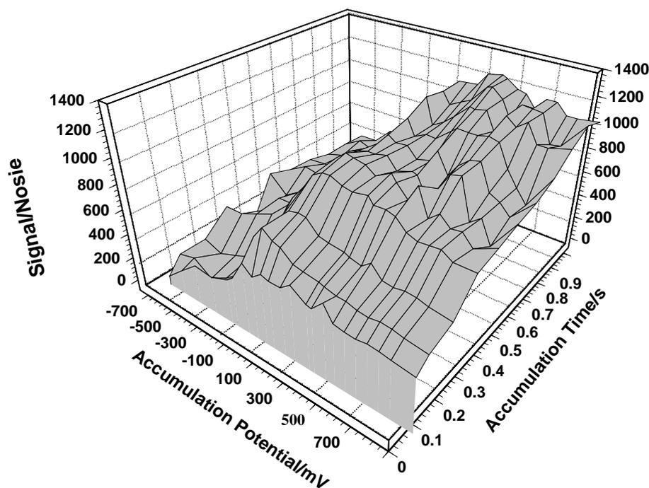
**Fig. 7.** Effect of accumulation potential and Effect of accumulation time on the electrode response to injections of  $1.0 \times 10^{-10}$  M folic acid in 0.05 M  $\text{H}_3\text{PO}_4$
