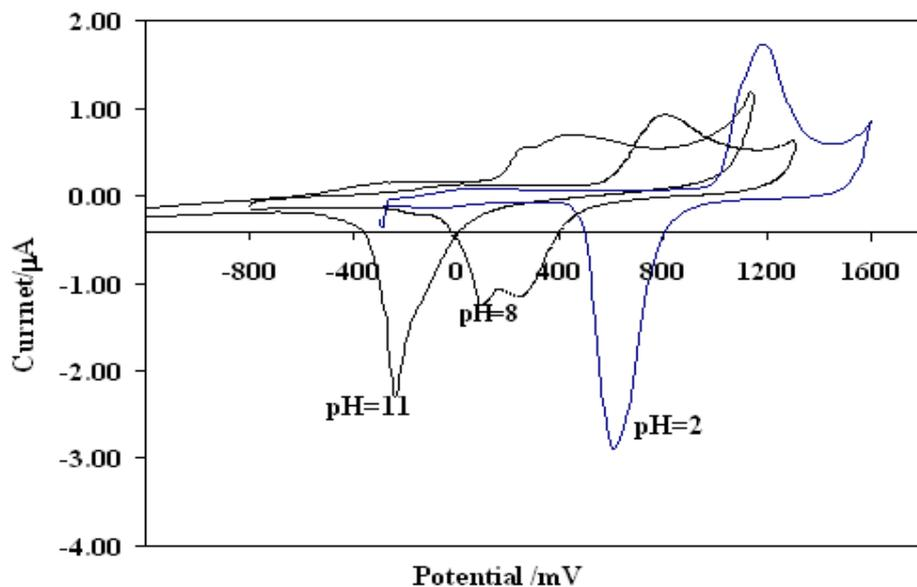
**Fig. 5.** Effect of pH on the response of electrode. The eluent was 0.05 M  $\text{H}_3\text{PO}_4$  and the flow rate was  $3 \text{ mL min}^{-1}$  and sweep rate  $70 \text{ Vs}^{-1}$  in  $1.0 \times 10^{-7} \text{ M}$  of Folic acid
