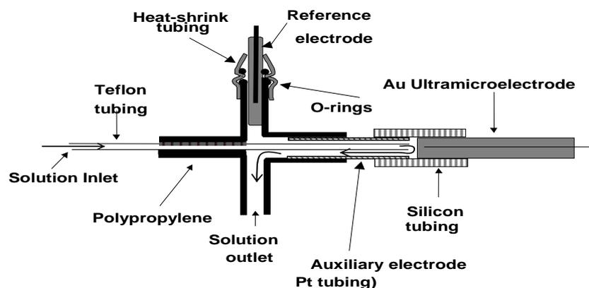
**Fig. 1.** Diagram of the electrochemical cell
