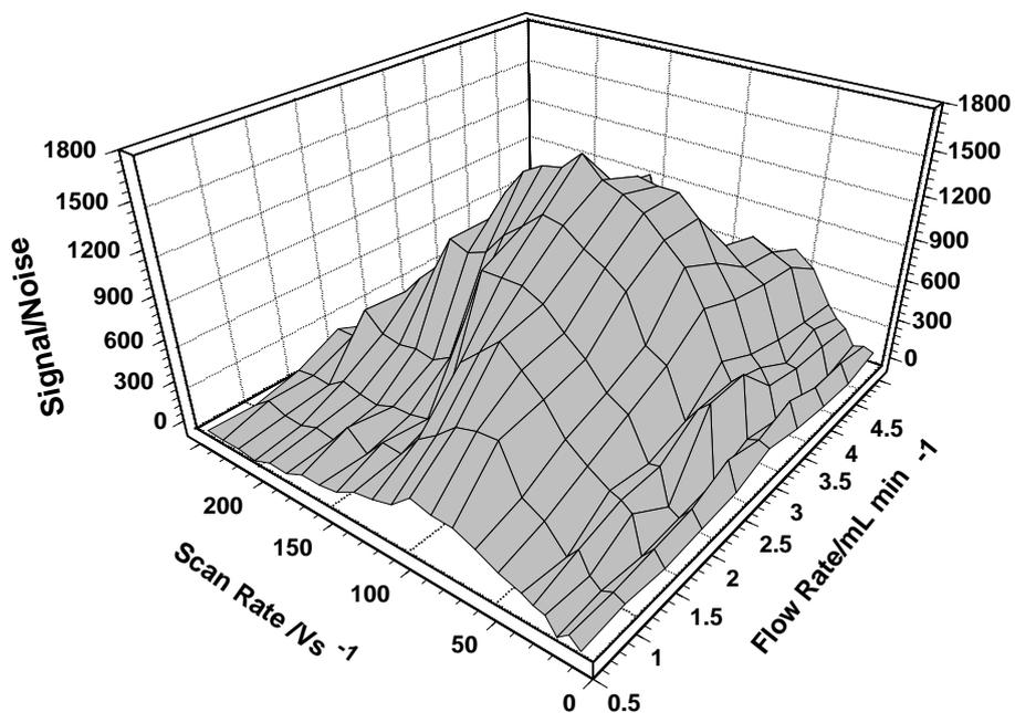
**Fig. 6.** Effect of the sweep rate on the response of the Au microelectrode to injections of  $1.0 \times 10^{-10} \text{ M}$  folic acid in 0.05 M  $\text{H}_3\text{PO}_4$
