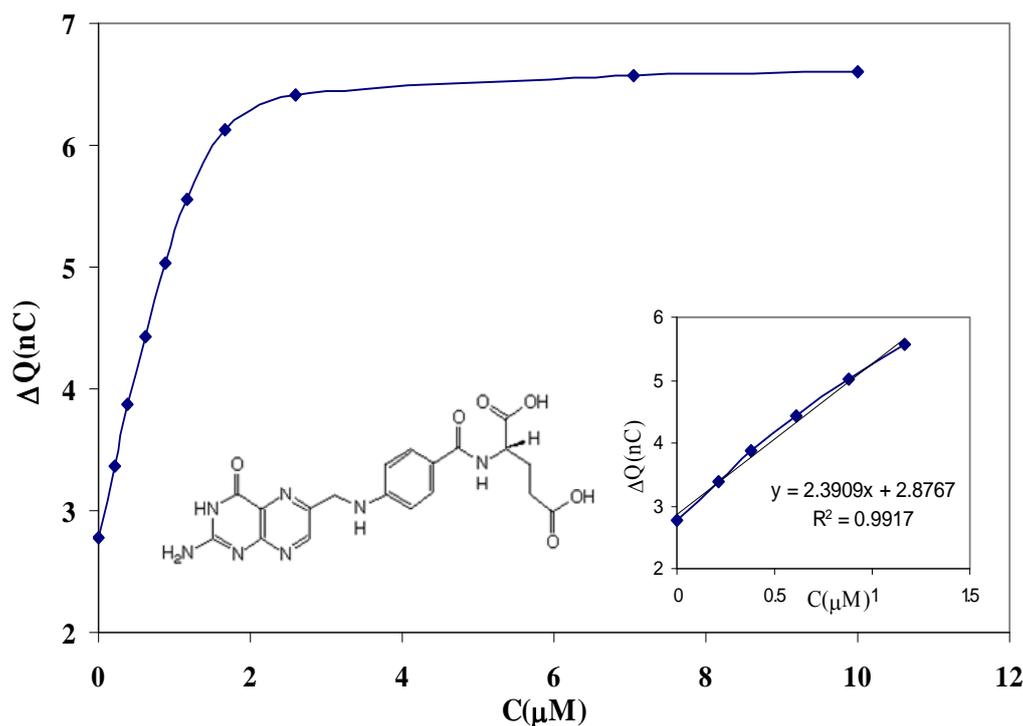
**Fig. 8.** Calibration curves obtained for folic acid on the Au microelectrode in 0.05 M  $\text{H}_3\text{PO}_4$
