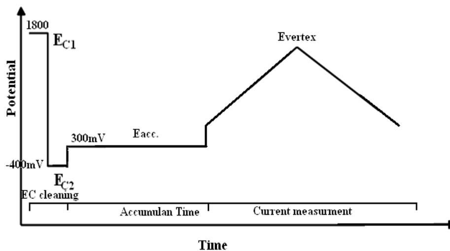
**Fig. 2.** Diagram of the applied potential waveform
