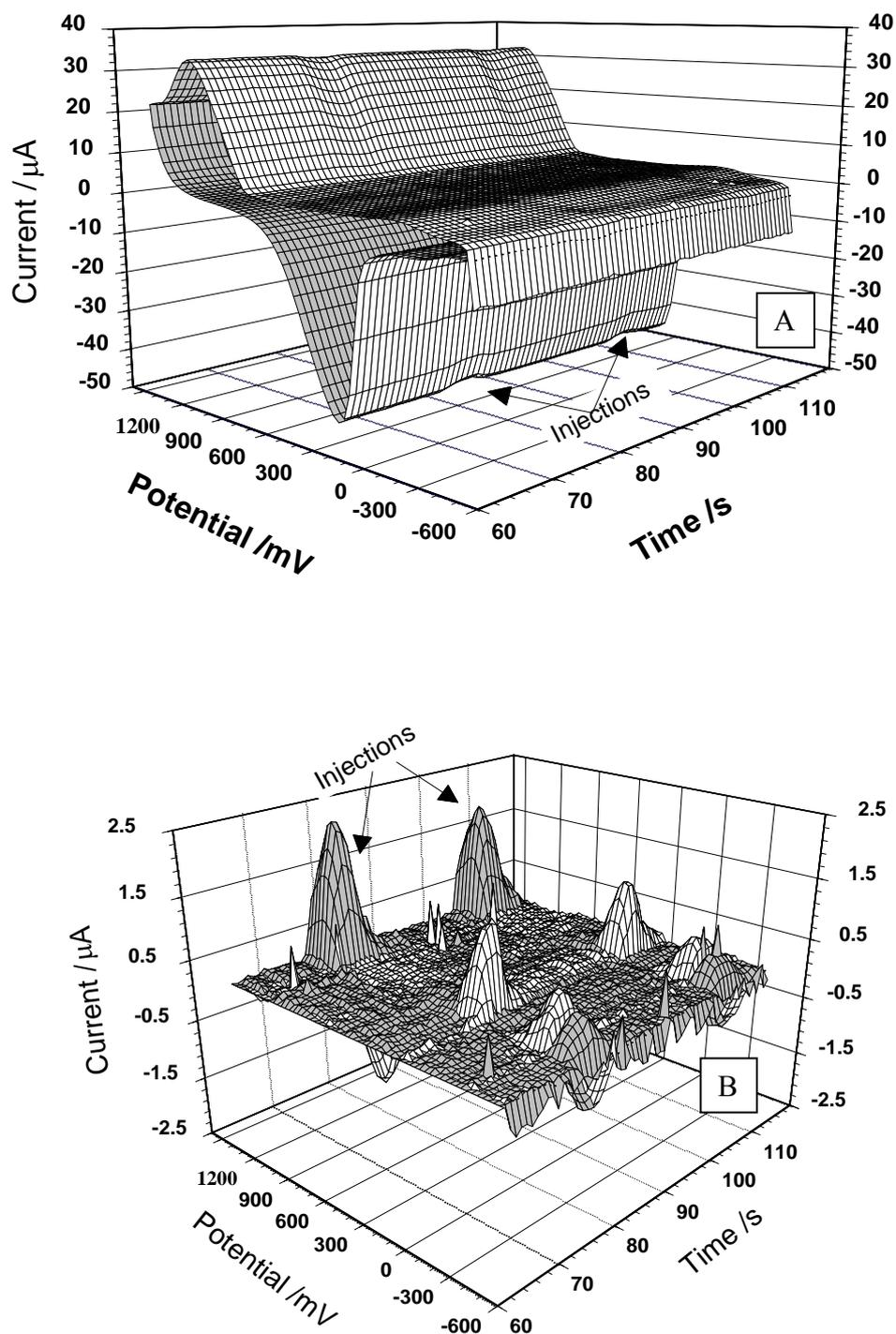
**Fig. 4(a).** Cyclic voltammograms at Au microelectrode recorded during the flow injection of  $50 \mu\text{L}$  of  $1.0 \times 10^{-6} \text{ M}$  of folic acid at optimum conditions. The eluent was  $0.05 \text{ M H}_3\text{PO}_4$  and the flow rate was  $3 \text{ mL min}^{-1}$  b). Curves result from subtracting an average CV (in the absence of analyte) from test of the CVs in (a)
