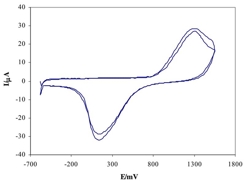
**Fig. 3.** The CV gram of electrode in the eluent 0.05 M  $\text{H}_3\text{PO}_4$  (pH=2) and the flow rate was  $3 \text{ mL min}^{-1}$ , sweep rate was  $70 \text{ Vs}^{-1}$  (a) in the absence and (b) in the presence of analyte ( $1.0 \times 10^{-6} \text{ M}$ )
