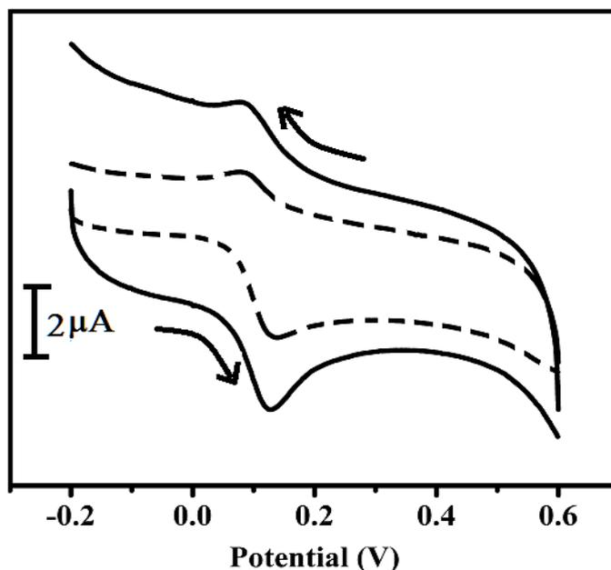
**Fig. 5.** Cyclic voltammogram of  $1 \times 10^{-5}$  M DA in PBS at pH 7.0 at dashed line for bare CPE and solid line for ZnO nanoparticles MCPE
