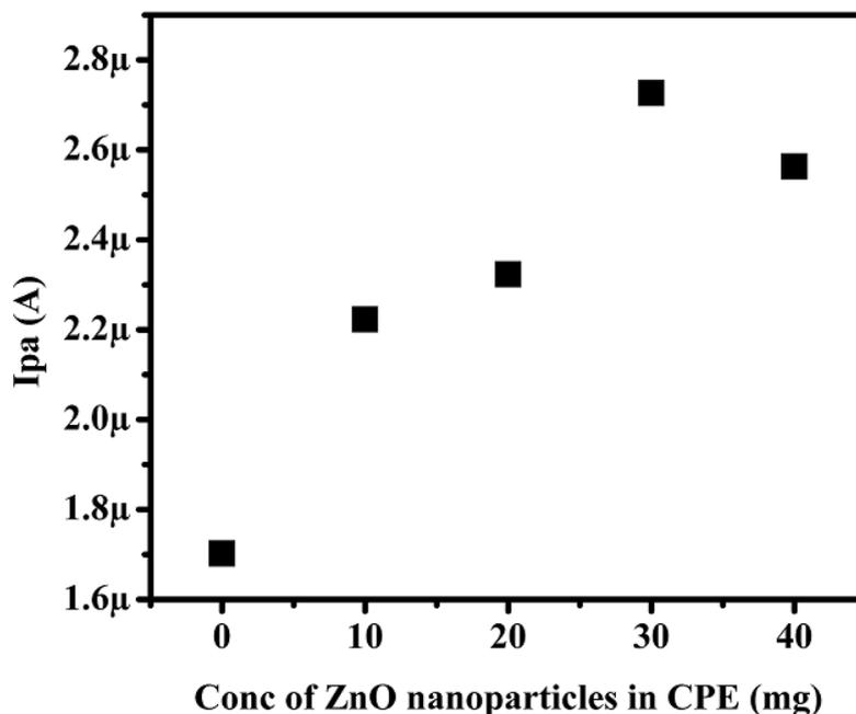
**Fig. 4.** Shows the graph between anodic peak current ( $I_{pa}$ ) vs. different concentration of ZnO nanoparticles in CPE
