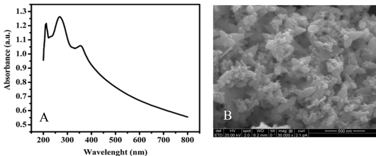
Fig. 3. A) UV-Vis absorption spectra and B) SEM image for ZnO nanoparticles
