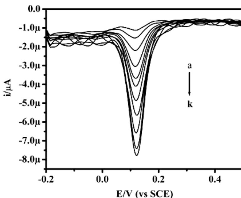
**Fig. 8.** Differential pulse voltammogram of (a)  $1.0 \times 10^{-7}$  M, (b)  $2 \times 10^{-7}$  M, (c)  $4 \times 10^{-7}$  M, (d)  $6 \times 10^{-7}$  M, (e)  $8 \times 10^{-7}$  M, (f)  $10.0 \times 10^{-7}$  M, (g)  $12.0 \times 10^{-7}$  M, (h)  $14.0 \times 10^{-7}$  M, (i)  $16.0 \times 10^{-7}$  M, (j)  $18.0 \times 10^{-7}$  M and (k)  $20.0 \times 10^{-7}$  M DA in 0.2 M phosphate buffer solution of pH 7.0 at ZnO nanoparticles MCPE
