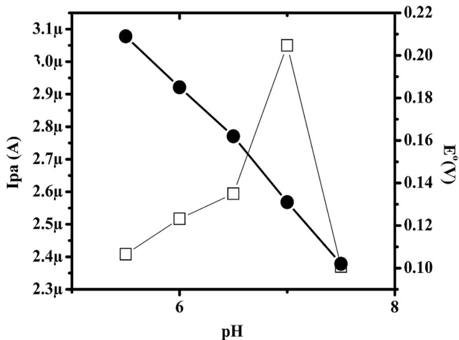
**Fig.6.** Graph shows the dependences of the DA oxidation peak current (-□-) and for formal redox potential (-●-) on the PBS solution pH with a scanning rate of  $100 \text{ mVs}^{-1}$
