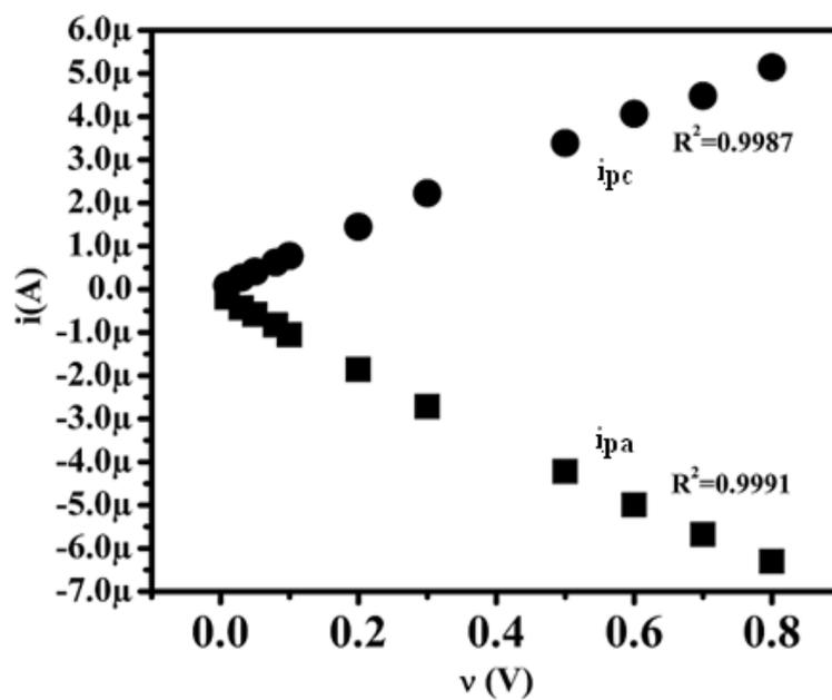
**Fig. 7.** Graph the linear relationship between the peak current vs. the different scan rate (10–800  $\text{mVs}^{-1}$ ) in 0.2 M PBS solutions at pH 7.0
