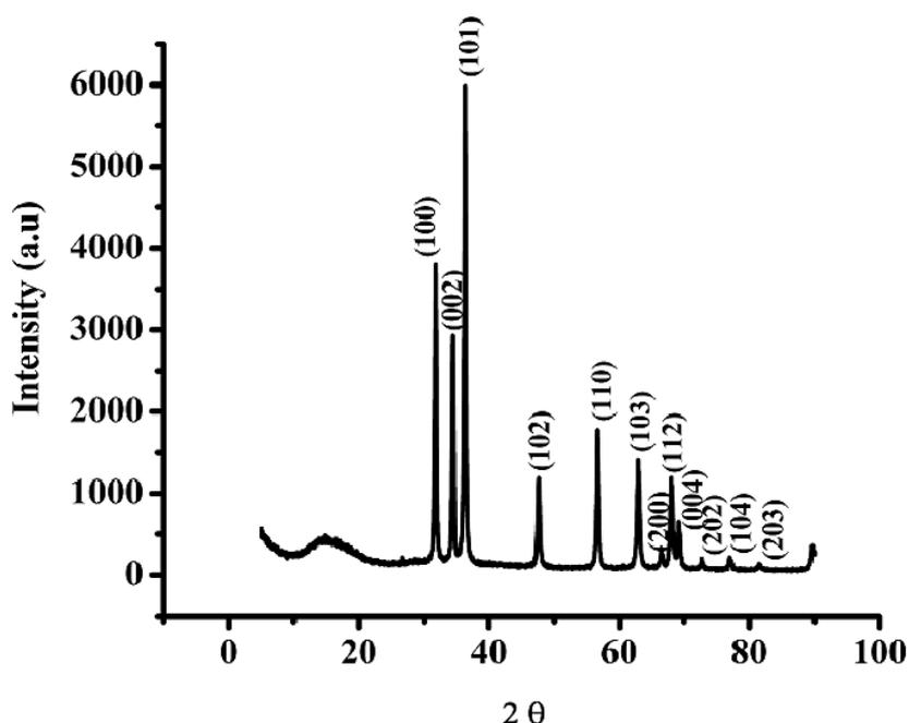
**Fig. 1.** XRD patterns for ZnO nanoparticles
