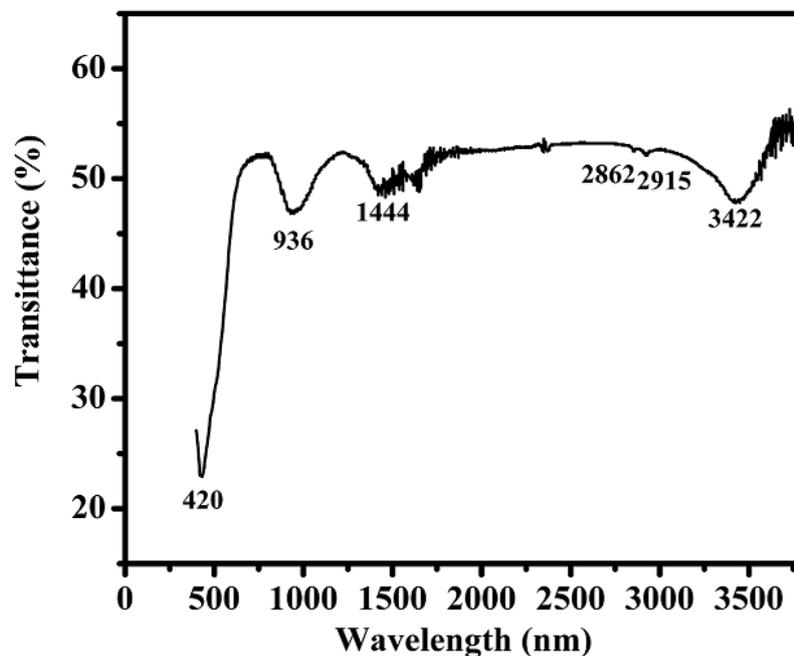
Fig. 2. IR Spectra of ZnO nanoparticles
