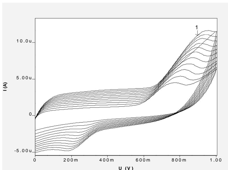
**Fig. 5.** Scan rate ( $v$ ) in BR buffer of pH 8 of  $2.5 \times 10^{-5}$  M Cilostazol solution at GCE
