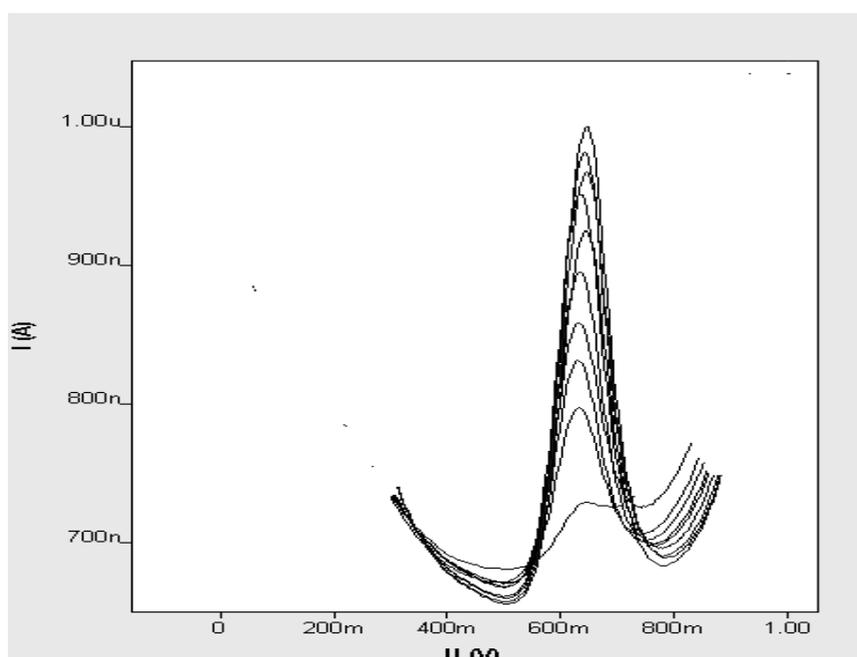
**Fig.11.** Differential pulse voltammograms recorded Cilostazol a( $4.0 \times 10^{-7}$  M), b( $1.15 \times 10^{-6}$  M),c( $1.9 \times 10^{-6}$  M),d( $2.65 \times 10^{-6}$  M),e( $3.4 \times 10^{-6}$  M),f( $4.15 \times 10^{-6}$  M),g( $4.9 \times 10^{-6}$  M),h( $5.65 \times 10^{-6}$  M), and i ( $6.4 \times 10^{-6}$  M) in BR buffer of pH 8 at carbon past electrode
