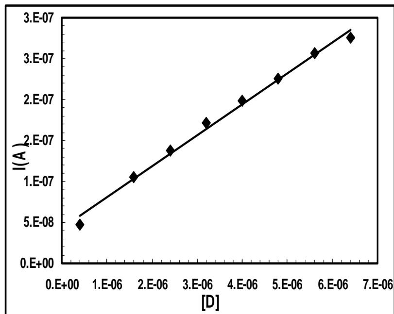
**Fig. 12.** Linear calibration curves of anodic peak currents vs. concentration in the range  $4.0 \times 10^{-7}$ – $6.40 \times 10^{-6}$  M of Cilostazol at carbon past electrode
