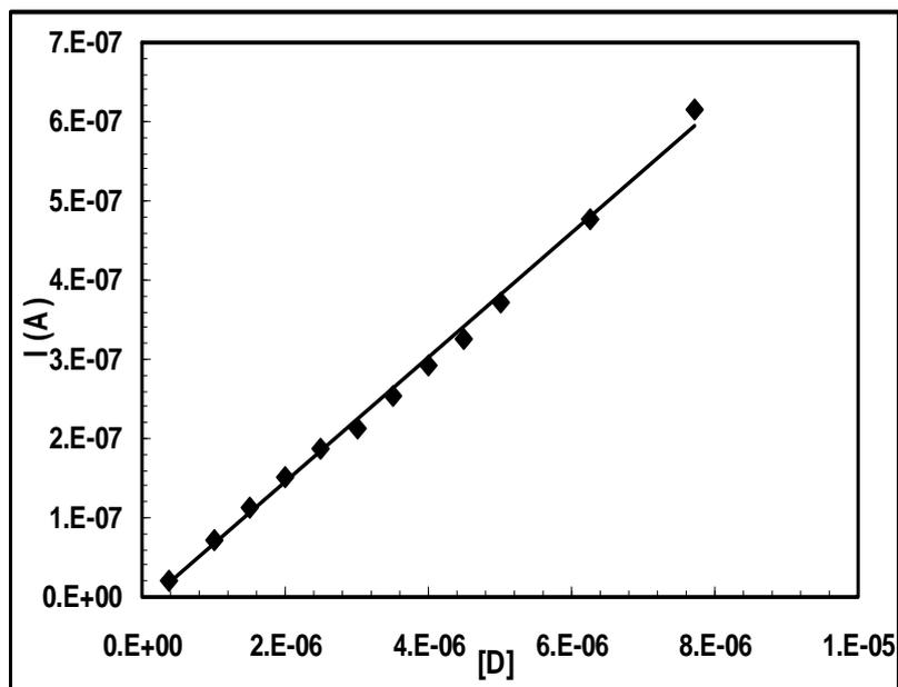
**Fig. 10.** Linear calibration curves of anodic peak currents vs. concentration in the range  $4 \times 10^{-7}$ – $7.7 \times 10^{-6}$  M. of Cilostazol at Glassy carbon electrode
