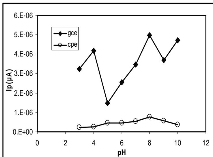
**Fig. 3.** Effect of pH on peak current of  $2.5 \times 10^{-6}$  M Cilostazol solution in BR buffer at CPE paste and GCE at a scan rate 100 mV/s
