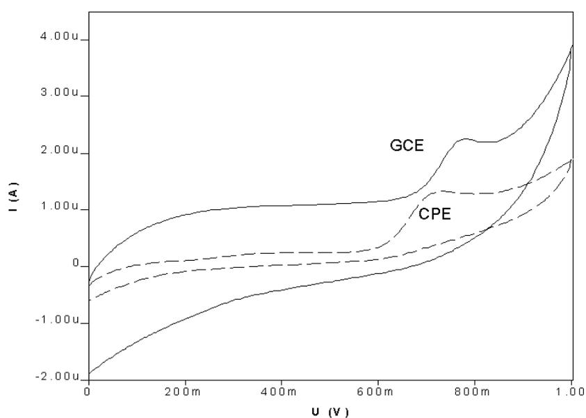
**Fig. 2.** Cyclic voltammograms of  $2.5 \times 10^{-6}$  M Cilostazol solution in BR buffer of pH 8 CPE and GCE at a scan rate 100 mV/s
