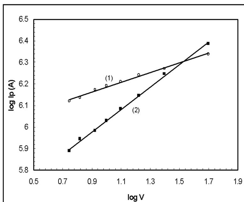
**Fig. 7.** Anodic peak current response of  $2.5 \times 10^{-5}$  M Cilostazole solution as a function of scan rate ( $\nu$ ) in BR buffer of pH 8 at CPE (1) and GCE (2)
