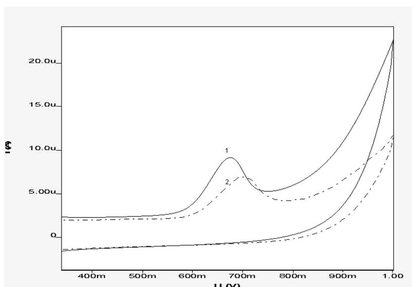
**Fig. 4.** Cyclic voltammograms of  $2.5 \times 10^{-6}$  M Cilostazole solution at GCP in BR buffer (1) and borate buffer (2) at pH 8. Scan rate 100 mV/s
