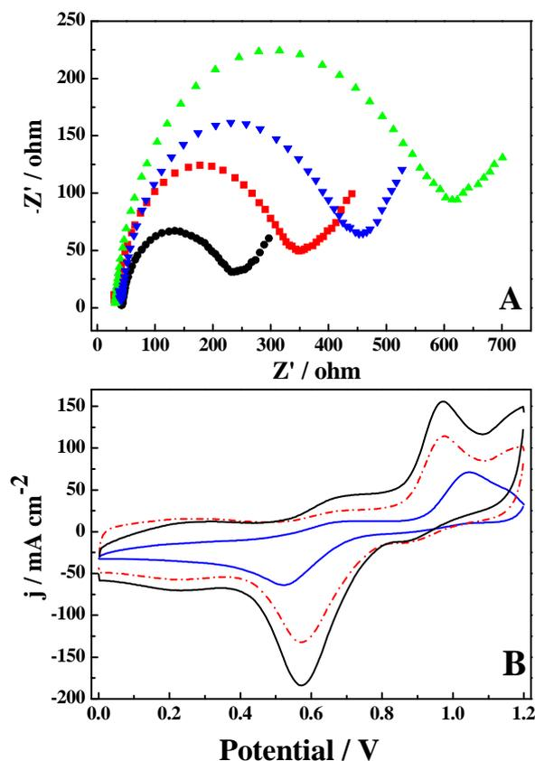
**Fig. 2.** (A) Nyquist plots of bare GCE, graphite/GCE, IL-graphite/GCE, AuNi/IL-graphite/GCE (from outer to inner). Solution composition: 1.0 mM  $K_3Fe(CN)_6$ +1.0 mM  $K_4Fe(CN)_6$ +0.1 M KCl; frequency range: 0.1– $10^5$  Hz. (B) CVs of AuNi/GCE, AuNi/graphite/GCE and AuNi/IL-graphite/GCE (from inner to outer). Supporting electrolyte: 0.5 M  $H_2SO_4$ ; potential scan rate: 100  $mV s^{-1}$
