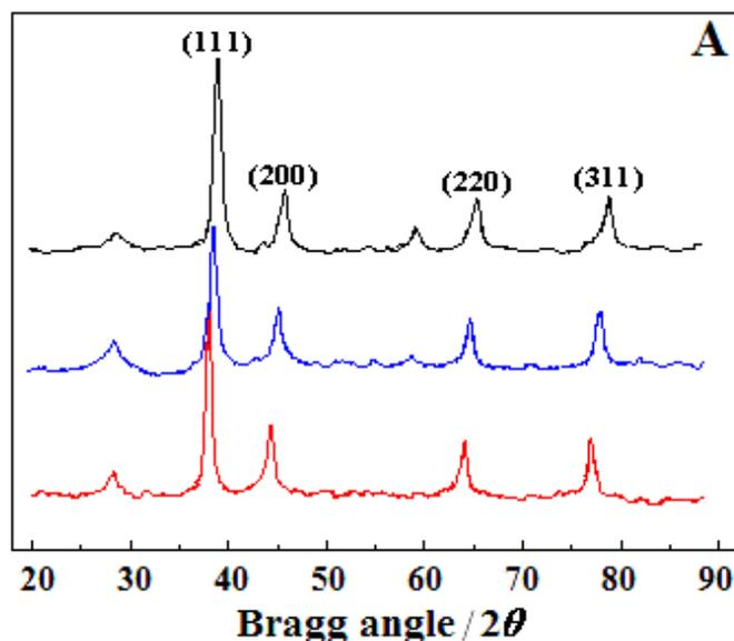
**Fig. 3.** XRD patterns of AuNi, AuCo and Au NPs (from upper to bottom) deposited on IL-graphite film
