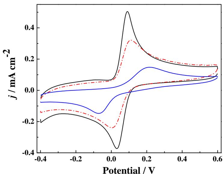
**Fig. 4.** CVs of AuNi/GCE, AuNi–graphite/GCE and AuNi–IL–graphite/GCE (from inner to outer). Solution composition: 0.10 M PBS (pH=7.4)+50  $\mu$ M hydroquinone; potential scan rate: 100 mV s<sup>-1</sup>
