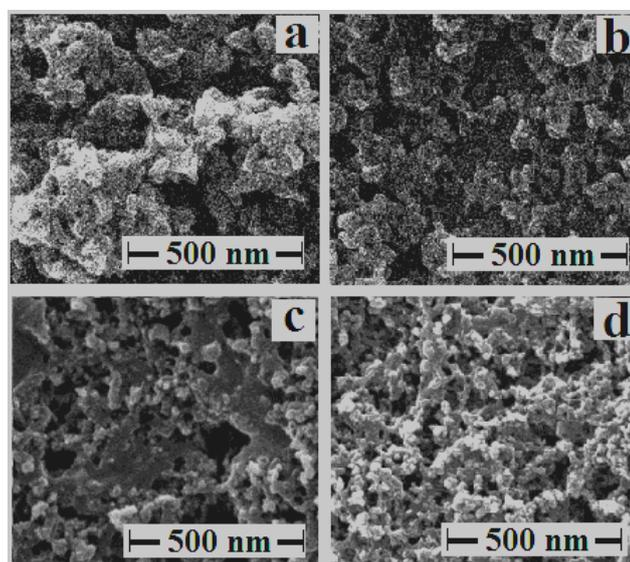
**Fig. 1.** SEM images of purified graphite (a), IL–graphite (b), AuNi–graphite (c) and AuNi IL–graphite (d). Electrodeposition potential: -1.1 V (*vs.* SCE); electrodeposition time: 500 s
