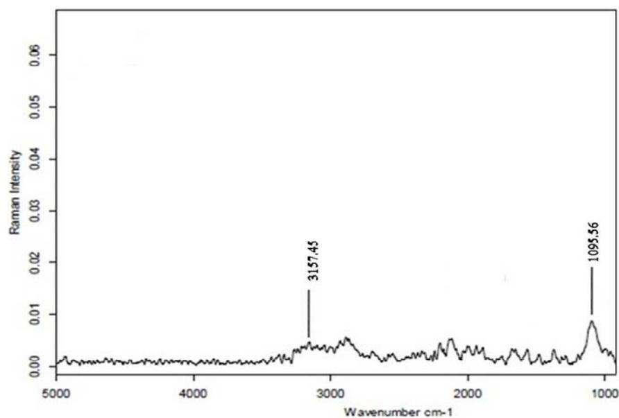
**Fig. 5.** Raman spectroscopy of gold nanoparticles functionalized 8-HQ
