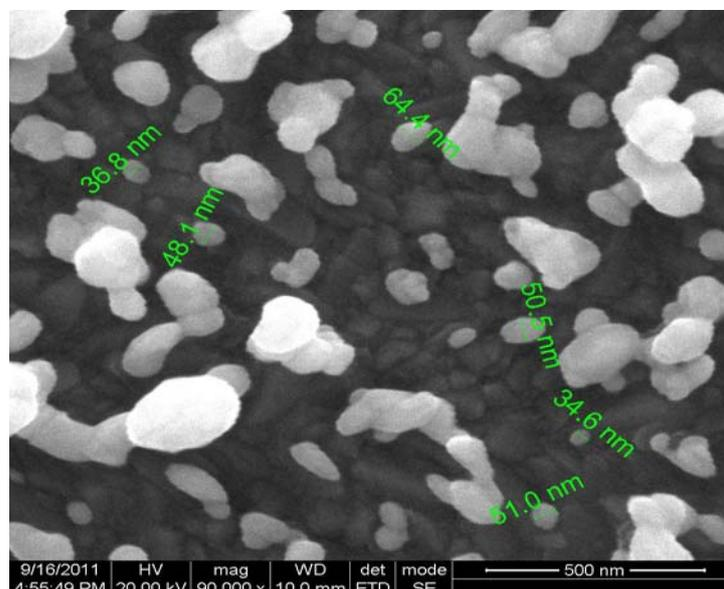
**Fig. 2.** SEM image of gold nanoparticles
