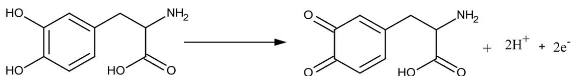
**Scheme 1.** Proposed mechanism for L-dopa on the surface of the electrode
