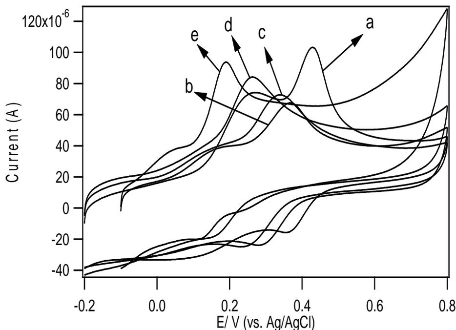
**Fig. 7.** Cyclic voltammograms of 1 mM L-dopa and 1mM AA on the gold nanoparticles functionalized 8-HQ GCE in various pH (a) 3.0, (b) 4.0, (c) 5.0, (c) 6.0, (d) 7.0 various PBS
