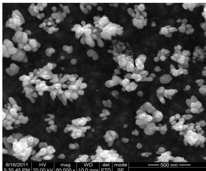
**Fig. 3.** SEM image of gold nanoparticles functionalized 8-HQ
