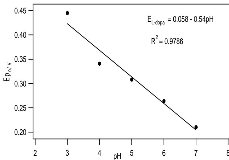
**Fig. 8.** Plot of  $E_{p_0}$  (L-dopa) vs. pH in gold nanoparticles functionalized 8-HQ GCE
