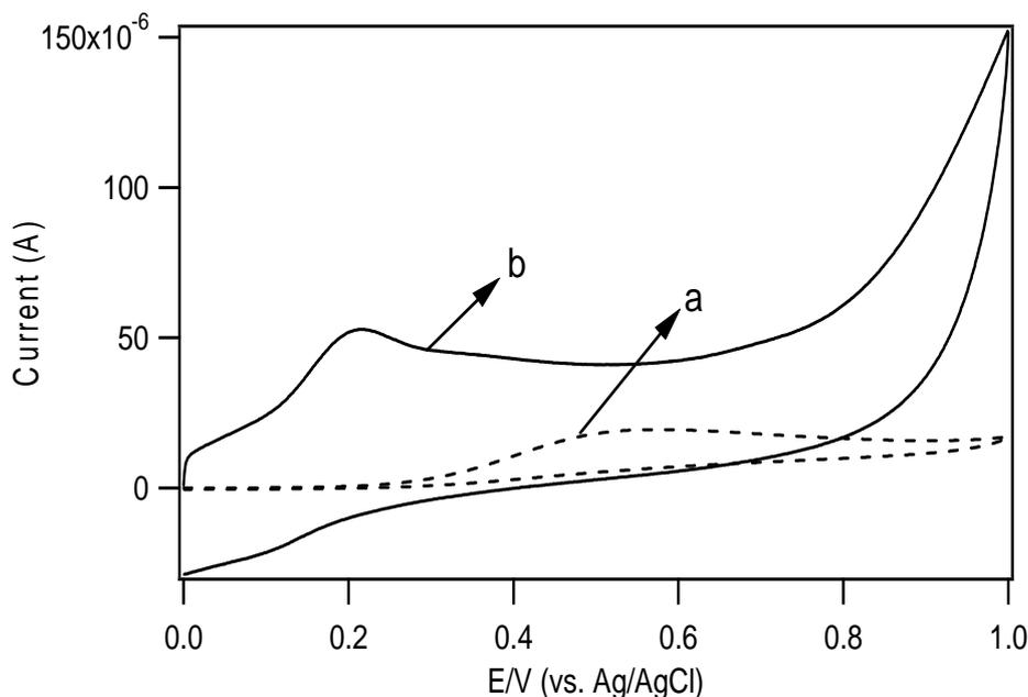
**Fig. 6.** Cyclic voltammogram of 1 mM L-dopa, (a) bare GCE (b) gold nanoparticles functionalized 8-HQ GCE
