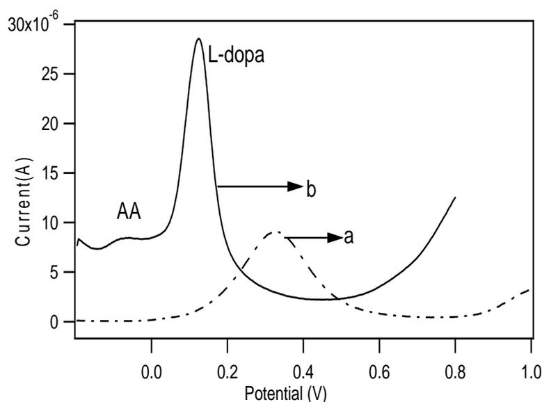
**Fig. 9.** DPV of 1 mM L-dopa and 1 mM AA, (a) bare, (b) gold nanoparticles functionalized 8-HQ
