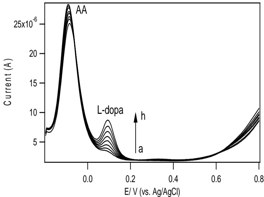
**Fig. 10.** Dpv of 1 mM AA at gold nanoparticles functionalized 8-HQ GCE in the presence of different concentration of L-dopa: (a) 3.0, (b) 4.0, (c) 5.0 (d) 6.0 (e) 7.0 (f) 8.0 (g) 9.0 (h) 10.0  $\mu\text{M}$
