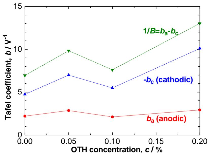
**Fig. 8.** Dependence of Tafel constants with respect of OTH concentration determined from cathodic ( $-b_c$ ) and anodic ( $b_a$ ) potential scan
