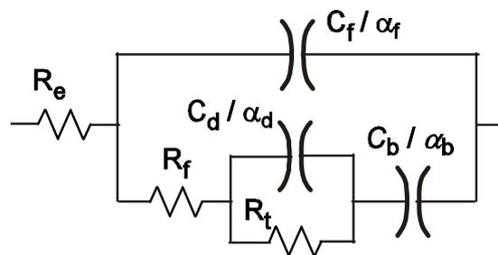
**Fig. 10.** Electrical equivalent circuit used to reproduce the impedance spectra presented in Fig. 9
