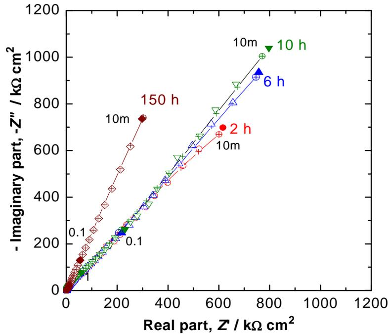
**Fig. 9.** Impedance diagrams of carbon steel in IRW+0.2% OTH for different immersion times; Disk rotation speed=600 rpm
