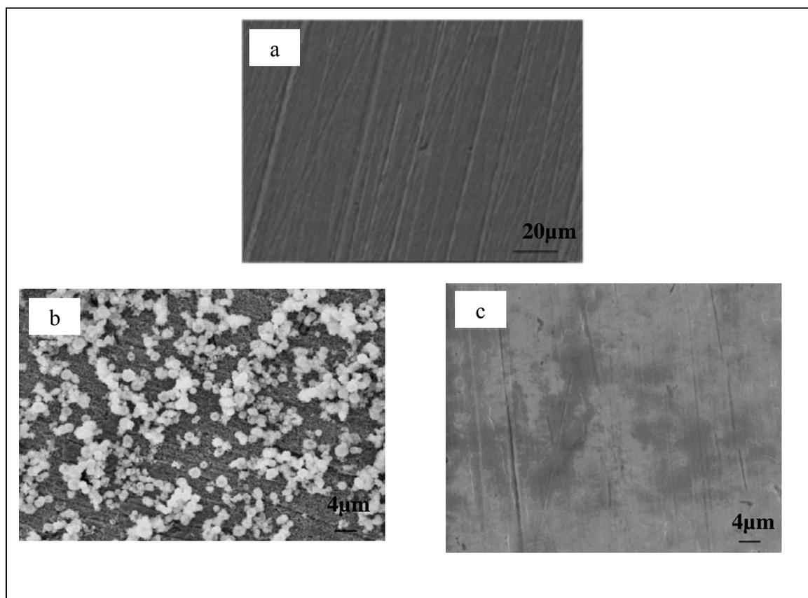
**Fig. 1.** SEM pictures (backscattered electrons) of carbon steel in presence and absence of 0.2% of inhibitor after 24 h of immersion rotated at 600 rpm (a) Carbon steel surface before experiment, (b) Carbon steel surface in (IRW) without inhibitor during 24 h, (c) Carbon steel surface in (IRW) with 0.2% of OTH during 24 h
