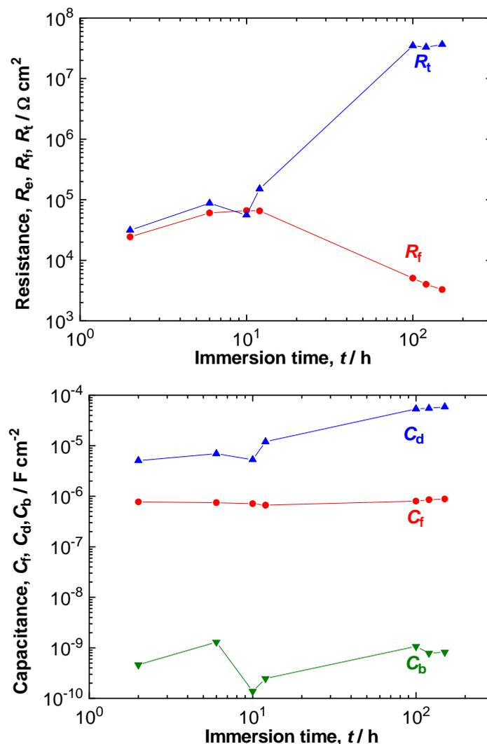
**Fig. 11.** Variation of circuit element values with immersion time for the impedance spectra presented in Fig. 9
