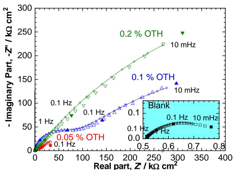
**Fig. 5.** EIS spectra of carbon steel in IRW, after 2 h of immersion. Disk rotation speed=600 rpm. Some frequencies at which the impedance was measured are also indicated together with OTH concentration
