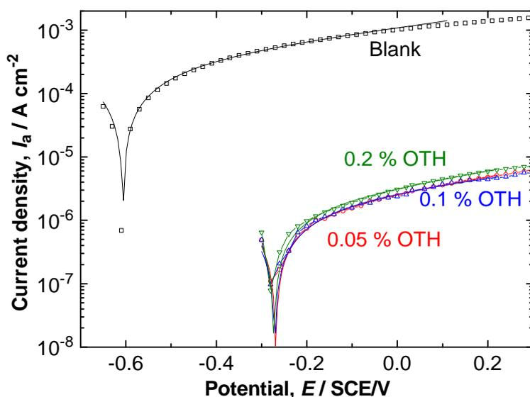
**Fig. 4.** Anodic current densities evaluated by Stern-Geary relationship in absence and in presence of OTH. Disk rotation speed at 600 rpm
