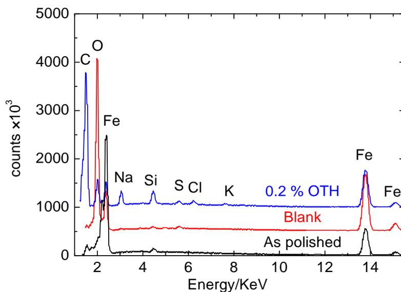
**Fig. 2.** EDS spectra for the electrode surface of carbon steel corresponding to the surface of SEM picture presented in Fig. 1: (a) as polished, (b) Blank, and (c) in presence of 0.2% OTH
