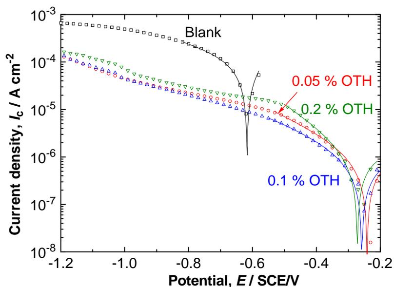
**Fig. 3.** Cathodic polarization curves of carbon steel in IRW with various OTH concentrations. Rotating disk electrode at 600 rpm
