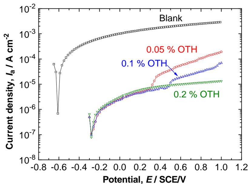
**Fig. 3.** Anodic polarization curves of carbon steel in IRW in presence of various OTH concentrations. Disk rotation speed at 600 rpm
