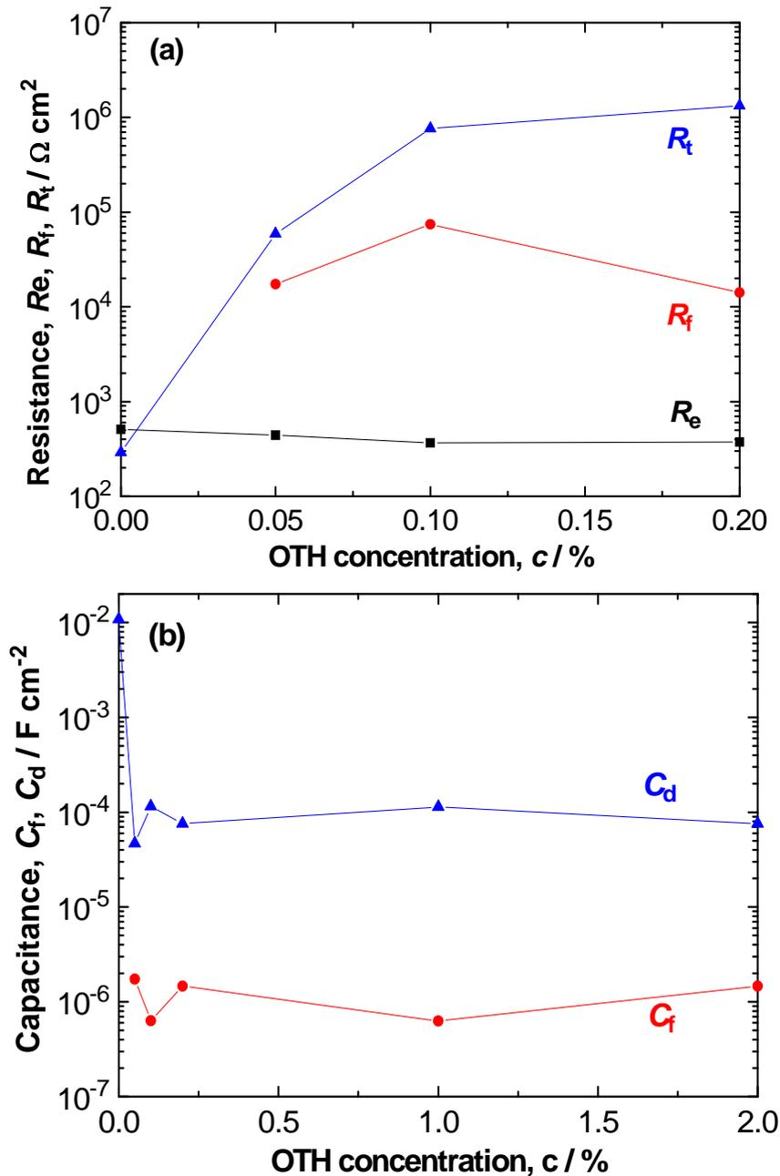
**Fig. 7.** Variation of resistances and capacitances determined by regression calculation on the results presented in Fig. 5 with the equivalent circuit of Fig. 6
