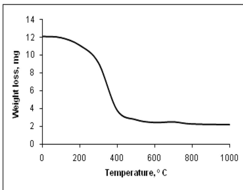
**Fig. 1.** TG curves of un-calcined NiTiO<sub>3</sub>
