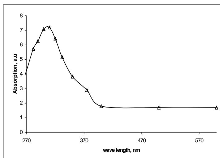
**Fig. 3.** UV-Vis spectrum of nickel titanate
