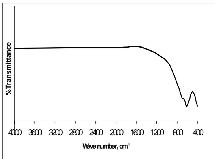
**Fig. 2.** FTIR spectra of the NiTiO<sub>3</sub> powder calcined at 850 °C
