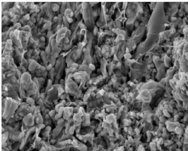
**Fig. 1.** SEM micrographs at cross section of platinum powder composite microelectrode (PPCM) with magnification x 2000
