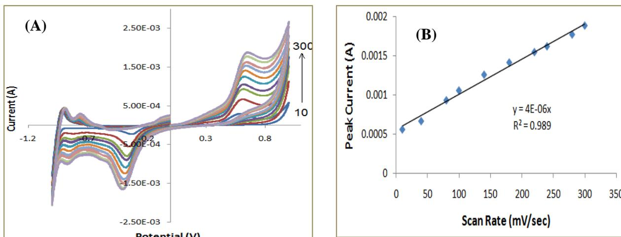
**Fig. 6.** Cyclic Voltammetry (A) and plot of peak currents as a function of scan rate of potential (B) in buffer phosphate solution with pH 4 in 1.0 g/L mefenamic acid with variation scan rate 10, 40, 80, 100, 140, 180, 220, 240, 280 and 300 mV/s
