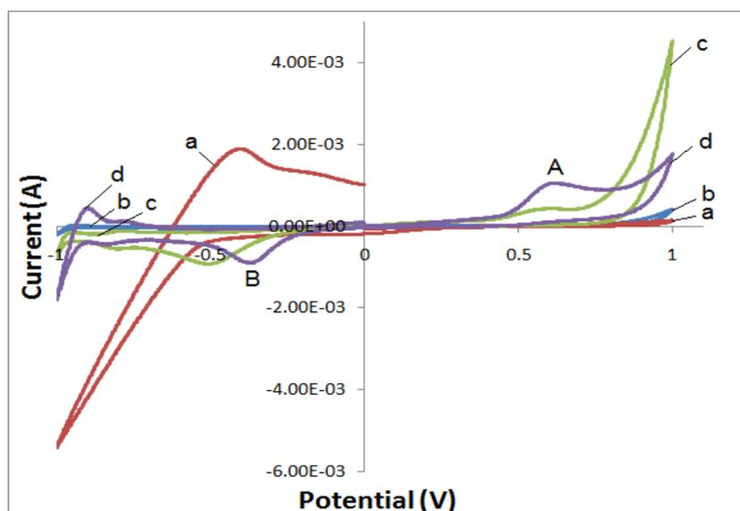
**Fig. 3.** Cyclic voltammetry of (A) buffer phosphate solution (pH 4); (B) distilled water; (C) distilled water+buffer phosphate solution (pH 4) without mefenamic acid; (D) distilled water+buffer phosphate solution (pH 4)+1.0 g/L mefenamic acid and at scan rate 100 mV/sec
