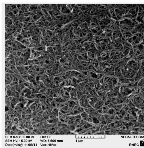
**Fig. 1.** SEM image of Nafion/MWNTs composite film on glassy carbon electrode
