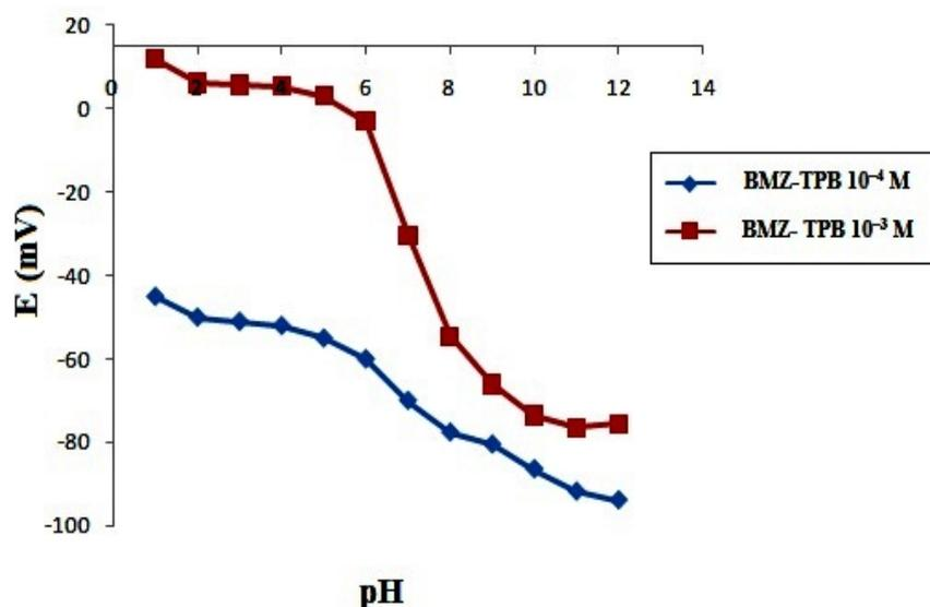
**Fig. 2.** Effect of pH on the response of bromazepam tetraphenyl borate electrode
