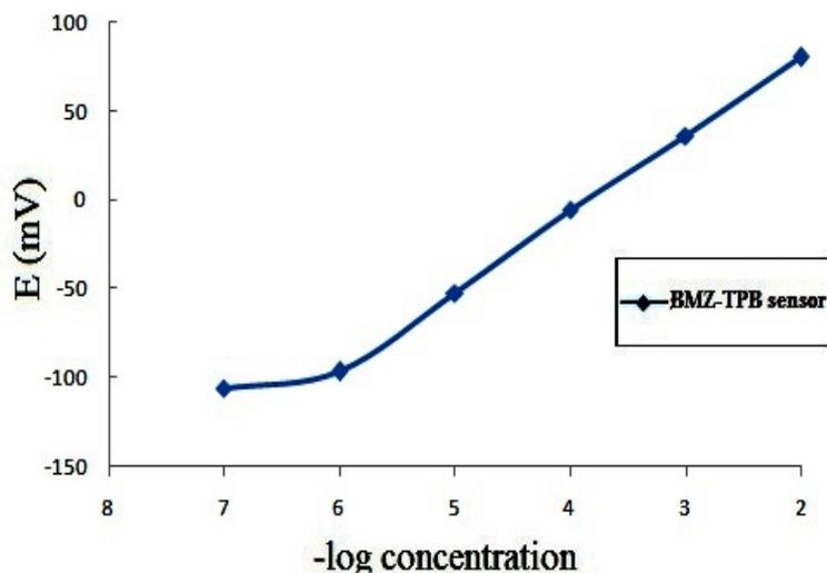
**Fig. 3.** Profile of the potential in mV to the  $-\log$  concentration of bromazepam tetraphenyl borate electrode
