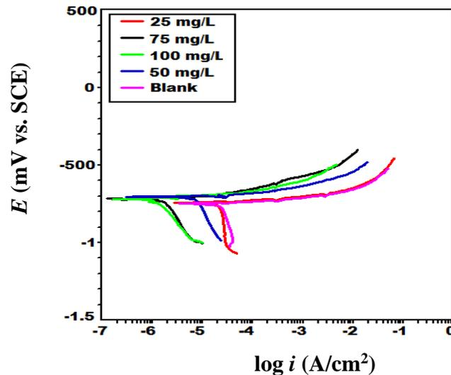
**Fig. 2.** Tafel polarization plots for aluminum alloy in 3.5% NaCl
