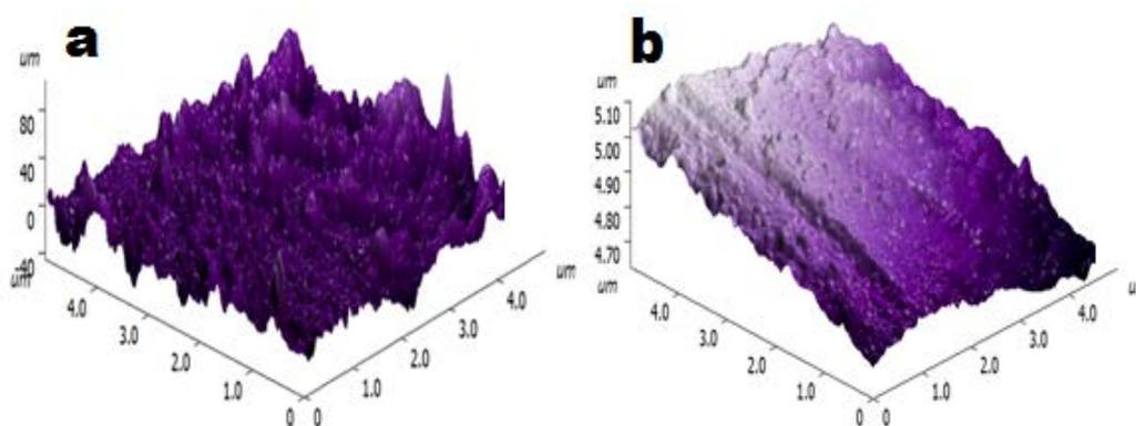
**Fig. 3.** AFM images (a) Blank (b) Inhibitor
