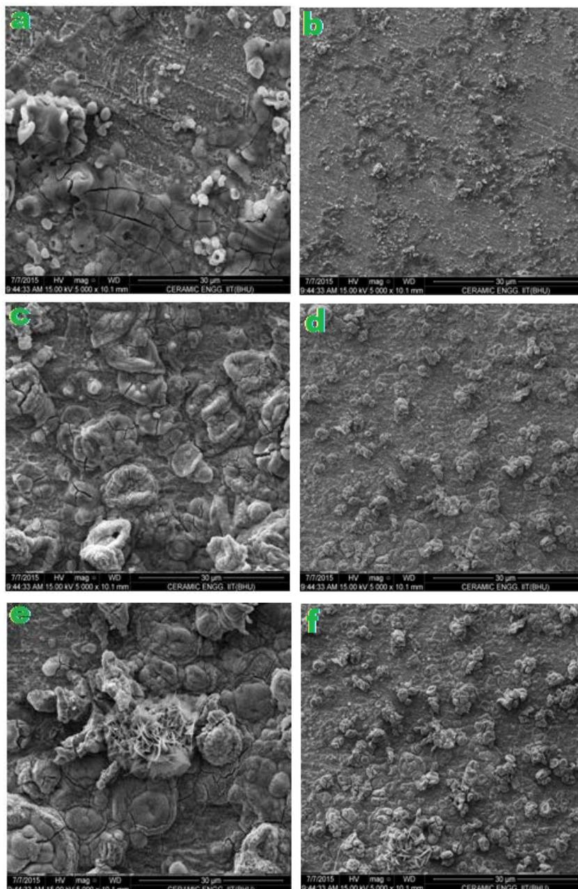
**Fig. 2.** SEM images (a) Blank at 308 K; (c) Blank at 318 K; (e) Blank at 328 K; (b) Inhibitor at 308 K; (d) Inhibitor at 318 K; (f) Inhibitor at 328 K
