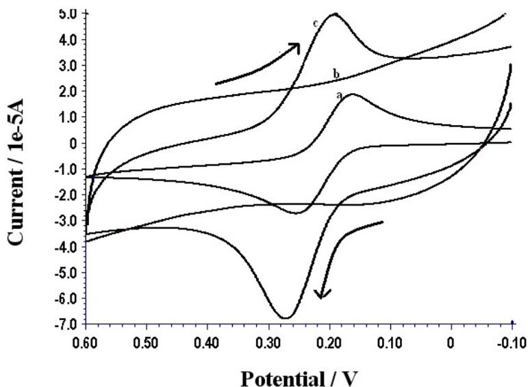
**Fig. 3.** Cyclic voltammograms recorded for the oxidation of 1.0 mM DA at BCPE (curve a) and poly(amoxicillin) MCPE (curve c) in 0.2 M ABS of pH 6.0. In the absence of DA (curve b)
