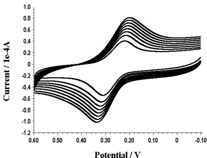
**Fig. 4.** Cyclic voltammograms of 1.0 mM DA at poly(amoxicillin) MCPE at different scan rates (a-h: 50, 60, 70, 80, 90, 100, 110, 120,  $\text{mVs}^{-1}$ ) in 0.2 M ABS of pH 5.0
