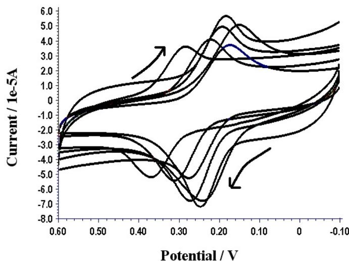
Fig. 6. Cyclic voltammograms obtained for the oxidation of 1.0 mM DA at poly(amoxicillin) MCPE in 0.2 M ABS of different pH values with the scan rate of  $50 \text{ mVs}^{-1}$
