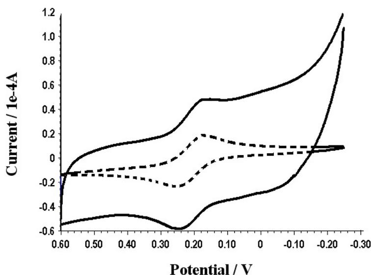
**Fig. 2.** Cyclic voltammograms obtained for the electrochemical response of 1mM  $\text{K}_4[\text{Fe}(\text{CN})_6]$  at BCPE (dotted line) and poly(amoxicillin) MCPE (solid line) in 1 M KCl at scan rate of  $50 \text{ mVs}^{-1}$
