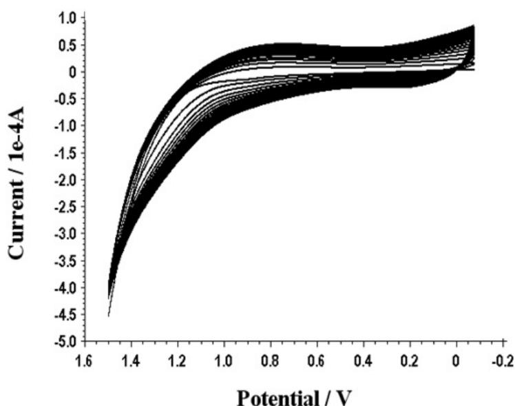
**Fig. 1.** Cyclic voltammograms obtained during the electropolymerisation of amoxicillin on the surface of BCPE
