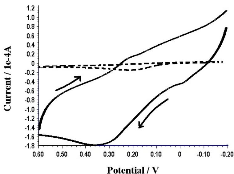
Fig. 8. Cyclic voltammograms obtained for the oxidation of 6.0 mM AA at BCPE (dashed line) and poly(amoxicillin) MCPE (solid line) in 0.2 M ABS (pH 6.0) at a scan rate  $50 \text{ mVs}^{-1}$
