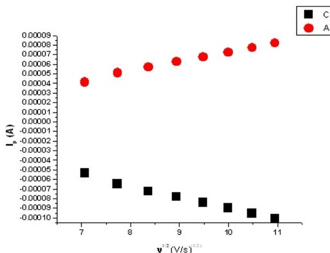
Fig. 5. Graph of peak current versus square root of scan rate
