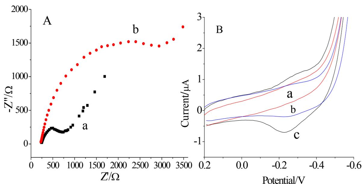
**Fig. 3.** EIS (A) of CS-p-Ppy/Au (a) and HRP/CS-porous-Ppy/Au (b) in 0.1 M, KCl that contained 5.0 mM  $[\text{Fe}(\text{CN})_6]^{3-/4-}$ , and CVs (B) of porous-Ppy/Au (a), HRP/cs/Au (b), and HRP/CS-porous-Ppy/Au(c) in 0.1 M, PBS (pH 7.0) with scan rate  $100 \text{ mV s}^{-1}$
