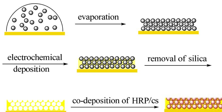
**Scheme 1.** Schematic representation of the fabrication procedure for 3D porous- Ppy/Au and HRP immobilization
