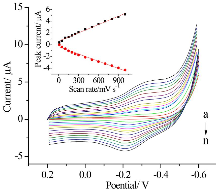
**Fig. 4.** Cyclic voltammograms of HRP/CS-porous-Ppy/Au at several scan rates: (from a to n: 10, 50, 100, 150, 200, 250, 300, 400, 500, 600, 700, 800, 900, and 1000  $\text{mVs}^{-1}$ ). Insert is the relationship between peaks current and scan rates
