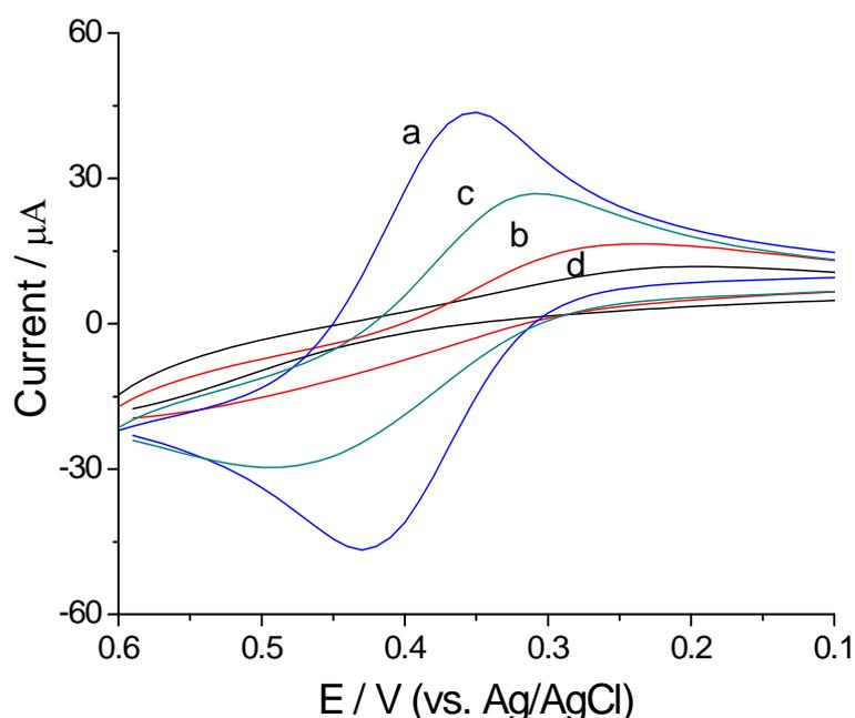
**Fig. 1.** The cyclic voltammograms of (a) bare Au, (b) silica-Ppy/Au, (c) porous-Ppy/Au, and (d) re-coupled silica on porous-Ppy/Au in 0.1 M KCl that contained 5.0 mM  $[\text{Fe}(\text{CN})_6]^{3-/4-}$  at  $100 \text{ mVs}^{-1}$ . The Ppy was electrodeposited in a 0.1 M pH 2.0 KCl+HCl+0.05 M pyrrole solution through 9 cycles of CV
