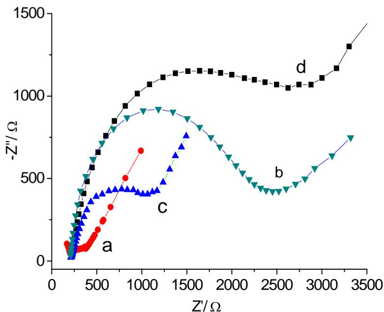
**Fig. 2.** EIS of (a) bare Au, (b) silica-Ppy/Au, (c) porous-Ppy/Au, and (d) re-coupling of silica nanoparticles on porous-Ppy/Au in 0.1 M KCl that contained 5.0 mM  $[\text{Fe}(\text{CN})_6]^{3-/4-}$
