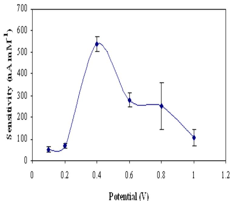
**Fig. 2.** Hydrodynamic voltammogram recorded by chronoamperometry based on 50 mM phosphate buffer pH 8 containing 0.05 mM ferrocene carboxaldehyde, 0.16 mM NADH, 2 mM  $\alpha$ -ketoglutaric acid and  $\text{NH}_4\text{Cl}$  (0 to 0.5 mM), respectively
