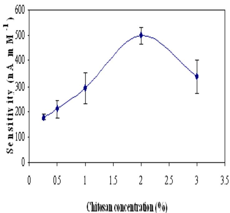
**Fig. 5.** Effect of chitosan concentration on the biosensor sensitivity. The reaction was conducted at 0.03 mM ferrocene carboxaldehyde, 0.16 mM NADH, 0.15 mM  $\alpha$ -ketoglutaric acid and  $\text{NH}_4\text{Cl}$  (0 mM to 0.5 mM), respectively. Potential was set at +0.4 V vs. Ag/AgCl
