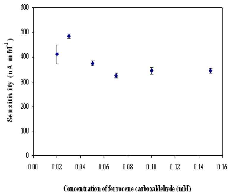
**Fig. 3.** Effect of ferrocene carboxaldehyde concentrations (0.02 mM to 0.15 mM) on the biosensor sensitivity. The experimental condition: 50 mM phosphate buffer pH 8 containing 2 mM  $\alpha$ -ketoglutaric acid, 0.16 mM NADH and ammonium ranging from 0 to 0.5 mM. Potential was set at +0.4 V vs. Ag/AgCl
