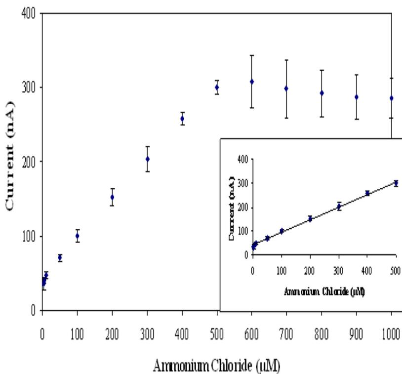
**Fig. 9.** Dynamic range of the biosensor towards different concentrations of  $\text{NH}_4\text{Cl}$  (0-1000  $\mu\text{M}$ ). Inset is the linearity of the biosensor towards  $\text{NH}_4\text{Cl}$  (2.5–500  $\mu\text{M}$ )
