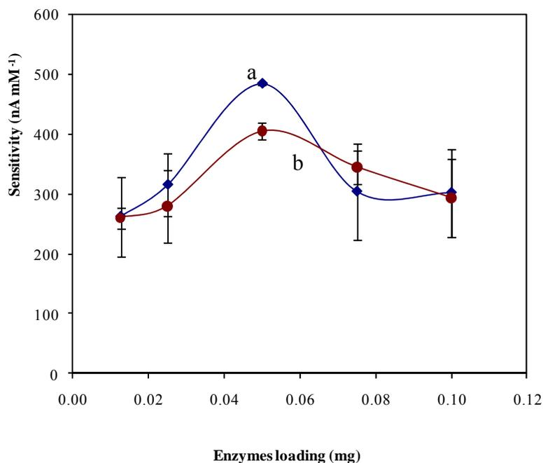
**Fig. 6.** Influence of GLDH (a) and diaphorase (b) concentrations. Sensitivity obtained from anodic current of 50 mM phosphate buffer pH 8 containing 0.16 mM NADH, 0.15 mM  $\alpha$ -ketoglutaric acid, 0.03 mM ferrocene carboxaldehyde and  $\text{NH}_4\text{Cl}$  (0 mM to 0.5 mM) at potential of +0.4 V
