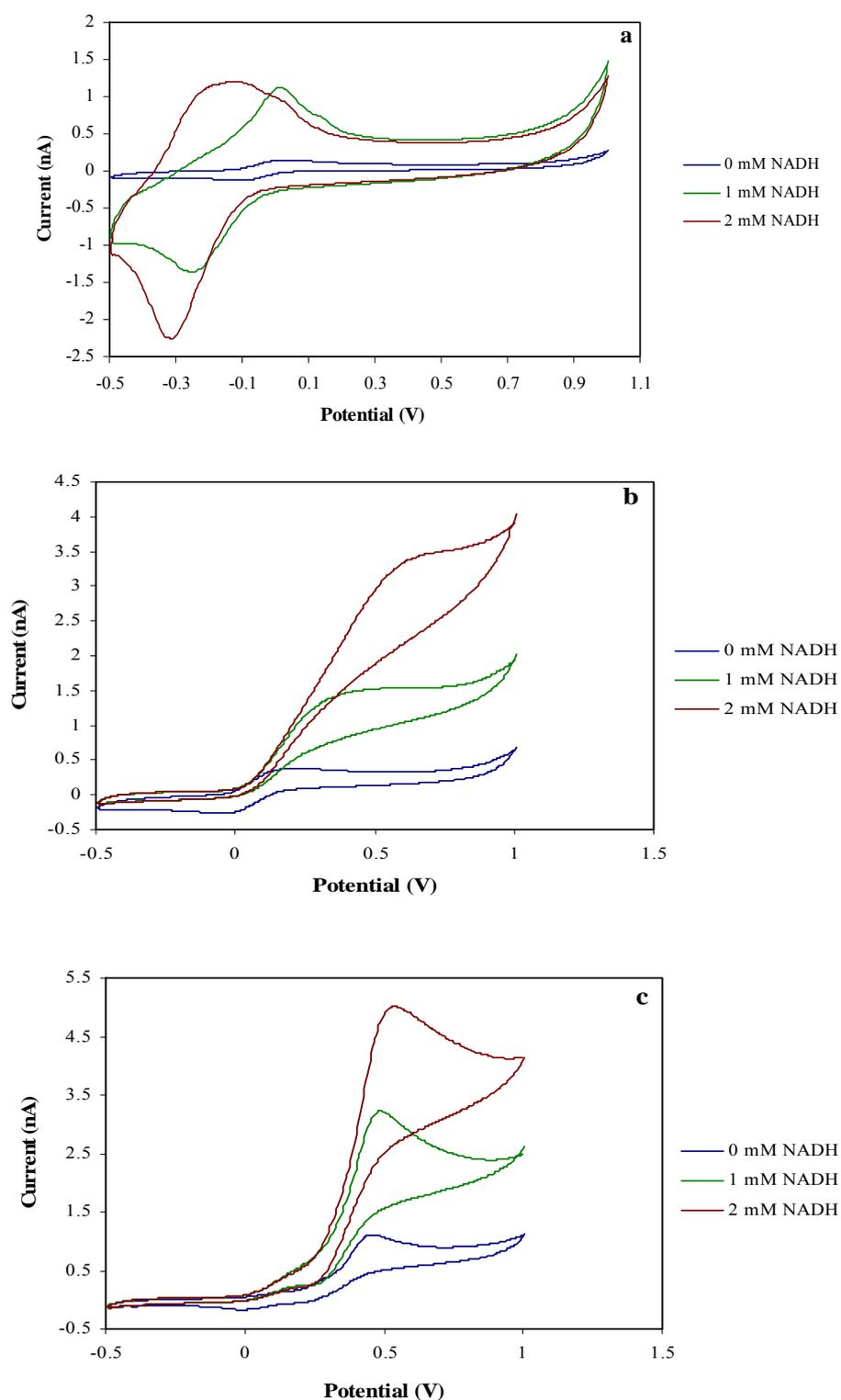
**Fig. 1.** Cyclic voltammogram of three types of ferrocene and its derivatives (a) 0.05 mM ferrocene, (b) 0.05 mM ferrocene carboxylic acid (c) 0.05 mM ferrocene carboxaldehyde in various concentrations of NADH. Scanning potential in the range of -0.5 V to +1.0 V with scan rate of  $0.05 \text{ Vs}^{-1}$  vs. Ag/AgCl
