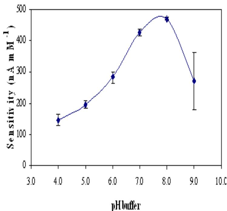
**Fig. 4.** Influence of pH on the biosensor sensitivity. Experimental condition: 50 mM phosphate buffer containing ferrocene carboxaldehyde (0.03 mM), NADH (0.16 mM),  $\alpha$ -ketoglutaric acid (2 mM) and ammonium (0 mM to 0.5 mM), respectively. Potential was set at +0.4 V vs. Ag/AgCl
