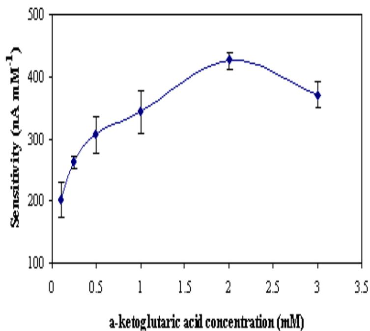
**Fig. 8.** Effect of  $\alpha$ -ketoglutaric acid concentrations on the biosensor sensitivity. The concentration of ferrocene carboxaldehyde and NADH were fixed at 0.03 mM and 0.16 mM, respectively. Concentration of  $\text{NH}_4\text{Cl}$  ranging from 0 to 0.5 mM
