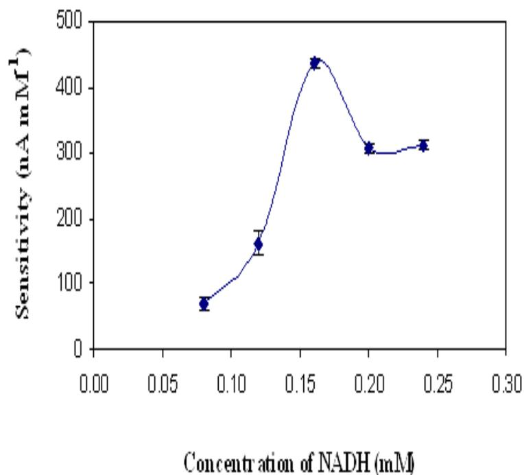
**Fig. 7.** Effect of NADH concentrations on the biosensor sensitivity. The reaction was carried out at 0.03 mM ferrocene carboxaldehyde, 0.15 mM  $\alpha$ -ketoglutaric acid and  $\text{NH}_4\text{Cl}$  ranging from 0 mM to 0.5 mM. Potential was set at +0.4 V vs. Ag/AgCl
