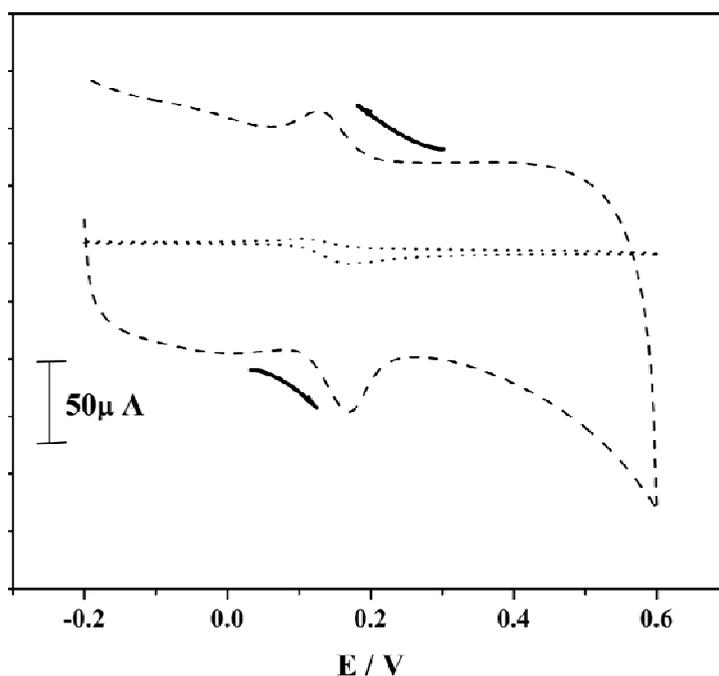
**Fig. 2.** Cyclic voltammogram in 0.2 M phosphate buffer solution pH 7.2 at BCPE (dotted line) and SDS/ $Li_2ZrO_3$  nanoparticle MCPE (dashed line) of  $0.1 \times 10^{-4}$  M DA with scan rate of  $50\text{ mV s}^{-1}$
