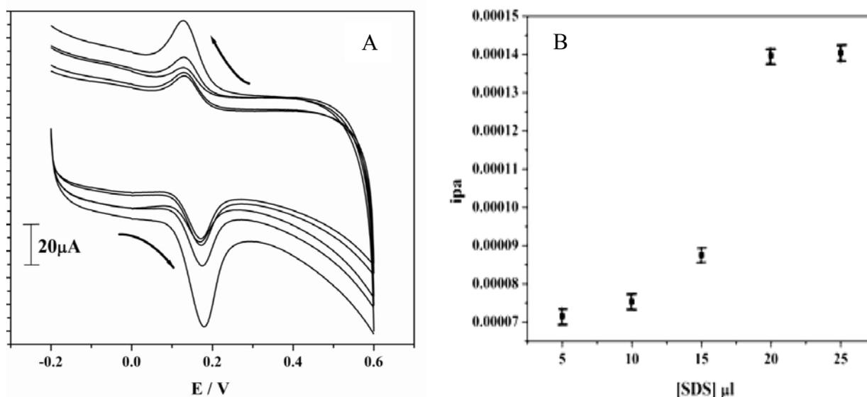
**Fig. 4.** A) Cyclic voltammogram of SDS at different concentration at SDS/  $\text{Li}_2\text{ZrO}_3$  nanoparticle MCPE in 0.2 M PBS of pH 7.2 B) Graph of current  $\text{V s}^{-1}$  concentration of SDS at scan rate  $50 \text{ mV s}^{-1}$  of pH 7.2
