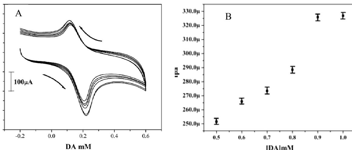
**Fig. 3.** A) Cyclic voltammogram of DA at different concentration at SDS/  $\text{Li}_2\text{ZrO}_3$  nanoparticle MCPE in 0.2 M PBS of pH 7.2 B) Graph of current  $\text{V s}^{-1}$  concentration of DA at scan rate  $50 \text{ mV s}^{-1}$  of pH 7.2
