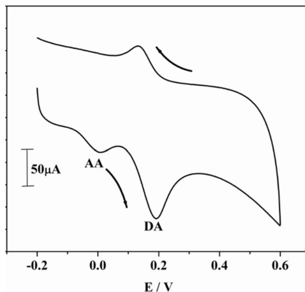
**Fig. 5.** Cyclic voltammogram obtained for oxidation of AA and DA at  $\text{SDS}/\text{Li}_2\text{ZrO}_3$  nanoparticle MCPE (solid line) at scan rate of  $50 \text{ mV s}^{-1}$ ,  $0.2 \text{ M PBS}$  (pH 7.2)
