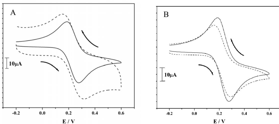
**Fig. 1.** A) Cyclic voltammogram of 1 mM  $[K_4Fe(CN)_6]$  at BCPE (solid line) and SDS/ $Li_2ZrO$  nanoparticle MCPE (dotted line) in 1 M KCl scan rate  $50\text{ mV s}^{-1}$  B) Cyclic voltammogram of 1 mM  $[K_4Fe(CN)_6]$  at BCPE (solid line) and  $Li_2ZrO_3$  nanoparticle MCPE (dotted line) in 1 M KCl scan rate  $50\text{ mV s}^{-1}$
