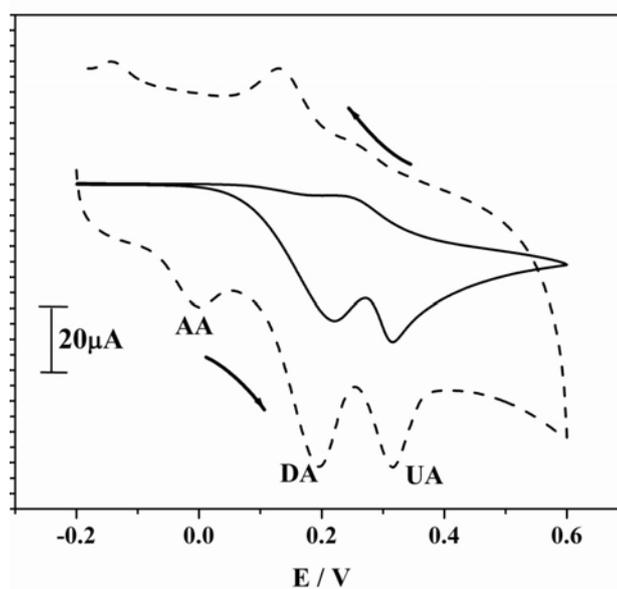
**Fig. 6.** Cyclic voltammogram obtained for the oxidation of AA, UA and DA at  $\text{SDS}/\text{Li}_2\text{ZrO}_3$  nanoparticle MCPE (solid line) at bare (dotted line) at scan rate of  $50 \text{ mV s}^{-1}$ ,  $0.2 \text{ M PBS}$  (pH 7.2)
