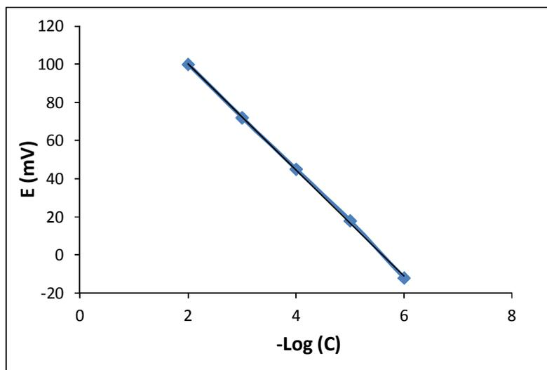
**Fig. 3.** Profile of the potential in mV to  $-\log$  concentration in  $\text{mol L}^{-1}$  obtained with sensor
