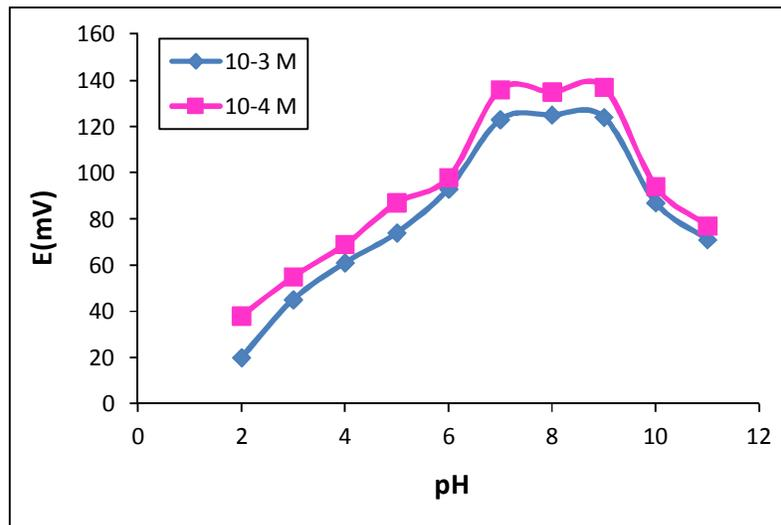
Fig. 4. Effect of pH on the response of LAM sensor
