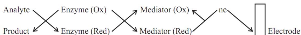
**Fig. 2.** The mediated electron transfer CP-based electrochemical sensor function scheme
