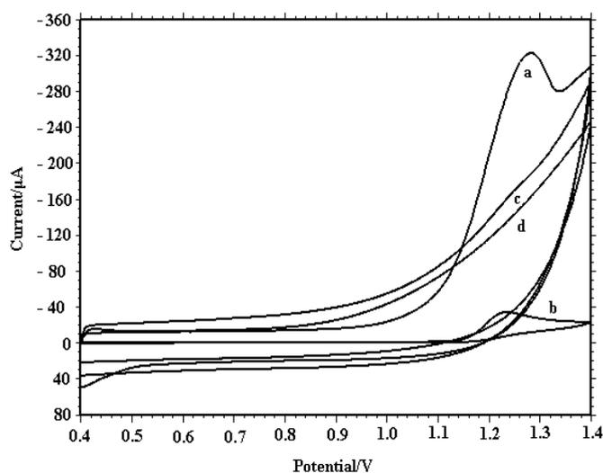
**Fig. 1.** Cyclic voltammograms of  $1 \times 10^{-3}$  MET on MWCNT-modified GCE (a) and bare GCE (b), Blank CVs of MWCNT-modified GCE (c), and bare GCE (d). Scan rate:  $50 \text{ mVs}^{-1}$ ; supporting electrolyte: 0.2 M phosphate buffer with pH 3.0; accumulation time: 60 s (at open circuit); volume of MWCNTs suspension: 12  $\mu\text{L}$
