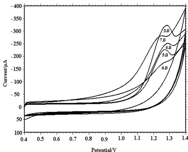
**Fig. 3.** Influence of pH on the shape of anodic peak of  $1.0 \times 10^{-3}$  M MET on MWCNTs glassy carbon electrode at scan rate  $50 \text{ mVs}^{-1}$  in phosphate buffer
