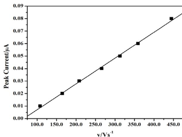
**Fig. 5.** Dependence of the oxidation peak current on scan rate
