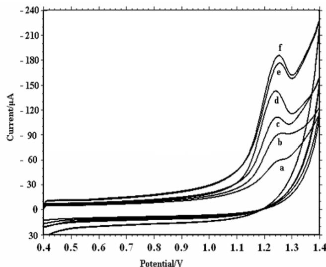
**Fig. 6.** Cyclic voltammograms of MWCNT-modified GCE in MET solution at different concentrations (a) 6.0; (b) 10.0; (c) 20.0; (d) 40.0; (e) 60.0; (f) 80.0  $\mu\text{M}$ . Inset: Plot of the peak current against the concentration of MET
