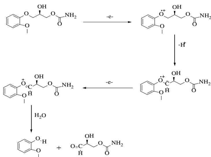
**Scheme 2.** Possible electrode reaction mechanism of MET
