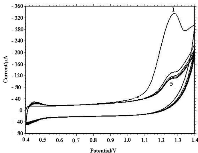
**Fig. 2.** Successive cyclic voltammograms of  $1.0 \times 10^{-3}$  M MET on MWCNT-modified GCE
