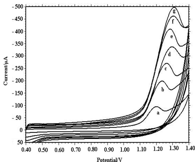
**Fig. 4.** Cyclic voltammograms of  $1.0 \times 10^{-3}$  M MET on MWCNT-modified GCE with different scan rates. (a)-(g) 10, 20, 40, 50, 60, 80 and  $120 \text{ mVs}^{-1}$ , respectively
