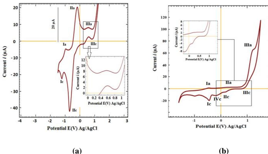
**Fig. 3.** CV of (a)  $\text{Fe}[\text{Me}_2\text{-(DBDPy)N}_6\text{tetraoxo[18]Cl}_2]\text{Cl}$  and (b) CV of  $\text{Ni}[\text{Me}_2\text{-(DBDPy)N}_6\text{tetraoxo[18]Cl}_2]$ , recorded in DMSO ( $1 \times 10^{-3}$  M) containing 0.1 M TEAP solution as supporting electrolyte at a scan rate of  $100 \text{ mVs}^{-1}$ . The inserts are enlarged portions of the CVs indicated by the arrows.
