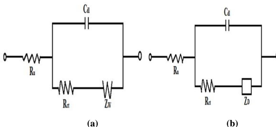
**Fig. 11.** (a) Randles equivalent circuit for Ni[Me<sub>2</sub>-(DBDPy)N<sub>6</sub>tetraoxo[18]Cl<sub>2</sub>] monomer; (b) Randles equivalent circuit for polymeric film of Ni[Me<sub>2</sub>-(DBDPy)N<sub>6</sub>tetraoxo[18]Cl<sub>2</sub>]
