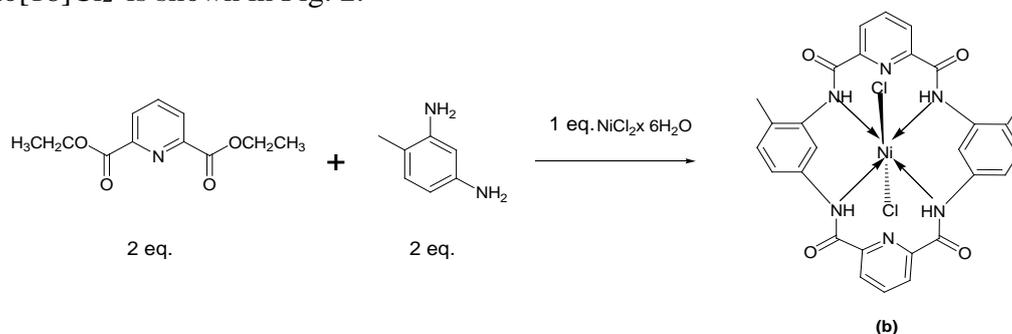
**Fig. 2.** Scheme for the synthesis of macrocyclic complex,  $\text{Ni}[\text{Me}_2\text{-(DBDPy)N}_6\text{tetraoxo[18]Cl}_2]$  (b)
