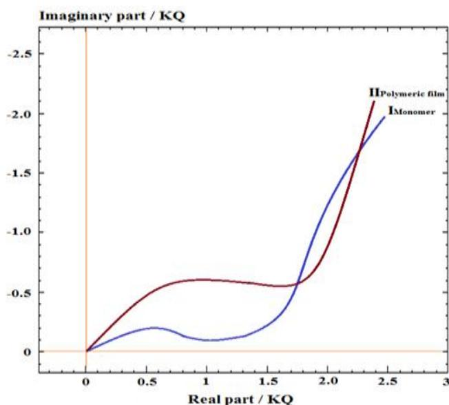
**Fig. 10.** (I) Nyquist plot for Ni[Me<sub>2</sub>-(DBDPy)N<sub>6</sub>tetraoxo[18]Cl<sub>2</sub>] monomer (II) Nyquist plot for polymeric film of Ni[Me<sub>2</sub>-(DBDPy)N<sub>6</sub>tetraoxo[18]Cl<sub>2</sub>]
