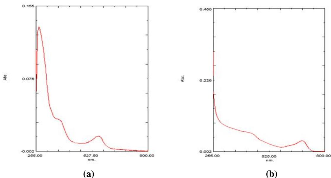
**Fig. 7.** (a) UV-Vis spectra of Fe[Me<sub>2</sub>-(DBDPy)N<sub>6</sub>tetraoxo[18]Cl<sub>2</sub>]Cl as monomer and (b) UV-Vis spectra of Fe[Me<sub>2</sub>-(DBDPy)N<sub>6</sub>tetraoxo[18]Cl<sub>2</sub>]<sub>n</sub>Cl as polymer
