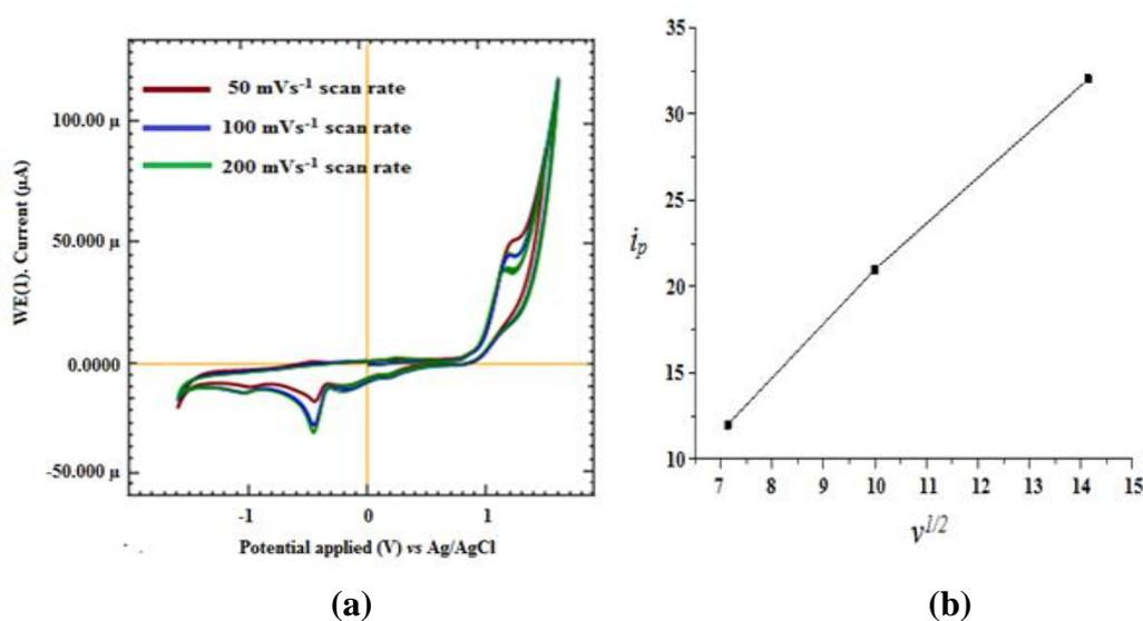
**Fig. 5.** (a) CV of  $\text{Ni}[\text{Me}_2\text{-(DBDPy)N}_6\text{tetraoxo[18]Cl}_2]$  at different scan rates (50-200  $\text{mVs}^{-1}$ ) and (b) Plot of  $i_p$  vs  $v^{1/2}$  for  $\text{Ni}[\text{Me}_2\text{-(DBDPy)N}_6\text{tetraoxo[18]Cl}_2]$
