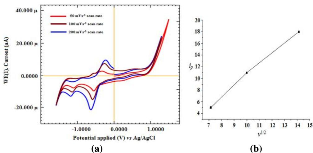
**Fig. 4.** (a) CV of  $\text{Fe}[\text{Me}_2\text{-(DBDPy)N}_6\text{tetraoxo[18]Cl}_2]\text{Cl}$  at different scan rates (50-200  $\text{mVs}^{-1}$ ) and; (b) Plot of  $i_p$  vs  $v^{1/2}$  for  $\text{Fe}[\text{Me}_2\text{-(DBDPy)N}_6\text{tetraoxo[18]Cl}_2]\text{Cl}$
