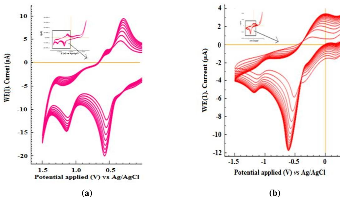
**Fig. 6.** Repeated scan CV of (a)  $\text{Fe}[\text{Me}_2\text{-(DBDPy)N}_6\text{-tetraoxo[18]Cl}_2]$  Cl and (b) CV of  $\text{Ni}[\text{Me}_2\text{-(DBDPy)N}_6\text{-tetraoxo[18]Cl}_2]$  showing electropolymerisation, recorded in DMSO ( $1 \times 10^{-3}$  M) containing 0.1 M TEAP solution as supporting electrolyte at 100  $\text{mVs}^{-1}$  scan rate. The inserts are enlarged portions of the CVs indicated by the arrows.
