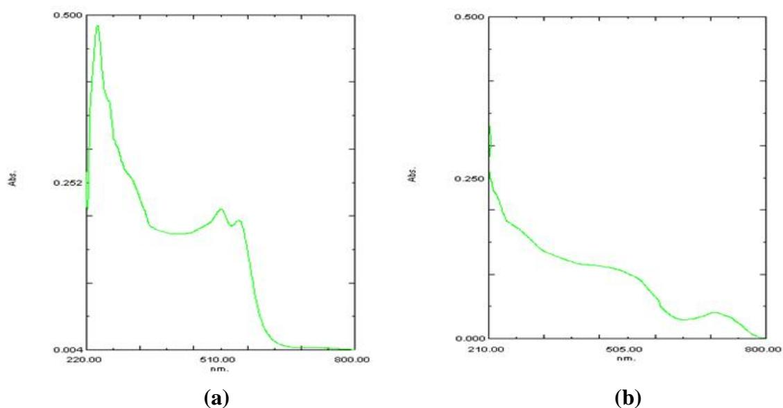
**Fig. 8.** (a) UV-Vis spectra of Ni[Me<sub>2</sub>-(DBDPy)N<sub>6</sub>tetraoxo[18]Cl<sub>2</sub>] as monomer and (b) UV-Vis spectra of Ni[Me<sub>2</sub>-(DBDPy)N<sub>6</sub>tetraoxo[18]Cl<sub>2</sub>]<sub>n</sub> as polymer
