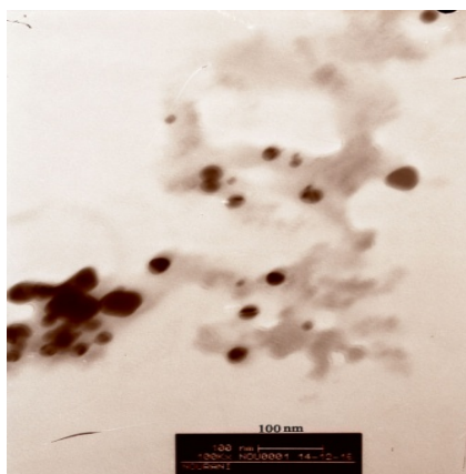
Fig. 3. TEM image of silver nanoparticle
