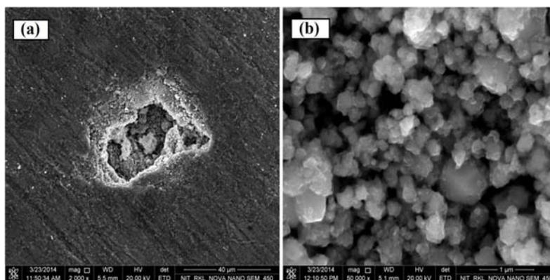
**Fig. 9.** (a) FESEM images of duplex (sintered at 1300 °C) corroded in 0.5 M NaCl concentration; (b) High resolution image of corroded region inside the pit
