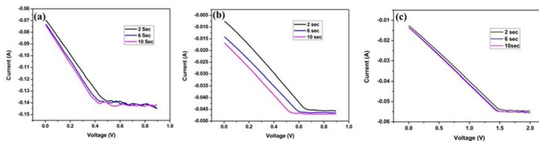
**Fig. 6.** Potentiometric curves duplex stainless steel consolidated at (a) 1100 °C (b) 1200 °C and (c) 1300 °C in 0.5 M NaCl solution at different quiet time (2 to 10 seconds)
