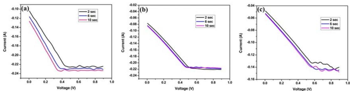
**Fig. 7.** Potentiometric curves duplex stainless steel consolidated at (a) 1100 °C (b) 1200 °C and (c) 1300 °C in 1 M NaCl solution at different quiet time (2 to 10 seconds)
