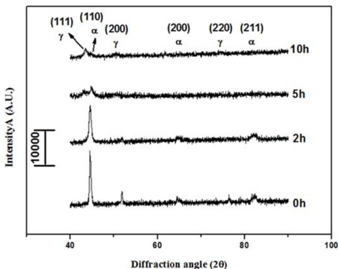
**Fig. 1.** XRD spectra of duplex stainless steel powder milled for 0, 2, 5 and 10 h respectively
