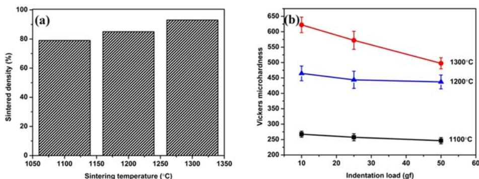
**Fig. 5.** Graph of (a) Sintered density (b) Vickers microhardness versus indentation load (10, 25 and 50 gf) of duplex stainless steel samples sintered at 1100, 1200 and 1300 °C in argon atmosphere
