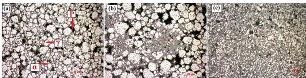
**Fig. 4.** Optical microstructure of duplex stainless steel samples sintered at 1100, 1200 and 1300 °C in argon atmosphere (P- Pores)
