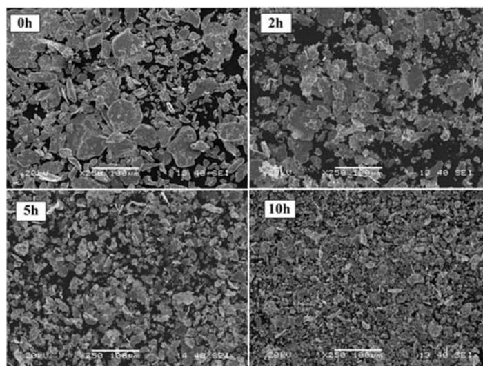
**Fig. 2.** SEM micrographs of duplex stainless steel powders milled at different time intervals (0 to 10 h)
