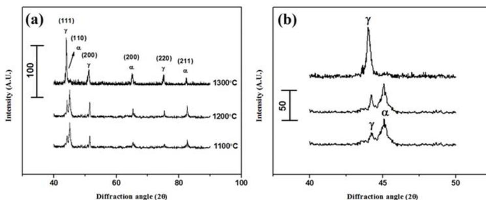
**Fig. 3.** (a) X-ray diffraction patterns of duplex stainless steel samples consolidated at 1100, 1200 and 1300  $^{\circ}\text{C}$  respectively; (b) The enlarge view (scan range 40–50 $^{\circ}$ ) of the first peak of duplex stainless steel
