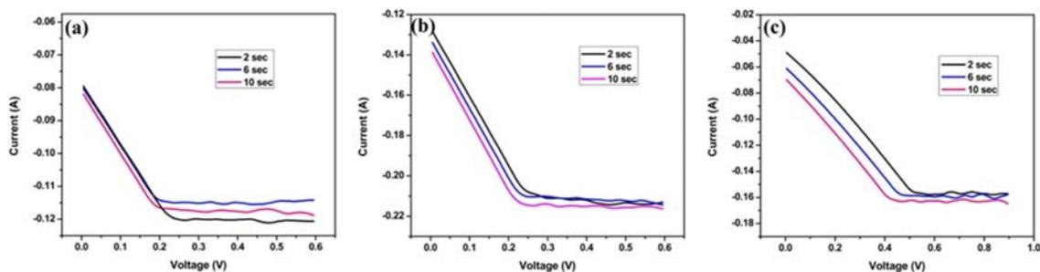
**Fig. 8.** Potentiometric curves duplex stainless steel consolidated at (a) 1100 °C (b) 1200 °C and (c) 1300 °C in 2 M NaCl solution at different quite time (2 to 10 seconds)
