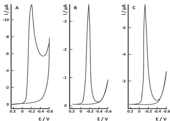
**Fig. 2.** Cathodic voltammograms at CSPE (type 3) in 0.1 M HNO<sub>3</sub> registered without addition and after addition of 40 mg L<sup>-1</sup> TZ at different VA modes: linear (a); differential pulse (b); square wave (c). Scan rate=60 mVs<sup>-1</sup>, pulse step=6 mV, pulse amplitude=20 mV, frequency=50 Hz
