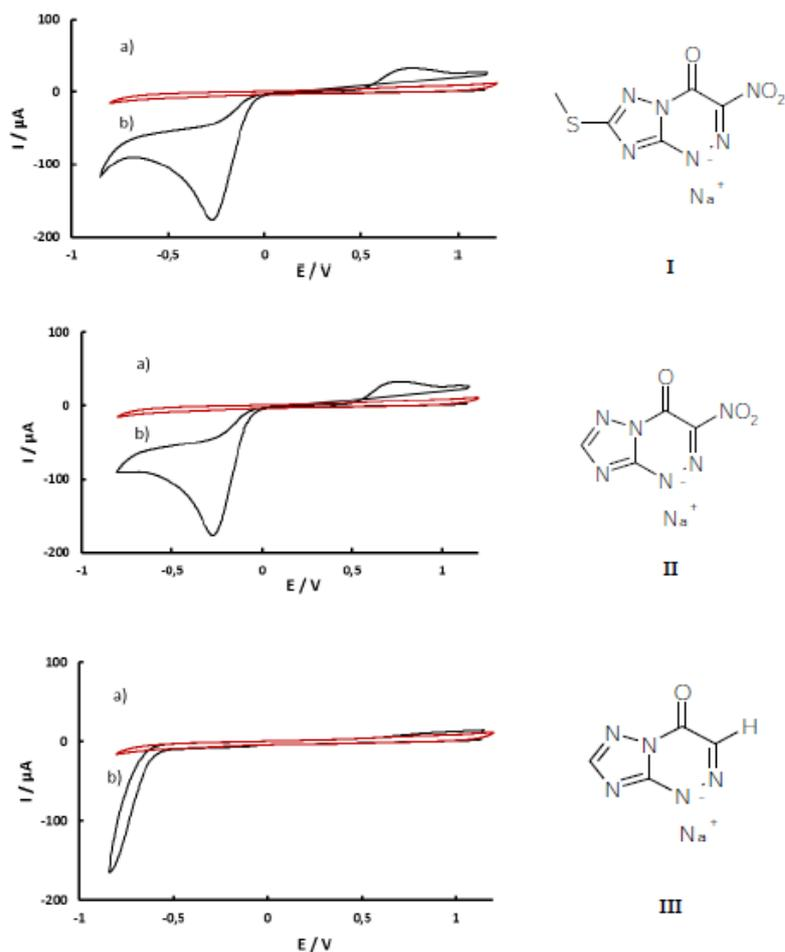
**Fig. 1.** Cyclic voltammograms at glassy carbon electrode in 0.1 M HNO<sub>3</sub> registered at a scan rate of 0.1 Vs<sup>-1</sup> without addition (1) and after addition (2) of 5 mM compounds I - III
