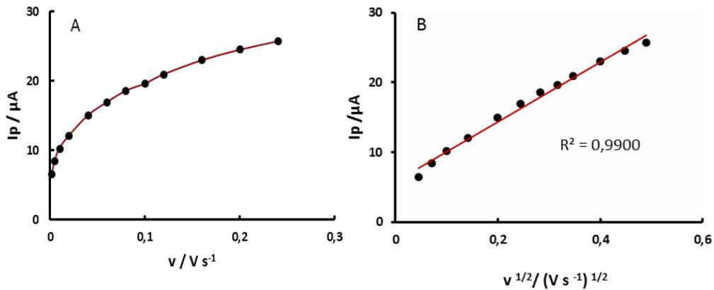
**Fig. 4.** A) Plot of peak current versus scan rate; B) Plot of peak current versus square root of scan rate for 40 mg L<sup>-1</sup> TZ in 0.1 M HNO<sub>3</sub>; pulse amplitude=50 mV, pulse step=6 and 12 mV, frequency=50 Hz
