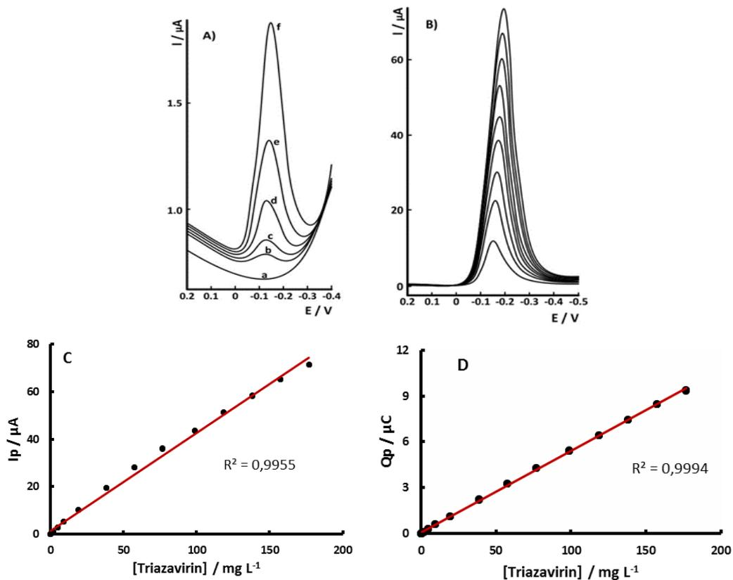
**Fig. 5.** SqW voltammograms (A) for low concentrations of TZ: (a) blank solution, (b) 0.1, (c) 0.2, (d) 0.5, (e) 1, (f) 2 mg L<sup>-1</sup>; (B) for 20 – 180 mg L<sup>-1</sup> of TZ with a step of 20 mg L<sup>-1</sup> and plots of height (C)/area (D) of TZ reduction peak versus its concentration (obtained from 3 independent measurements for each one). SqW sweep parameters: scan rate=120 mV s<sup>-1</sup>, pulse step=12 mV, pulse amplitude=50 mV, frequency=50 Hz
