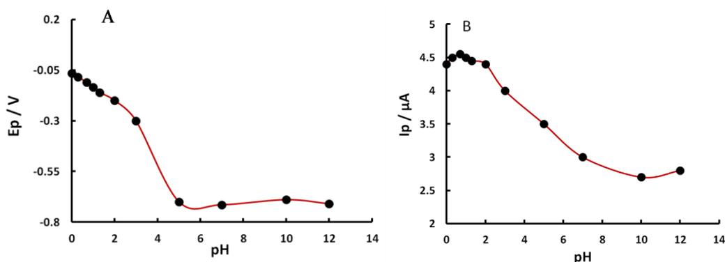
**Fig. 3.** Plot of peak potential (A) and peak current (B) versus pH for 40 mg L<sup>-1</sup> TZ, Supporting electrolyte: 1 M HNO<sub>3</sub> (pH=0); 0.5 M HNO<sub>3</sub> (pH=0.3), 0.2 M HNO<sub>3</sub> (pH=0.7); 0.1 M HNO<sub>3</sub> (pH=1); 0.05 M HNO<sub>3</sub> (pH=1.3); 0.1 M NaNO<sub>3</sub>+xM HNO<sub>3</sub> (pH=2,3), 0.1 M NaNO<sub>3</sub> (pH=5), 0.1 M NaNO<sub>3</sub>+xM NaOH (pH=7, 10, 12). SqW sweep parameters are as given in Table 1
