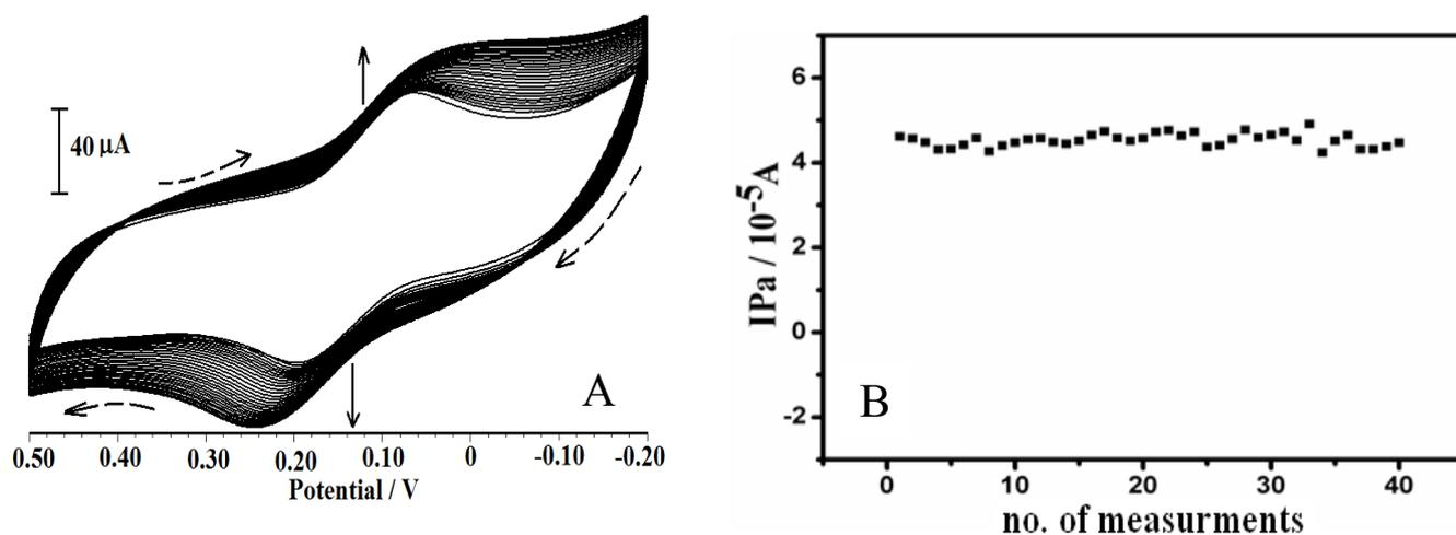
**Fig.7. A)** Cyclic voltammograms for 40 multiple cycle of  $2.0 \times 10^{-4}$  M  $\text{H}_2\text{Q}$  in 40% EtOH/0.1 M ABS solution of pH 5.0 at a scan rate of  $25 \text{ mV s}^{-1}$ , **B)** A plot of number of repetitive cycles vs.  $I_p$
