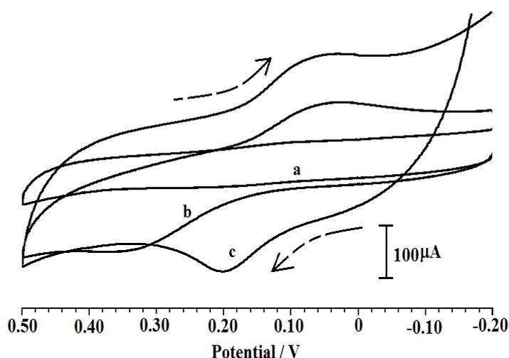
**Fig. 1.** Cyclic voltammograms for the electrochemical response of  $2 \times 10^{-4} \text{ M H}_2\text{Q}$  (a) Blank (b) Bare CPE (c) HRP-SiSG/CPE in 40% EtOH/ 0.1 M ABS at the scan rate 10 mV/S
