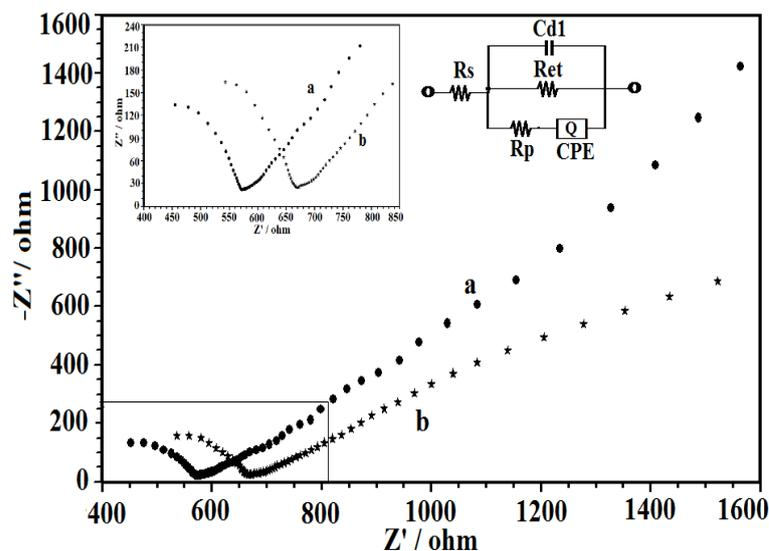
**Fig. 8.** EIS spectrum of  $H_2Q$  (a) CPE (b) HRP-SiSG/ CPE, inset equivalent circuit at HRP- SiSG/ CPE Amplitude: 5 mV, Frequency: 1 Hz to 100 KHz
