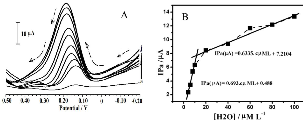
**Fig. 5.** **A)** A differential pulse voltammograms of  $H_2Q$  for different concentrations. (a)  $4 \times 10^{-5}$  M (b)  $6 \times 10^{-5}$  M (c)  $8 \times 10^{-5}$  M (d)  $1 \times 10^{-4}$  M (e)  $2 \times 10^{-5}$  M (f)  $4 \times 10^{-4}$  M (g)  $6 \times 10^{-4}$  M (h)  $8 \times 10^{-4}$  M (i)  $1 \times 10^{-3}$  M, **B)** Calibration plot of  $H_2Q$  concentration
