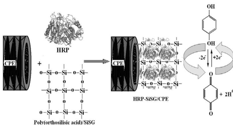
**Scheme 1.** A schematic diagram showing the steps involved in the fabrication of HRP-SiSG/CPE
