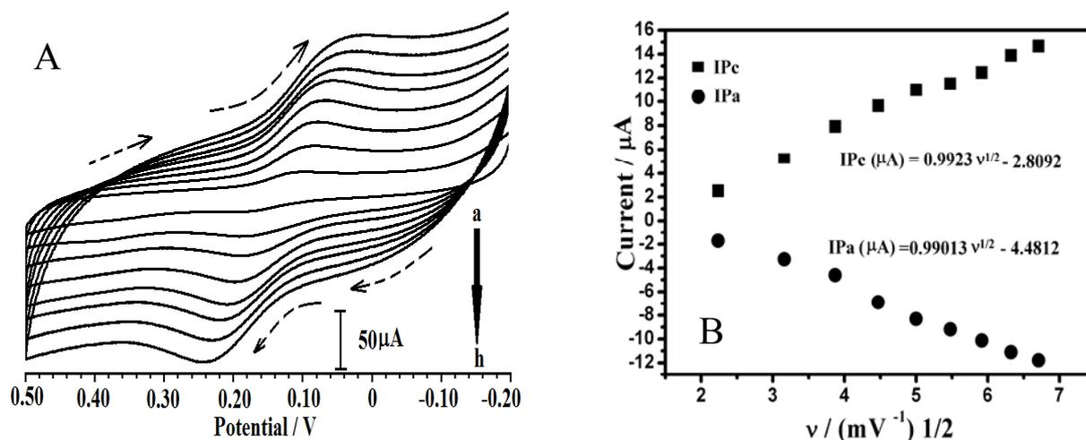
**Fig. 4.** **A)** Cyclic voltammograms of variation of scan rate for H<sub>2</sub>Q at HRP-SiSG/ CPE.(a to h, 5–40 mV/S) in 40% EtOH/ 0.1 M ABS (pH 5.0) solution, **B)** Calibration plots for the redox peak currents *vs.* the square root of scan rate
