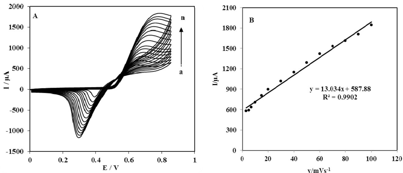
**Fig. 5.** (A) Cyclic voltammograms of Ni/Al-LDH/NMCP electrode in  $0.1 \text{ mol L}^{-1}$  NaOH containing  $0.050 \text{ mol L}^{-1}$  of methanol at various potential scan rates (from inner to outer)  $3\text{-}100 \text{ mV s}^{-1}$ . (B) Plot of  $I_p$  vs.  $v$
