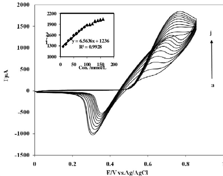
**Fig. 9.** Cyclic voltammograms of different concentrations of methanol at Ni/Al-LDH/NMCP electrode in  $0.1 \text{ mol L}^{-1}$  NaOH at a scan rate of  $50 \text{ mV s}^{-1}$ . Concentrations of methanol from (a) to (j) are  $0.01, 0.02, 0.03, 0.04, 0.05, 0.06, 0.07, 0.08, 0.09$  and  $0.1 \text{ mol L}^{-1}$ , respectively
