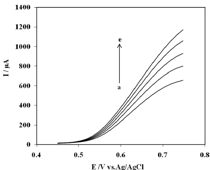
**Fig. 11.** Pseudo-steady state polarization curves of Ni-Al LDH/NMCP electrode obtained in 0.03 (a), 0.004 (b), 0.05 (c), 0.06 (d) and 0.1 (e) mol L<sup>-1</sup> methanol respectively. The potential sweep rate is 5 mVs<sup>-1</sup>
