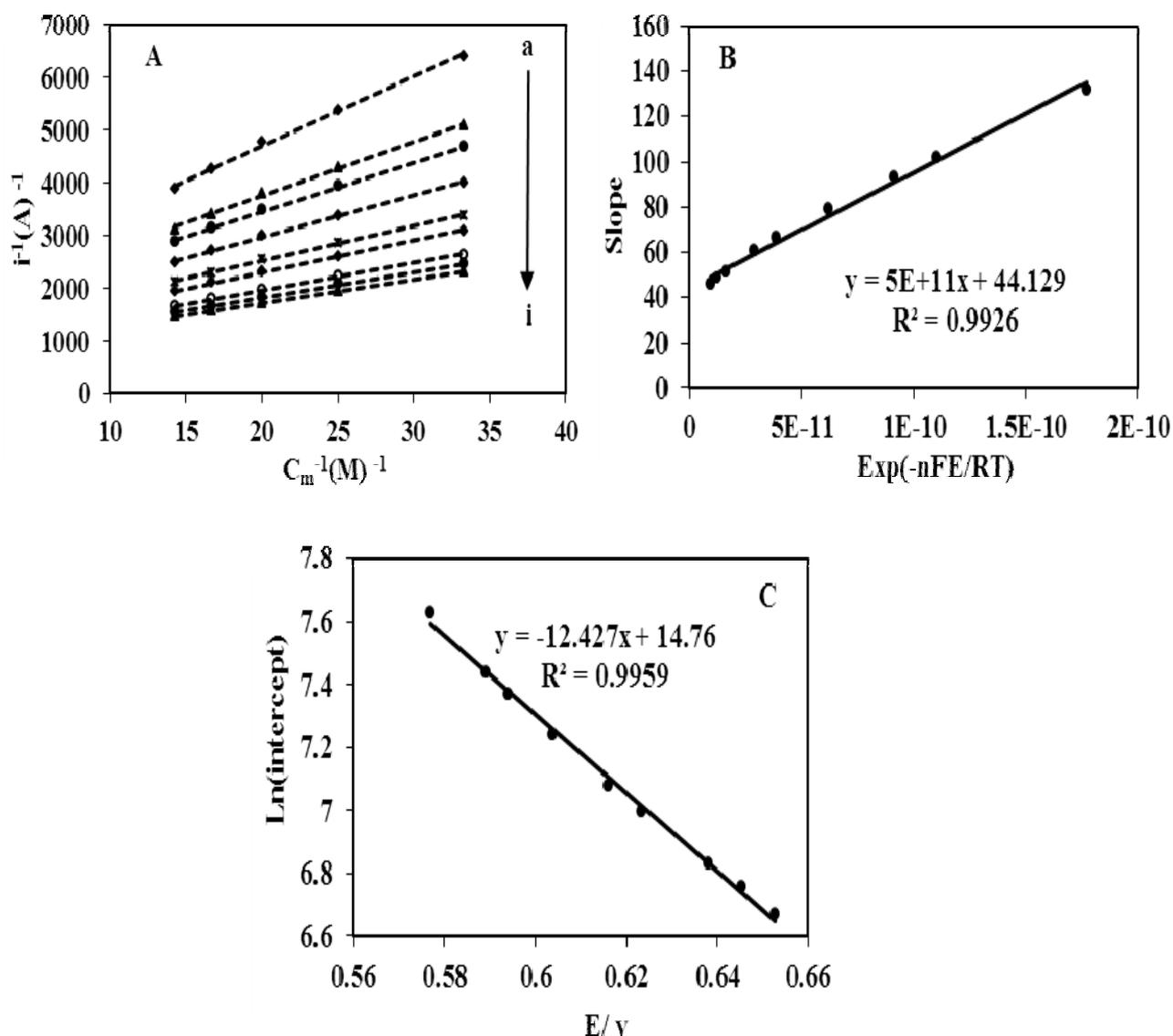
**Fig. 12.** (A) Plot of  $i^{-1}$  (from polarization curves in Fig. 11. against  $C_m^{-1}$  at various potentials: (a) 576; (b) 589; (c) 594; (d) 602; (e) 616; (f) 623; (g) 638; (h) 645 and (i) 652 mV/Ag, AgCl as curves (a–i). (B) Plot of the slopes (of curves in 12A) vs.  $\text{exp}(-nFE/RT)$ . (C) Plot of the  $\text{Ln}(\text{intercepts})$  (of curves in 12A) vs. applied potential
