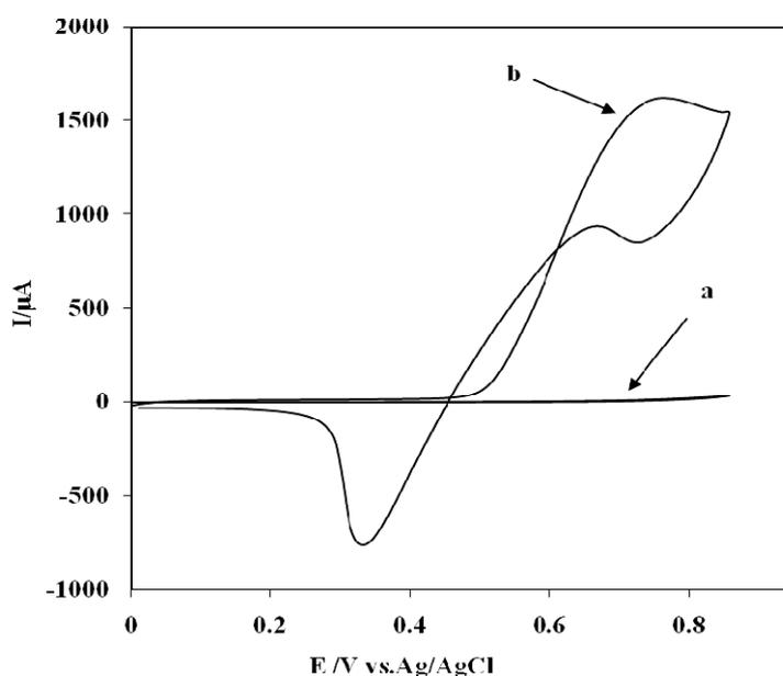
**Fig. 3.** Cyclic voltammograms of bare carbon paste (a) and Ni/Al-LDH/NMCP (b) electrode in  $0.1 \text{ mol L}^{-1}$  NaOH containing  $0.05 \text{ mol L}^{-1}$  methanol
