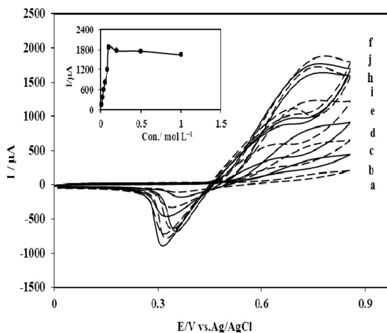
**Fig. 4.** Cyclic voltammograms of Ni/Al-LDH/NMCP electrode in  $0.05 \text{ mol L}^{-1}$  methanol containing different concentrations of NaOH at the scan rate of  $50 \text{ mV s}^{-1}$ . The NaOH concentration is (a) 0.01, (b) 0.02, (c) 0.03, (d) 0.05, (e) 0.08, (f) 0.1, (g) 0.2, (h) 0.5, and (i)  $1.0 \text{ mol L}^{-1}$ . The inset displays the peak currents vs. NaOH concentration
