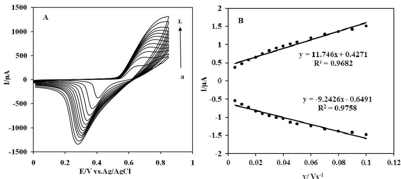
**Fig. 2.** (A) Cyclic voltammograms of Ni/Al-LDH/NMCP electrode in  $0.1 \text{ mol L}^{-1} \text{ NaOH}$  at various potential scan rates: (a) 5, (b) 10, (c) 15, (d) 20, (e) 30, (f) 40, (g) 50, (h) 60, (i) 70, (j) 80, (k) 90 and (l)  $100 \text{ mV s}^{-1}$ . (B) The dependency of anodic and cathodic peak currents vs. scan rate
