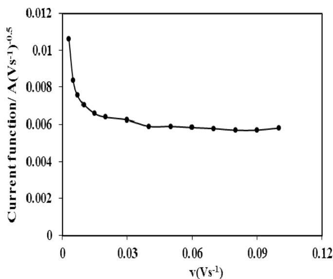
**Fig. 6.** Current function vs.  $v$  for  $0.1 \text{ mol L}^{-1}$  NaOH solution in the presence of  $0.050 \text{ mol L}^{-1}$  methanol
