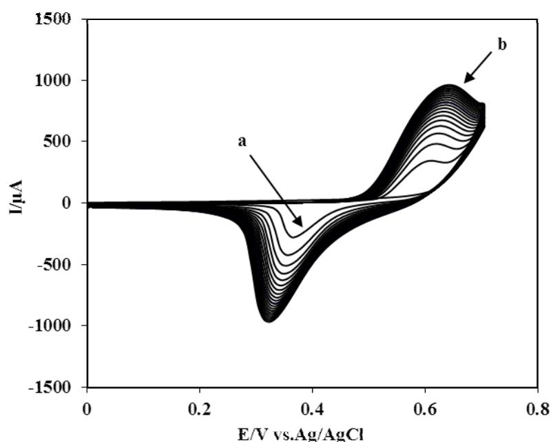
**Fig. 1.** Repetitive cyclic voltammograms of Ni/Al-LDH/NMCP electrode in 0.1 mol L<sup>-1</sup> NaOH in the potential range of 0 to 700 mV. Potential sweep rate is 50 mV s<sup>-1</sup>. (a) First cycle and (b) end cycle
