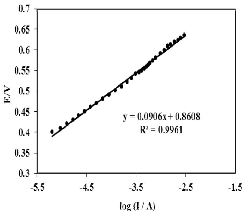
**Fig. 7.** Tafel plot derived from the rising part of voltammogram recorded at a scan rate  $5 \text{ mV s}^{-1}$
