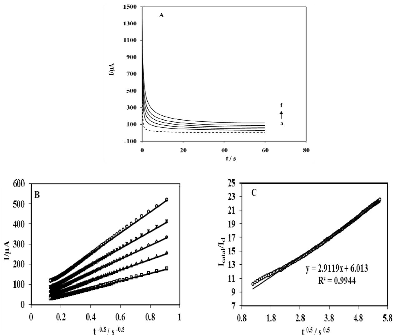
**Fig. 10.** (A) Chronoamperograms of Ni-Al LDH/MCP electrode in 0.1 M NaOH containing different concentrations of methanol: 0.0, 0.01, 0.02, 0.03, 0.04 and 0.05 mol L<sup>-1</sup>, from (a) to (f), respectively. Potential steps were 0.75 and 0.0 V, respectively. (B) Dependency of transient current on  $t^{-1/2}$ . (C) Dependency of  $I_{\text{cat}}/I_d$  on  $t^{1/2}$  derived from CAs of (a) and (f) in panel (A)
