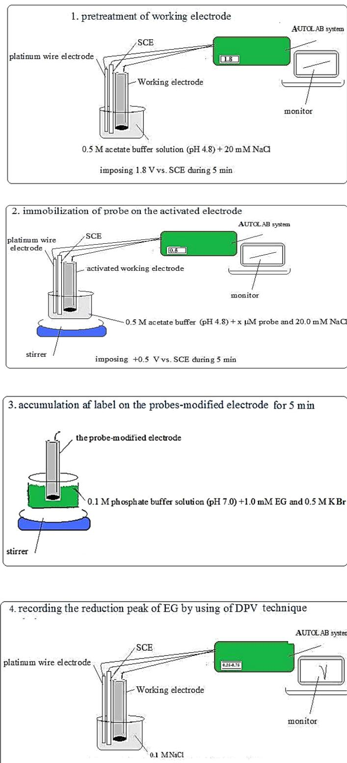
**Scheme 2.** The general scheme of all electrode modification before the measurements
