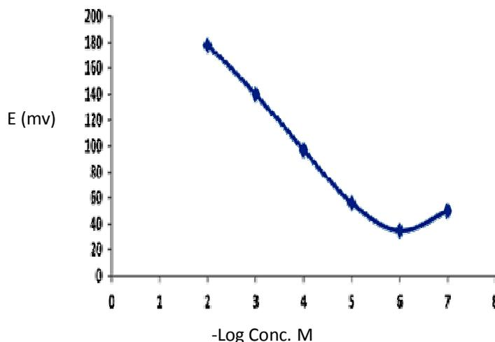
**Fig. 2.** Profile of the potential in mV vs.  $-\log$  concentration of sitagliptin phosphate obtained by using the proposed electrode
