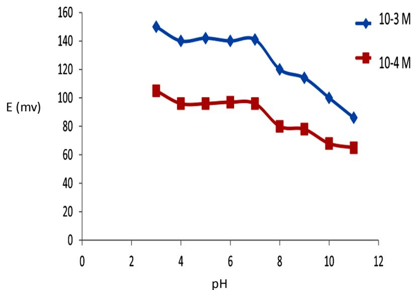
**Fig. 3.** Effect of pH on the response of the proposed electrode
