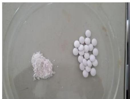
**Fig. 2.** Powder converted into tablet by tablet compressing machine
