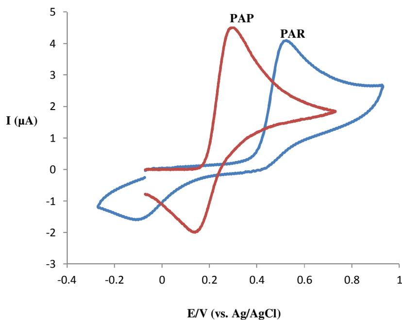
**Fig. 1.** Cyclic voltammograms of (a) PAR ( $50 \mu\text{g mL}^{-1}$ ) and (b) PAP ( $50 \mu\text{g mL}^{-1}$ ) in pH 7.0 phosphate buffer solution on GCE
