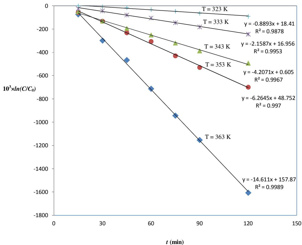
**Fig. 4.** The plot of  $\ln(C/C_0)$  vs. reaction time  $t$  for PAR hydrolysis at various temperatures of 50, 60, 70, 80 and 90°C
