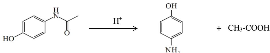
**Scheme 1.** The hydrolysis reaction of paracetamol
