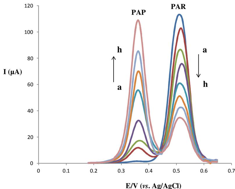
**Fig. 3.** Differential pulse voltammograms of PAR hydrolyzed solution in the hydrolysis times of (a) 0, (b) 15, (c) 30, (d) 45, (e) 60, (f) 75, (g) 90 and (h) 120 min at the reaction temperature of 80 °C. The initial concentration of PAR was 250 µg ml<sup>-1</sup>
