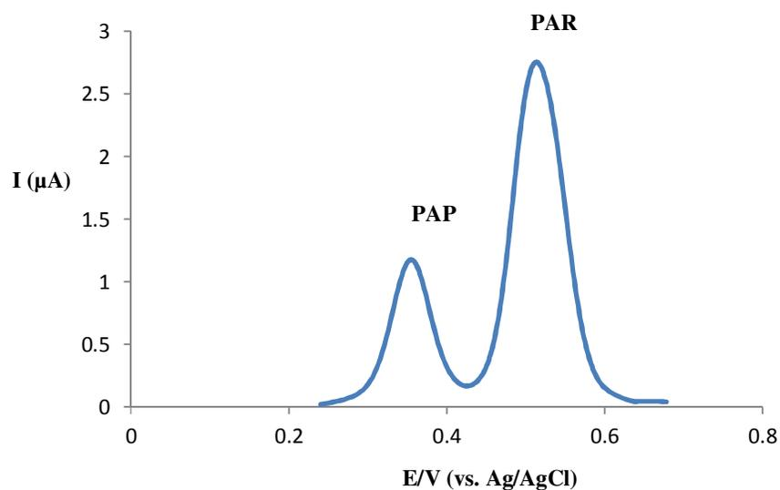
**Fig. 2.** Differential pulse voltammogram of GCE in a solution containing PAR ( $5.0 \mu\text{g mL}^{-1}$ ) and PAP ( $1.0 \mu\text{g mL}^{-1}$ ) in pH 7.0 on GCE
