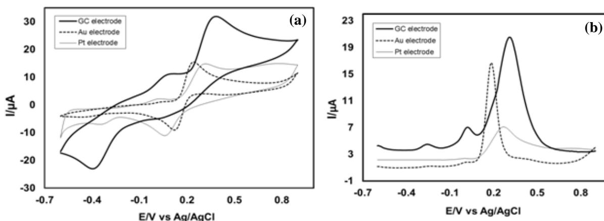
**Fig. 5.** a) Cyclic voltammogram (CV) and b) Differential pulse voltammogram (DPV) of 2 mM catechol with 70 mM aspartic acid in Gc electrode (3.0 mm), Gold electrode (1.6 mm) and Platinum electrode (1.6 mm) at pH 7 and scan rate 0.1 V/s
