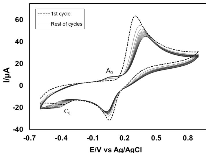
**Fig. 6.** Cyclic voltammogram of 70 mM aspartic acid with 2 mM catechol of GC (3 mm) electrode in the buffer solution of pH 7 at scan rate 0.1 V/s (15 cycles). The appeared anodic peak current ( $A_0$ ) and cathodic peak current ( $C_0$ ) increased with the iteration scan from the first cycle. First cycle marked by dashed line and the rest of the cycles by solid line
