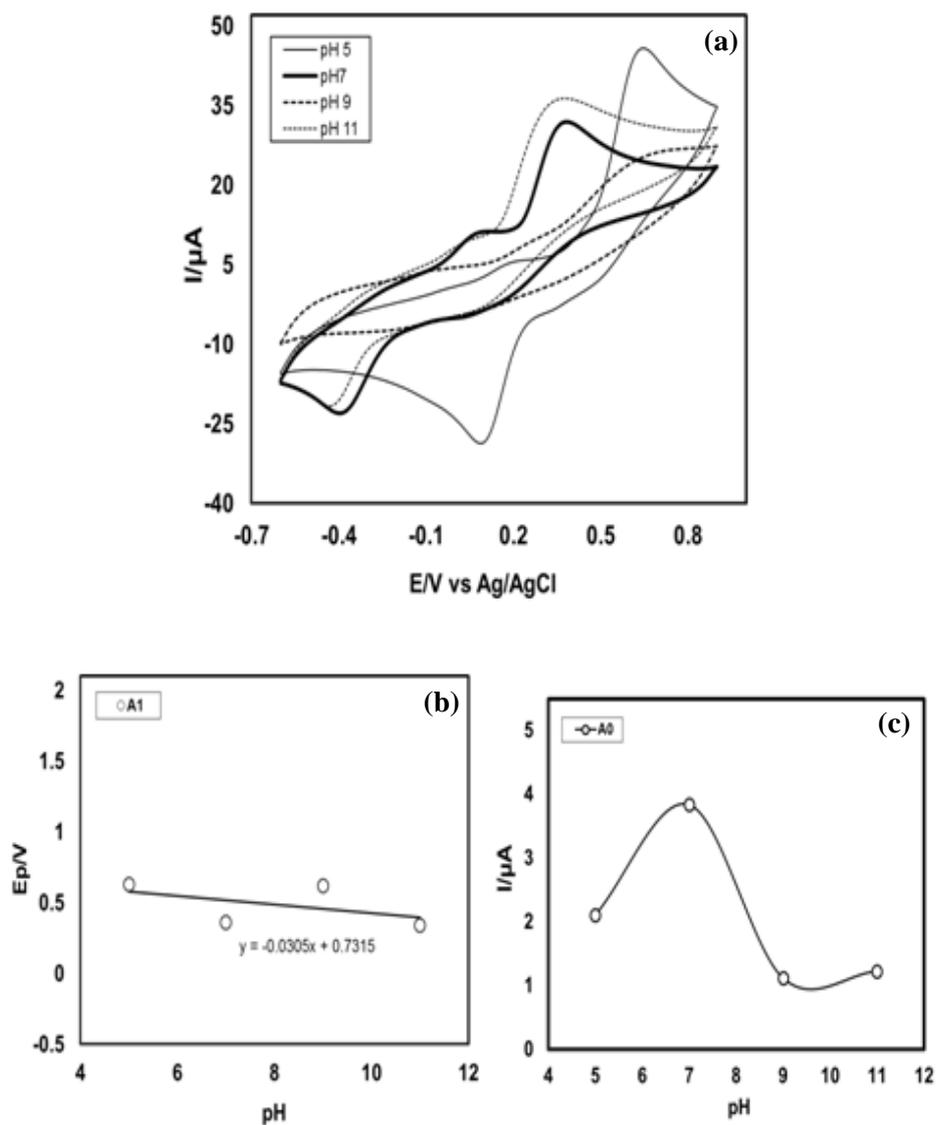
**Fig. 3.** a) Cyclic voltammogram of 2 mM catechol with 70 mM aspartic acid of GC (3 mm) electrode in different pH (5, 7, 9 and 11) at scan rate 0.1 V/s; b) Plots of peak potential vs pH in the same condition; c) Plots of peak current vs pH in the same condition. The meaning of symbol  $A_0$  and  $A_1$  is similar to Fig. 1
