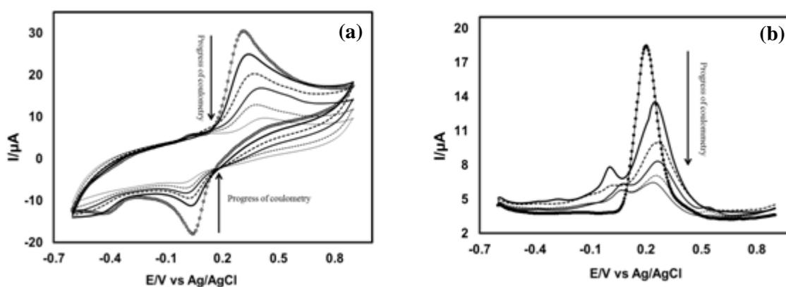
**Fig. 7.** a) Cyclic voltammogram and b) Differential pulse voltammogram (DPV) of 1mM Catechol in presence of 35 mM aspartic acid of GC electrode during controlled potential coulometry at 0.45 V in pH 7 at scan rate 0.1 V/s after consumption of 0-100 C
