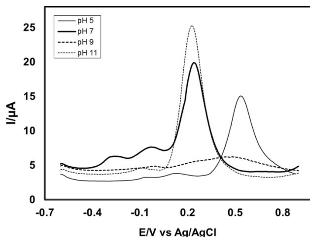
**Fig. 8.** Differential pulse voltammogram (DPV) of 2 mM catechol with 70 mM aspartic acid of GC electrode in second scan of different pH (5, 7, 9 and 11) and scan rate 0.1 V/s
