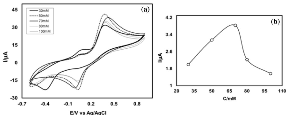
**Fig. 4.** a) CV of composition changes of aspartic acid (30, 50, 70, 80 and 100 mM) with fixed 2 mM catechol of GC electrode at pH 7 and scan rate 0.1 V/s. b) Plots of anodic peak current,  $I_p$  vs concentration of (30, 50, 70, 80 and 100 mM) aspartic acid with (fixed 2 mM catechol) in same condition. The meaning of  $A_0$  is similar to Fig. 1
