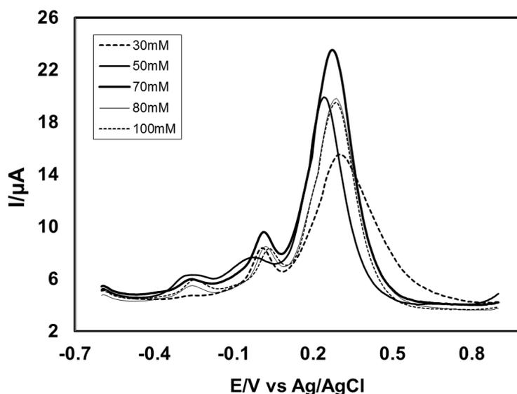
**Fig. 10.** Differential pulse voltammogram (DPV) of composition change of aspartic acid (30, 50, 70, 80 and 100 mM) with the fixed composition of 2 mM Catechol in second scan of pH 7 at  $E_{puls}$  0.02 V,  $t_{puls}$  20 ms of GC electrode and scan rate  $0.1 \text{ Vs}^{-1}$
