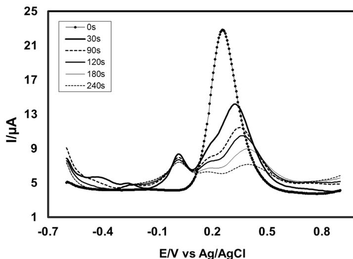
**Fig. 9.** Differential pulse voltammogram (DPV) of deposition time change (0, 10, 30, 60, 90, 120 and 240 s) of 2 mM catechol with 70 mM aspartic acid of pH7 at  $E_{puls}$  0.02 V,  $t_{puls}$  20 ms and scan rate  $0.1 \text{ V s}^{-1}$
