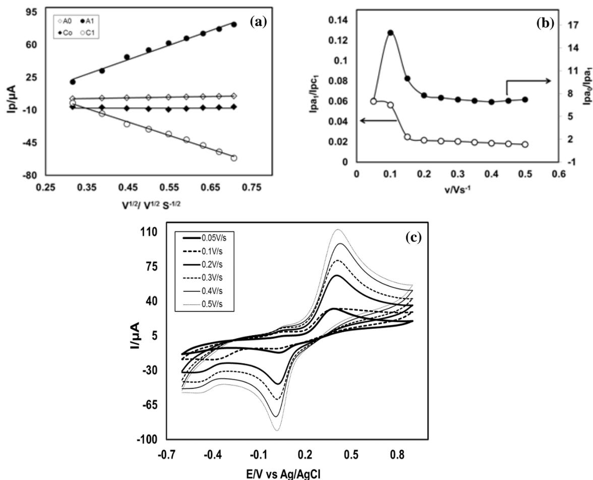
**Fig. 2.** a) Cyclic voltammogram of 2 mM catechol with 70 mM aspartic acid in the second scan of potential at Gc electrode in buffer solution (pH 7) at scan rate 0.05 V/s to 0.5 V/s; b) Plots of peak current *vs.* square root of scan rate in the same condition. Legend shows the symbol of oxidation and reduction peaks; c) Variation of peak current ratio of corresponding peak ( $I_{pa1}/I_{pc1}$ ) and anodic peak ( $I_{pa0}/I_{pa1}$ ) *vs.* scan rate in the same condition
