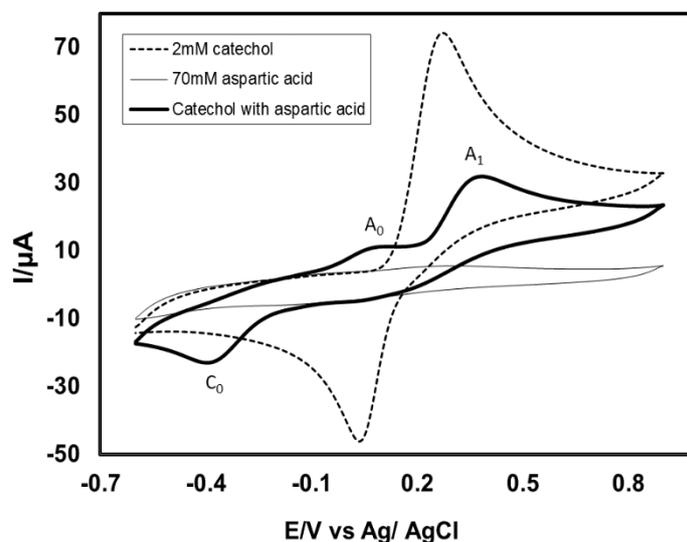
**Fig. 1.** Cyclic voltammogram of 2 mM catechol (dashed line), 70 mM aspartic acid (solid line) and 2 mM catechol with 70 mM aspartic acid (deep solid line) of GC electrode in buffer solution (pH 7) at scan rate 0.1 V/s (2nd cycle).  $A_0$  and  $A_1$  is appeared anodic peak and anodic peak,  $C_0$  is corresponding cathodic peak
