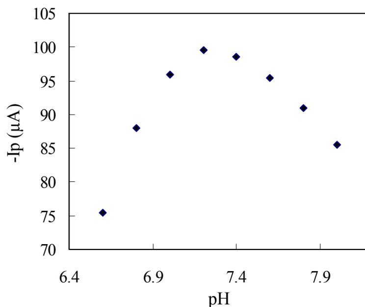
**Fig. 6.** pH dependency of KI anodic peak current at HRP-anti-HIgG/HIgG/anti-HIgG/NH<sub>2</sub>-CNTs/GC electrode. The electrode was placed in 50 mM PBS buffer containing 3 mM KI and 2 mM H<sub>2</sub>O<sub>2</sub>, HRP-anti-HIgG and HIgG (75 ng/ml). Scan rate was 50 mV/s
