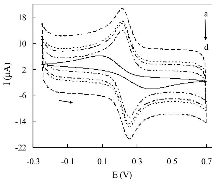
**Fig. 4.** CVs of  $[\text{Fe}(\text{CN})_6]^{2/3+}$  at different stages of GC electrode modification. Solid line shows the CV on GC electrode. The other CVs from outer to inner: (a) MWCNTs/GC, (b) anti-HIgG/ $\text{NH}_2$ -MWCNTs/GC, (c) (BSA)anti-HIgG/ $\text{NH}_2$ -MWCNTs/GC, (d) HIgG/(BSA)anti-HIgG/ $\text{NH}_2$ -MWCNTs/GC electrodes in 2.0 mM  $[\text{Fe}(\text{CN})_6]^{3/4-}$  and  $\text{KNO}_3$  solution (1 M, pH 7.2). Scan rate was  $50 \text{ mV s}^{-1}$
