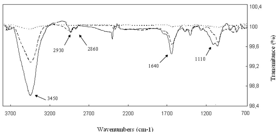
**Fig. 2.** FTIR spectra of pristine MWCNTs (dotted line), acid-functionalized MWCNTs (dashed line) and amine-functionalized MWCNTs (solid line)
