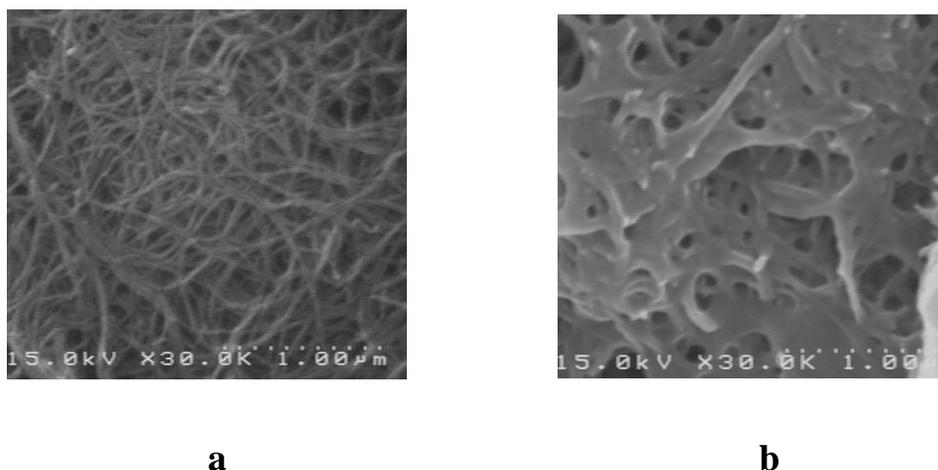
**Fig. 3.** Field emission scanning electron micrograph images of (a) NH<sub>2</sub>-MWCNTs, (b) anti-HIgG/NH<sub>2</sub>-MWCNTs. Accelerating voltage and magnification were 15 kV and ×30000, respectively
