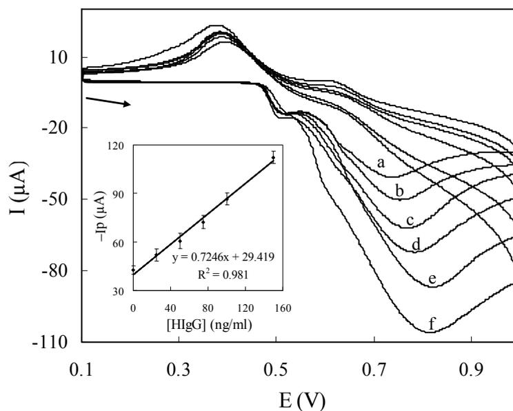
**Fig. 7.** CVs of the sandwich form modified electrode using different concentrations of HIgG: 0, 25, 50, 75, 100 and 150 ng/mL (from a to f), respectively. Inset shows the calibration curve for HIgG.  $I_p$  is the anodic peak current at 0.73 V. The experimental condition was the same as Fig. 6
