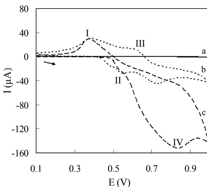
**Fig. 5.** CVs of the sandwich form of HRP-anti-HIgG/HIgG/anti-HIgG/ $\text{NH}_2$ -CNTs/GC electrode in: (a)  $\text{H}_2\text{O}_2$  (2 mM), (b) KI (3 mM), (c) mixture of  $\text{H}_2\text{O}_2$  (2 mM) and KI (3 mM). All samples prepared in 50 mM PBS (pH 7.2). Scan rate was 50 mV/s
