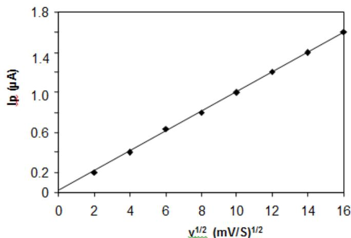
**Fig. 5.** Effect of square root of scan rate on peak current of parathion ( $0.1 \mu\text{M}$ )
