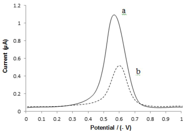
**Fig. 1.** Differential pulse adsorptive stripping voltammograms of parathion (1  $\mu\text{M}$ ) at a) SPAN/GCE and b) bare GCE
