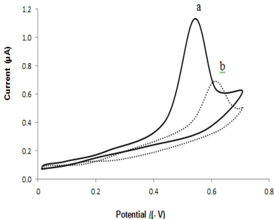
**Fig. 2.** Cyclic voltammograms of parathion (0.1  $\mu\text{M}$ ) from 0.0 V to -0.8 V at scan rate of 20  $\text{mV s}^{-1}$  at a) SPAN/GCE and b) bare GCE
