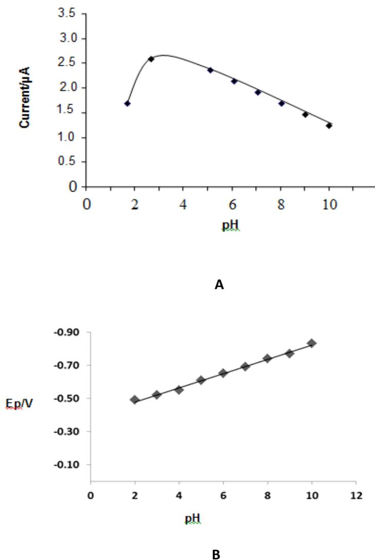
**Fig. 3. A:** Effect of pH on the peak current of parathion ( $1\mu\text{M}$ ) at SPAN/GCE; **B:** Effect of pH on the peak potential of parathion ( $1\mu\text{M}$ ) at SPAN/GCE
