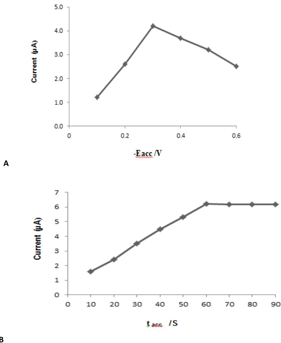
**Fig. 4. A:** Effect of accumulation potential on peak current of parathion (1  $\mu\text{M}$ ) at SPAN/GCE; **B:** Effect of accumulation time on peak current of parathion (1  $\mu\text{M}$ ) at SPAN/GCE
