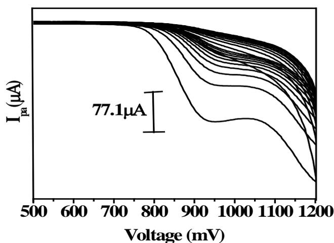
**Fig. 3.** Electropolymerisation of L-tyrosine on SnO<sub>2</sub> nanoparticles modified CPE
