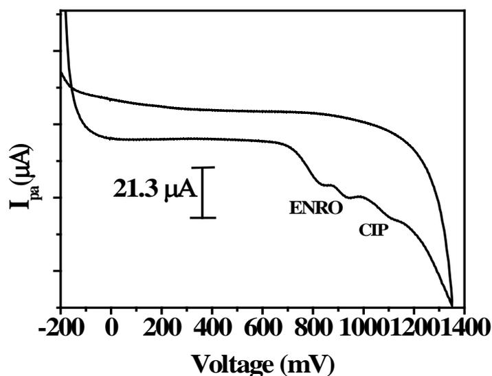
**Fig. 12.** Cyclic voltammogram obtained for oxidation of ENRO and CIP at PLTSNMCPE at scan rate of 50 mVs<sup>-1</sup>, 0.2 M PBS (pH 6.5)
