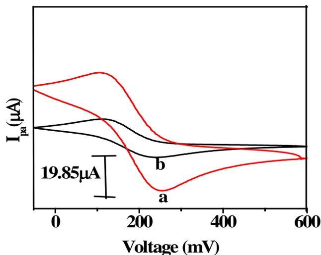
**Fig. 5.** Comparison of 0.1 mM  $K_4[Fe(CN)_6]$  in 0.1 M KCl solution at PLTSNMCPE (a) and bare CPE (b)
