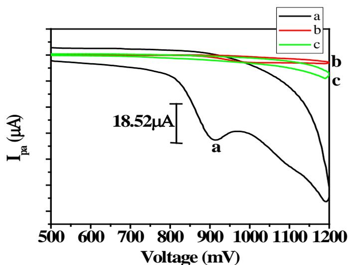
**Fig. 6.** Comparison of 0.1 mM CIP at PLTSNMCPE (a) Bare CPE (b) and Blank solution at PLTSNMCPE (c) pH 6.5, scan rate  $50 \text{ mVs}^{-1}$
