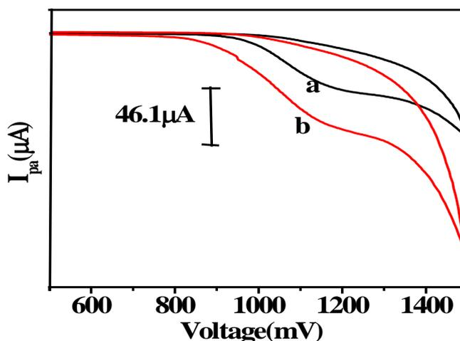
**Fig. 11.** Typical cyclic voltammograms for the determination of CIP in Ciprodac tablet sample at bare CPE (curve a) and at PLTSNMCPE (curve b) with a scan rate of  $50 \text{ mVs}^{-1}$
