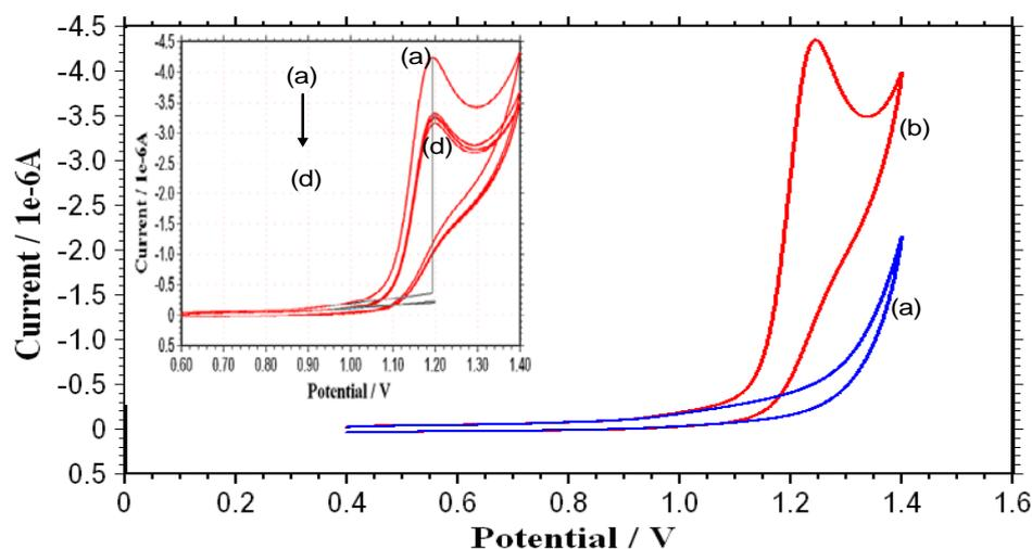
**Fig. 1.** Cyclic voltammograms of 1.0 mM PAC on carbon paste electrode, bare CPE(a); CPE+1.0 mM PAC (b); scan rate  $50 \text{ mVs}^{-1}$ ; phosphate buffer of pH 7.0 as supporting electrolyte; accumulation time: 60 s (at open circuit). Inset: Successive cyclic voltammograms obtained for 1.0 mM PAC at CPE
