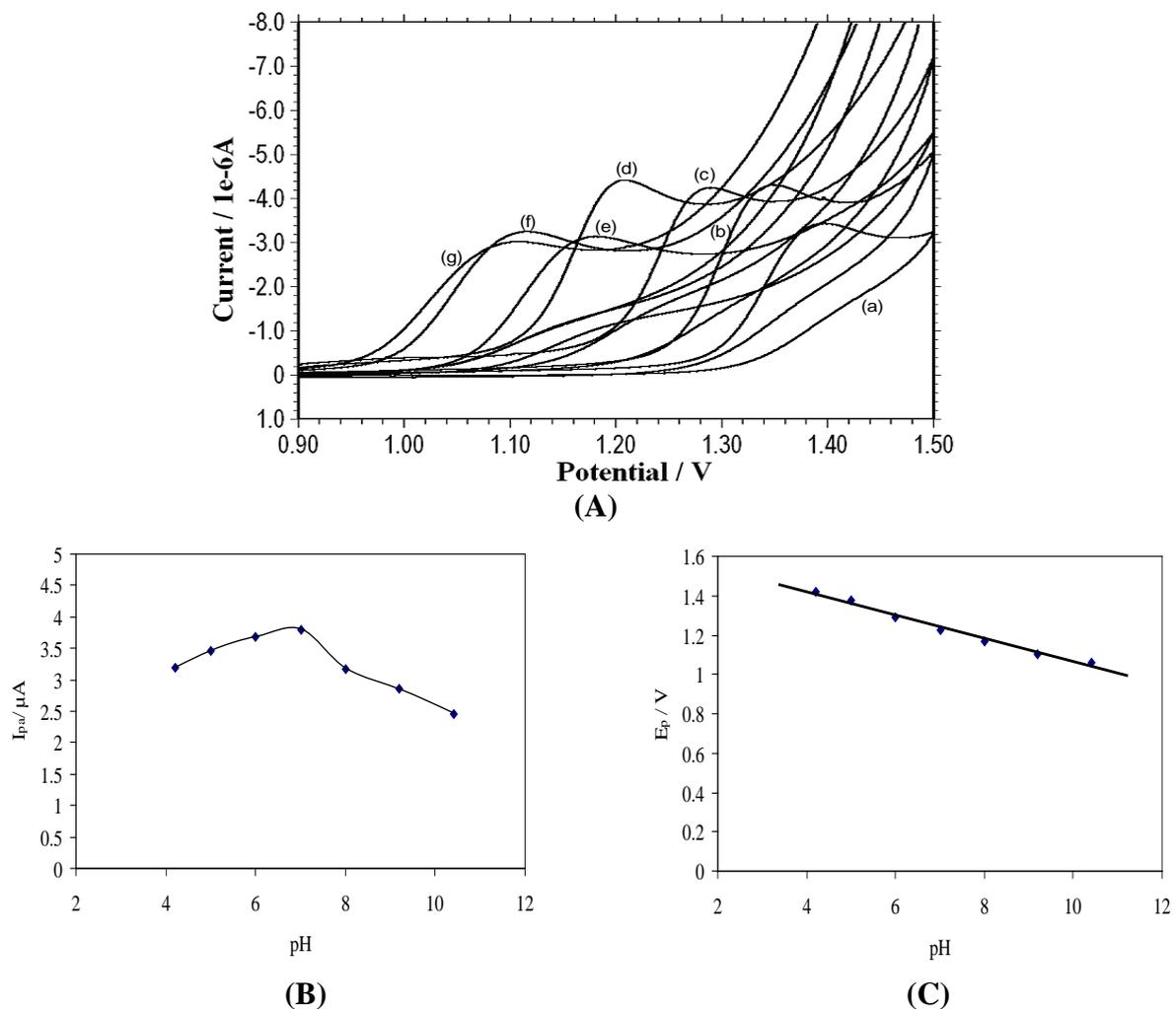
**Fig. 3.** (A) Influence of pH on the shape of the anodic peak, pH: (a) 4.2; (b) 5.0; (c) 6.0; (d) 7.0; (e) 8.0; (f) 9.2; (g) 10.4; (B) Variations of peak currents  $I_{pa}(\mu A)$  of PAC with pH. Other conditions are as in Fig. 1; (C) Influence of pH on the peak potential  $E_p$  (V) of PAC. Other conditions are as in Fig. 1
