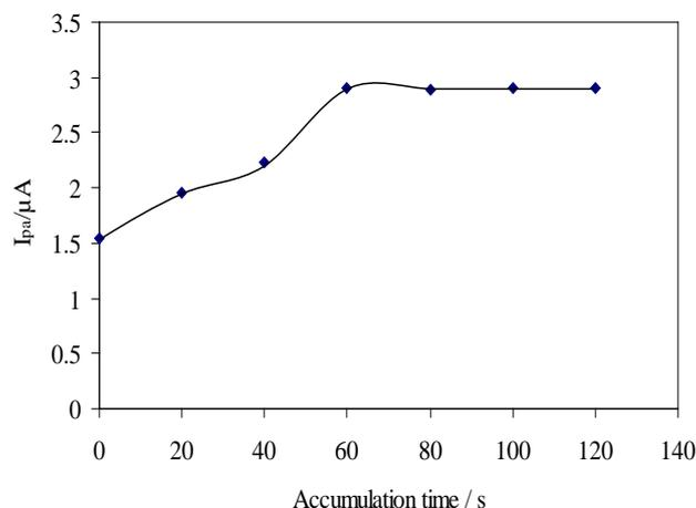
**Fig. 2.** Variation of the anodic peak current  $I_{pa}(\mu\text{A})$  with accumulation time  $t$  (s). Other conditions are as in Fig. 1
