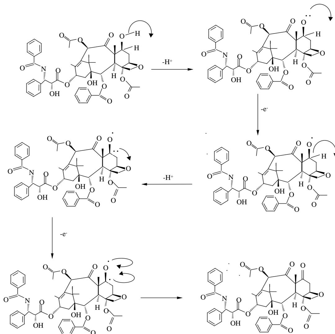
**Scheme 2.** Probable electrode oxidation mechanism of PAC
