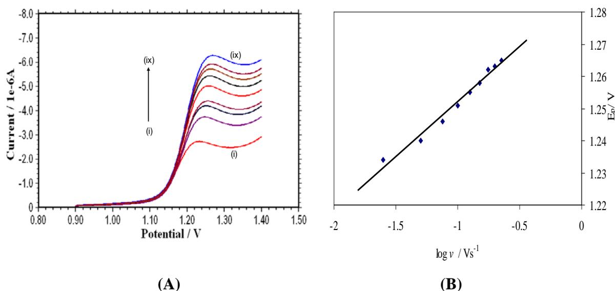
**Fig. 4.** (A) Linear sweep voltammograms for the oxidation of PAC at CPE at different scan rates (i) 0.025 (ii) 0.05 (iii) 0.075 (iv) 0.10 (v) 0.125 (vi) 0.150 (vii) 0.175 (viii) 0.2 (ix) 0.225; (B) Dependence of oxidation peak potential on the logarithm of scan rate
