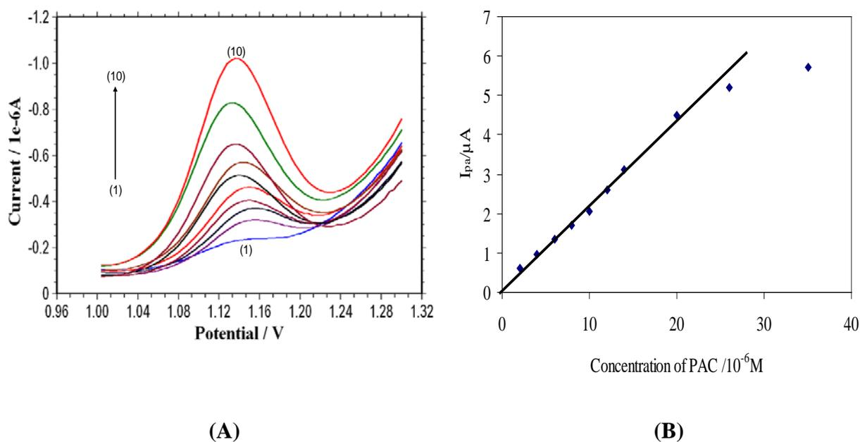
**Fig. 5.** (A) Differential pulse voltammograms for increasing concentration of PAC at CPE: (1) 2.0 (2) 4.0 (3) 6.0 (4) 8.0 (5) 10.0 (6) 12.0 (7) 14.0 (8) 20.0 (9) 26.0 (10) 35.0/ $10^{-6}$  M. other conditions are same as in Fig. 1; (B) Plot of current against the concentration of PAC
