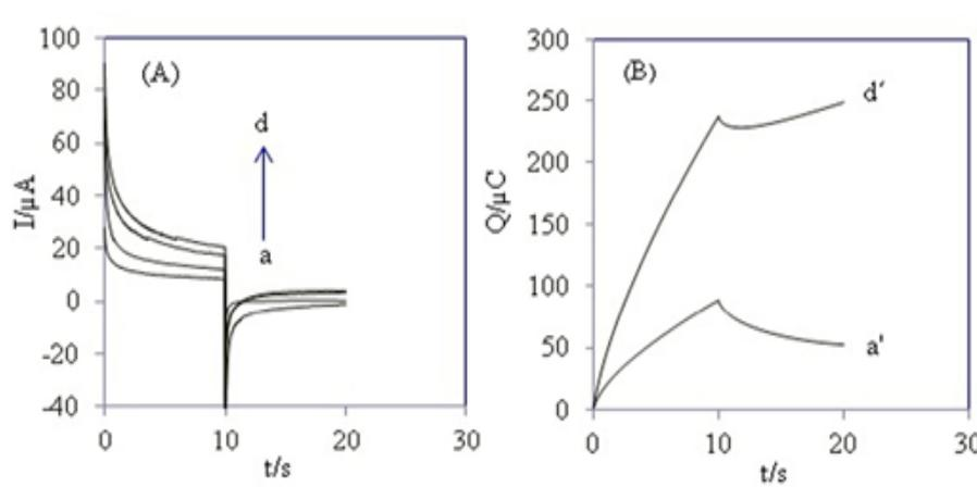
**Fig. 6.** (A) Chronoamperograms obtained for different concentration of NAC in the presence of AC in 0.1 M phosphate buffer solution (pH=7.00) with applied potential of 0.4 V and 0.2 V vs. Ag| AgCl| KCl (3M) at forward and backward step at MWCNT-CPE, respectively. The numbers a-d correspond to 0.0, 50, 250 and 300  $\mu\text{M}$  of NAC; (B) chronocolougrams of (a) and (d) of plot (A)
