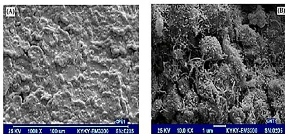
Fig. 2. SEM image of (A) CPE and (B) MWCNT/CPE
