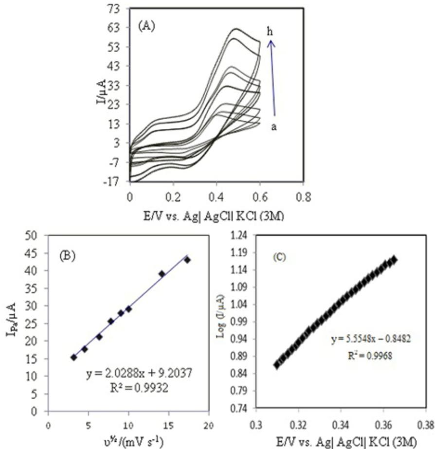
**Fig. 5.** (A) Cyclic voltammograms of NAC in the presence of AC at MWCNT-CPE in 0.1 M phosphite buffer solution (pH=7.00) at various scan rates: (a) 10, (b) 20, (c) 40, (d) 80, (e) 100, (f) 200 and (g) 300  $\text{mVs}^{-1}$ ; (B) Plot of anodic peak currents versus  $v^{1/2}$  from cyclic voltammograms of (A); (C) Variation of  $\text{Log } I$  vs. Oxidation peak potential (Tafel plot)
