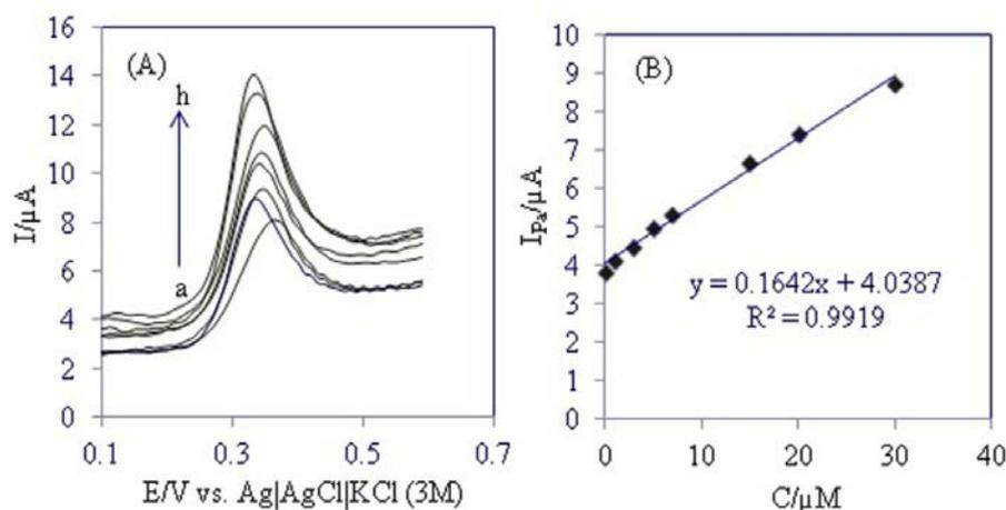
**Fig. 8.** (A) Differential pulse voltammograms of 100  $\mu\text{M}$  acetaminophen in the absence (a) and in the presence of different concentrations of NAC: (b) 1, (c) 3, (d) 5, (e) 7, (f) 15, (g) 20 and (h) 30  $\mu\text{M}$  in 0.1 M phosphate buffered solution (pH=7.00) at MWCNT-CPE; (B) The plot of peak current versus NAC concentrations
