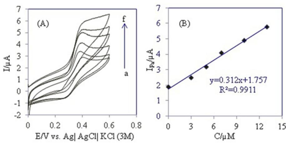
**Fig. 7.** (A) Cyclic voltammograms of 100  $\mu\text{M}$  acetaminophen in the absence (a) and presence of NAC at different concentrations: (b) 3, (c) 5, (d) 7, (e) 10 and (f) 13  $\mu\text{M}$  in 0.1 M phosphate buffer solution (pH=7.00) at a scan rate of 20  $\text{mV s}^{-1}$  at MWCNT-CPE; (B) The plot of peak currents versus NAC concentrations
