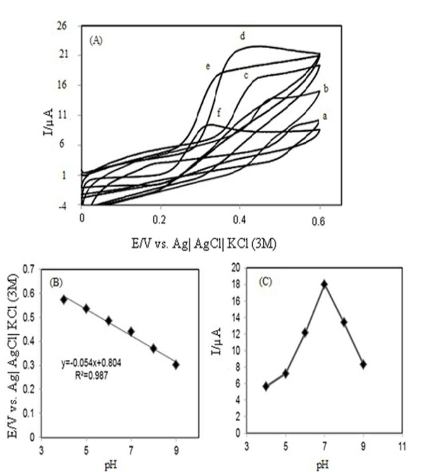
**Fig. 4.** (A) Cyclic voltammograms of 100  $\mu M$  acetaminophen in the presence of NAC in 0.1 M phosphate buffer solution at the surface of MWCNT-CPE in the various pHs: (a) 4.0, (b) 5.0, (c) 6.0, (d) 7.0, (e) 8.0 and (f) 9.0 at scan rate 20  $mV s^{-1}$ ; The variation of (B), NAC oxidation peak potentials and (C) electrooxidation peak currents of NAC versus pH values
