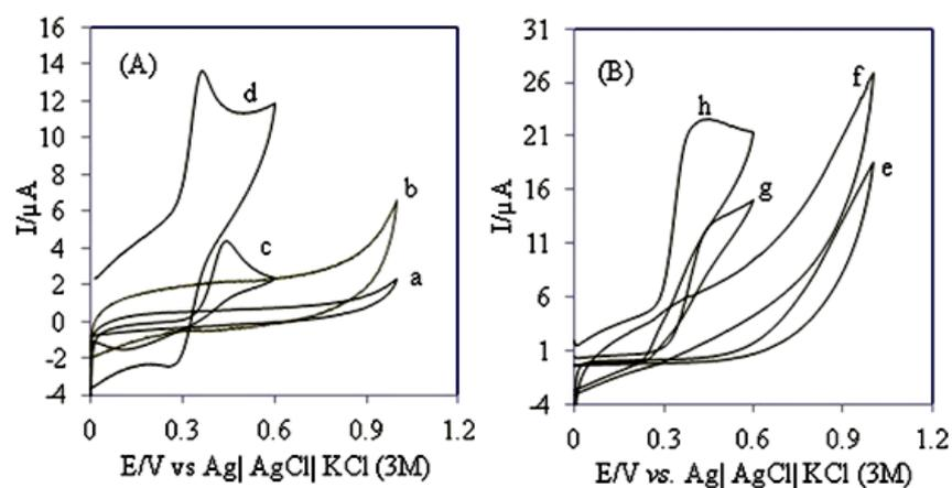
**Fig. 3.** (A) Cyclic voltammograms of (a) bare CPE, (b) MWCNT-CPE in 0.1 M PBS (pH=7.00), (c) as (a) and (d) as (b) in the presence of 100  $\mu\text{M}$  AC in 0.1 M PBS (pH=7.00); (B) Cyclic voltammograms (e) as (a) , (f) as (b) in the presence of 1000  $\mu\text{M}$  NAC, (g) as (a) and (h) as (b) in the presence of 1000  $\mu\text{M}$  NAC and 100  $\mu\text{M}$  AC in 0.1 M PBS (pH=7.00). Scan rate of potential is 20  $\text{mV s}^{-1}$
