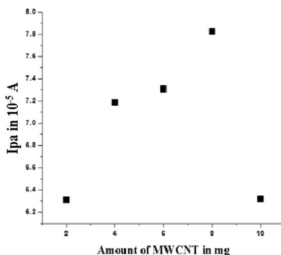
**Fig. 1.** Effect of quantity of MWCNT on anodic peak current oxidation of 0.2 mM FA in 0.2 M PBS of pH 7.4 with scan rate  $100 \text{ mVs}^{-1}$
