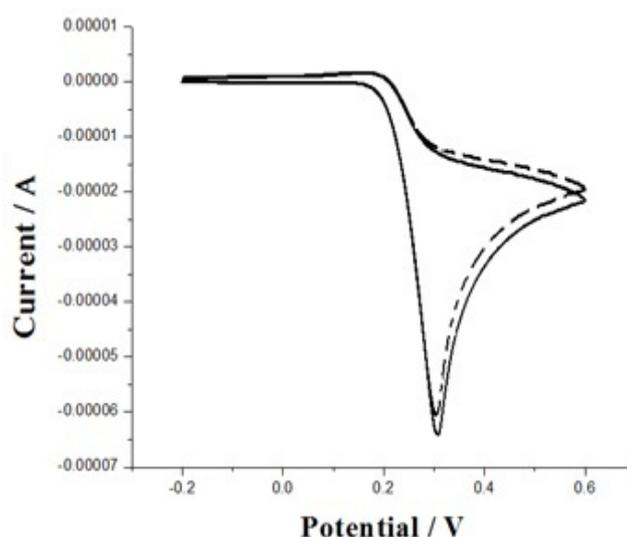
**Fig. 5.** Cyclic Voltammogram of BCPE (dotted line) and MWCNTMCPE (Solid line) in the presence of  $0.2 \text{ mM UA}$  and  $0.2 \text{ M PBS}$ , Scan rate= $100 \text{ mVs}^{-1}$
