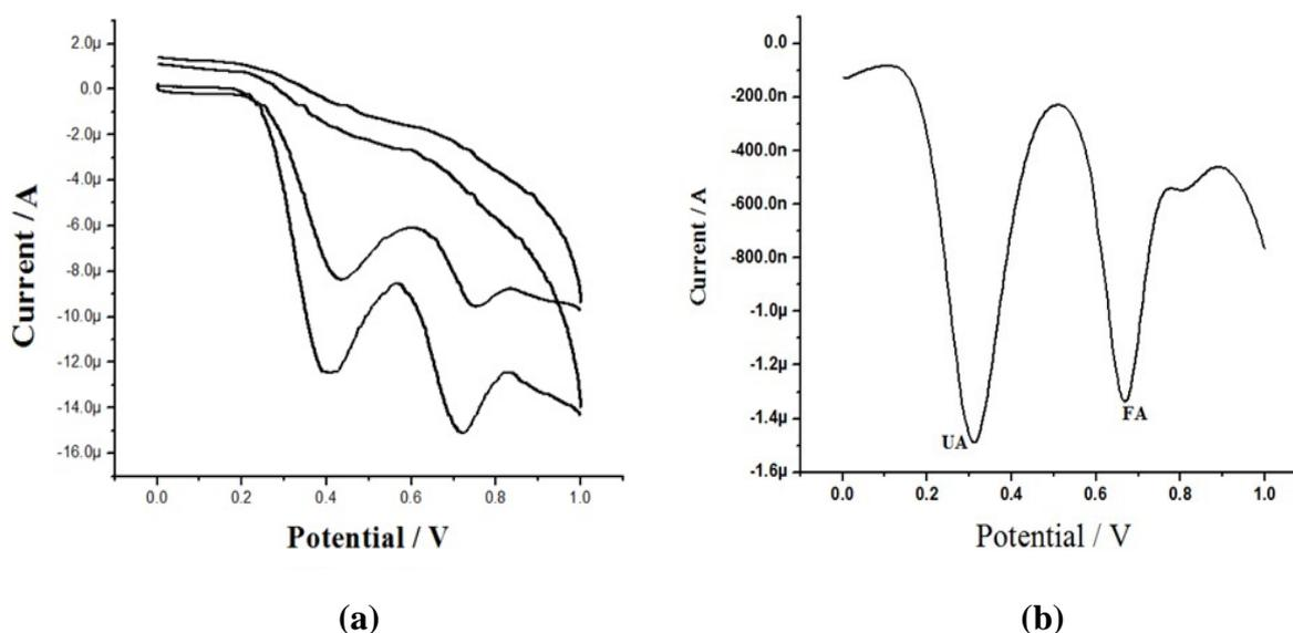
**Fig. 8.** (a) Cyclic voltammogram of 2 mM FA and 0.5 mM UA at BCPE (dotted line) and MWCNTMCPE (solid line) in 0.2 M PBS of pH 7.4 at scan rate  $50 \text{ mVs}^{-1}$ ; (b) Differential pulse voltammogram of 2 mM FA and 0.5 mM UA MWCNTMCPE in 0.2 M PBS of pH 7.4
