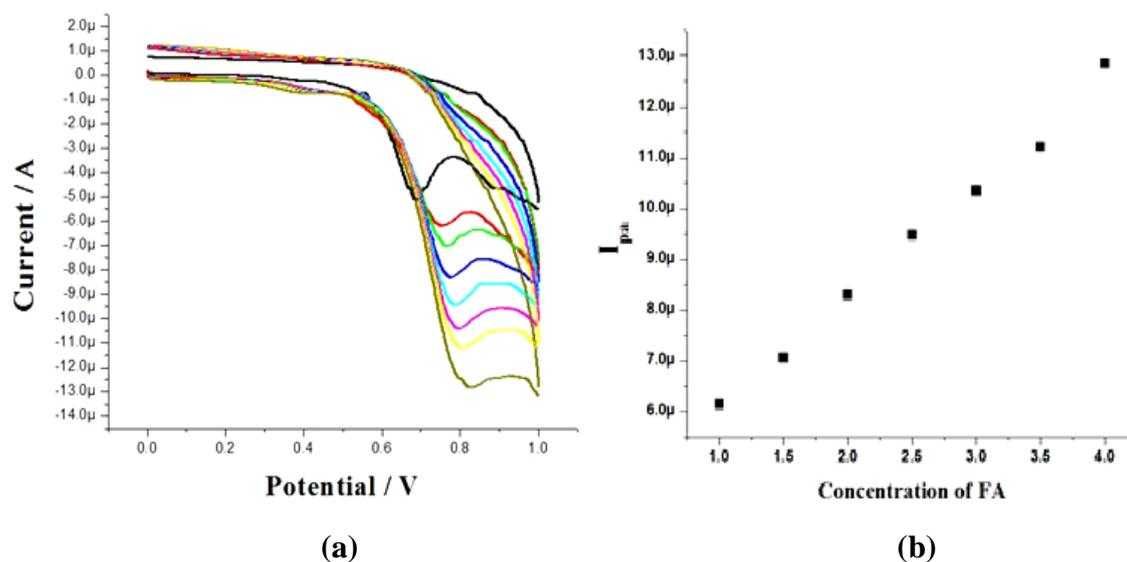
**Fig. 4.** (a) Cyclic voltammogram of variation of concentration of FA from  $1 \times 10^{-4} \text{ M}$  to  $4 \times 10^{-4} \text{ M}$  in presence of PBS of pH 7.4; (b) Effect of variation of concentration of FA versus anodic peak current
