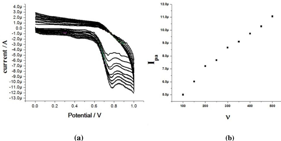
**Fig. 3.** (a) Cyclic voltammograms with different scan rate in the presence of 2 mM folic acid and 0.2 M PBS of pH 7.4, scan rate 100  $mVs^{-1}$ -500  $mVs^{-1}$ ; (b) Graph of anodic peak current versus scan rate of FA
