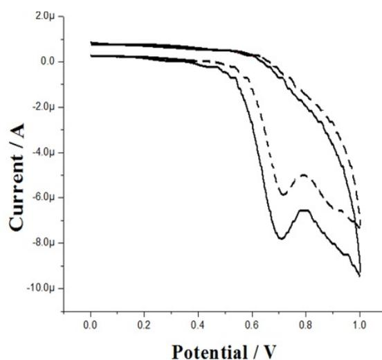
**Fig. 2.** Cyclic voltammograms of BCPE (dotted line) and MWCNTMCPE (Solid line) in the presence of 0.2 mM FA in 0.2 M PBS of pH 7.4 at the scan rate= $100 \text{ mVs}^{-1}$
