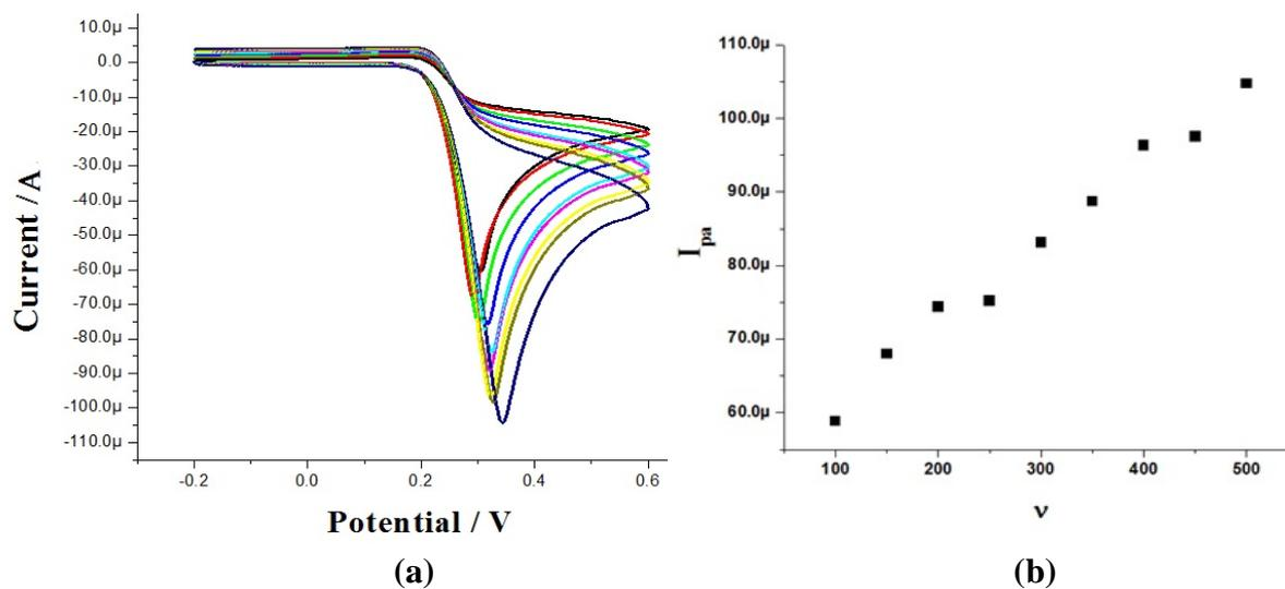
**Fig. 6.** (a) Effect of variation of scan rate on the anodic peak current of 2 mM UA in 0.2 M PBS of pH 7.4; (b) Graph of anodic peak current versus scan rate of UA
