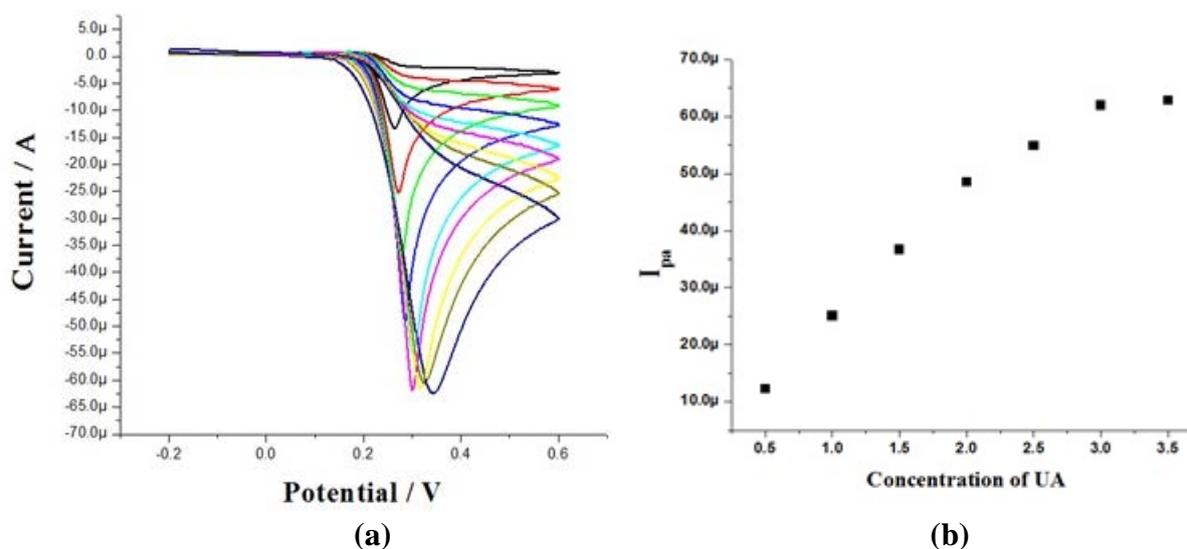
**Fig. 7.** (a) Cyclic voltammograms of variation of concentration of UA from  $0.5 \times 10^{-4}$  M to  $4.5 \times 10^{-4}$  M in 0.2 M PBS of pH 7.4; (b) Graph of anodic peak current versus concentration of UA
