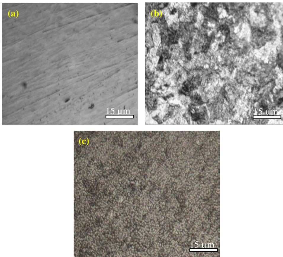
**Fig. 6.** Optical microscopy images of API 5L carbon steel, (a) before immersion, (b) after immersion (1800 s) in 0.5 M H<sub>2</sub>SO<sub>4</sub>, and (c) after immersion (1800 s) in 0.5 M H<sub>2</sub>SO<sub>4</sub>+12 g/L Thyme leaves extract
