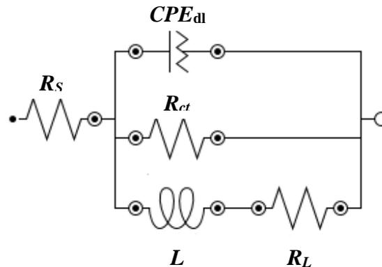
**Fig. 3.** The best equivalent circuit used to model the experimental EIS data of API 5 L carbon steel in 0.5 M H<sub>2</sub>SO<sub>4</sub> in the absence and presence of different concentration of Thyme
