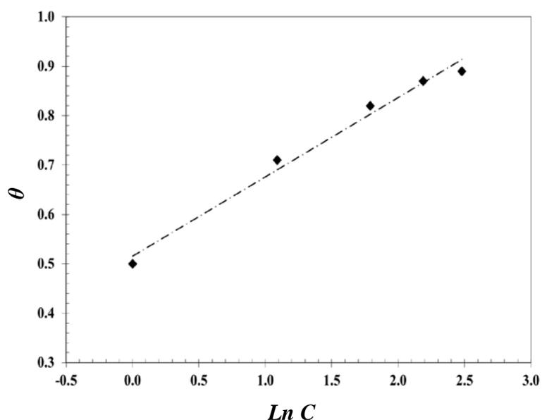
**Fig. 5.** Temkin Langmuir adsorption isotherm for API 5L carbon steel in the absence and presence of Thyme leaves extract in 0.5 M H<sub>2</sub>SO<sub>4</sub>
