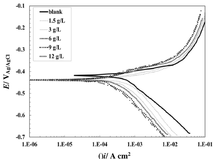
**Fig. 1.** Tafel polarization curves of API 5L carbon steel in 0.5 M H<sub>2</sub>SO<sub>4</sub> in the absence and presence of different concentration of Thyme leaves extract.
