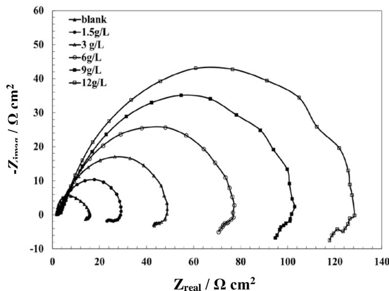
**Fig. 2.** Nyquist plots of API 5L carbon steel in 0.5 M H<sub>2</sub>SO<sub>4</sub> in the absence and presence of different concentration of Thyme leaves extract
