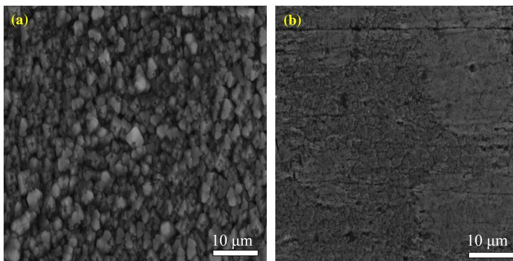
**Fig. 7.** Scanning electron microscope images of API 5L carbon steel, (a) after immersion (1800 s) in 0.5 M H<sub>2</sub>SO<sub>4</sub>, and (b) after immersion (1800 s) in 0.5 M H<sub>2</sub>SO<sub>4</sub> + 12 g/L Thyme leaves extract
