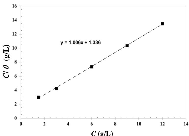
**Fig. 4.** Langmuir adsorption isotherm for API 5L carbon steel in the absence and presence of Thyme leaves extract in 0.5 M H<sub>2</sub>SO<sub>4</sub>
