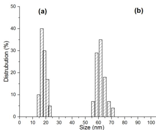
**Fig. 5.** Particle size distributions of (a) bare and (b) PVP/PVC coated Fe<sub>3</sub>O<sub>4</sub> nanoparticles
