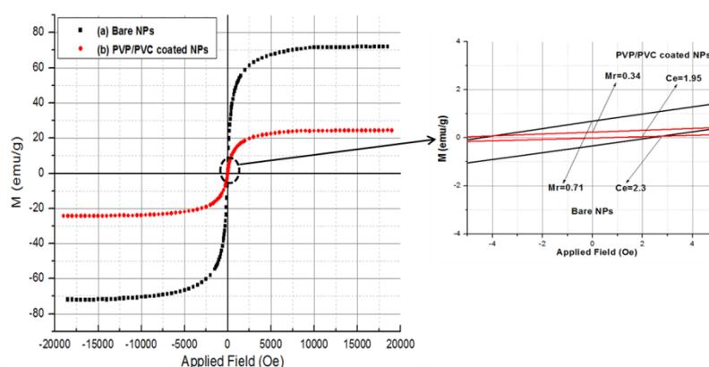
**Fig. 6.** VSM curves for the prepared (a) bare and (b) PVP/PVC coated Fe<sub>3</sub>O<sub>4</sub> nanoparticles
