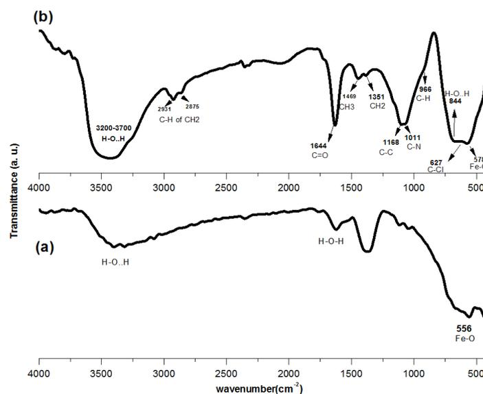
**Fig. 2.** FT-IR spectra of the prepared (a) bare and (b) PVP/PVC coated Fe<sub>3</sub>O<sub>4</sub> nanoparticles
