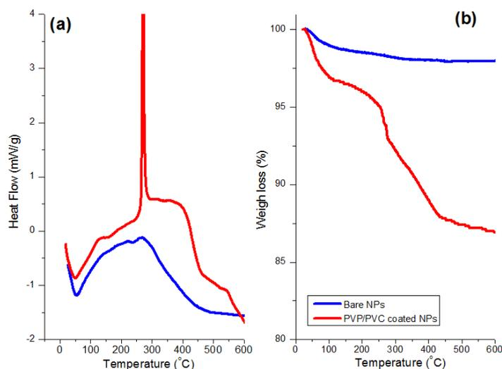
**Fig. 4.** DSC-TG curves for the prepared (a) bare and (b) PVP/PVC coated Fe<sub>3</sub>O<sub>4</sub> nanoparticles
