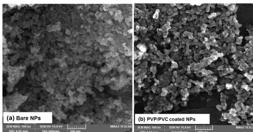
**Fig. 3.** FE-SEM images of the prepared (a) bare and (b) PVP/PVC coated  $\text{Fe}_3\text{O}_4$  nanoparticles
