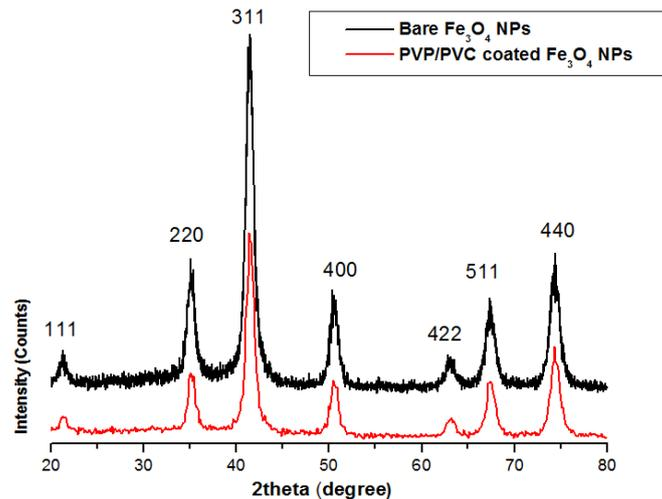
**Fig. 1.** XRD patterns of the prepared (a) bare and (b) PVP/PVC coated Fe<sub>3</sub>O<sub>4</sub> nanoparticles
