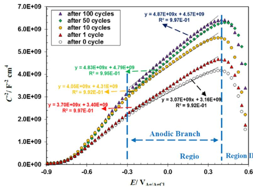
**Fig. 9.** Mott–Schottky plots of mild carbon reinforcing steel samples obtained after different numbers of cycles
