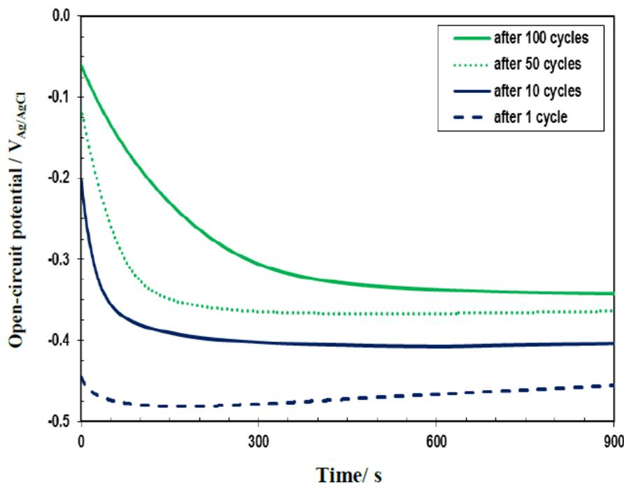
**Fig. 4.** The OCP curves after different cycles for mild carbon reinforcing steel samples
