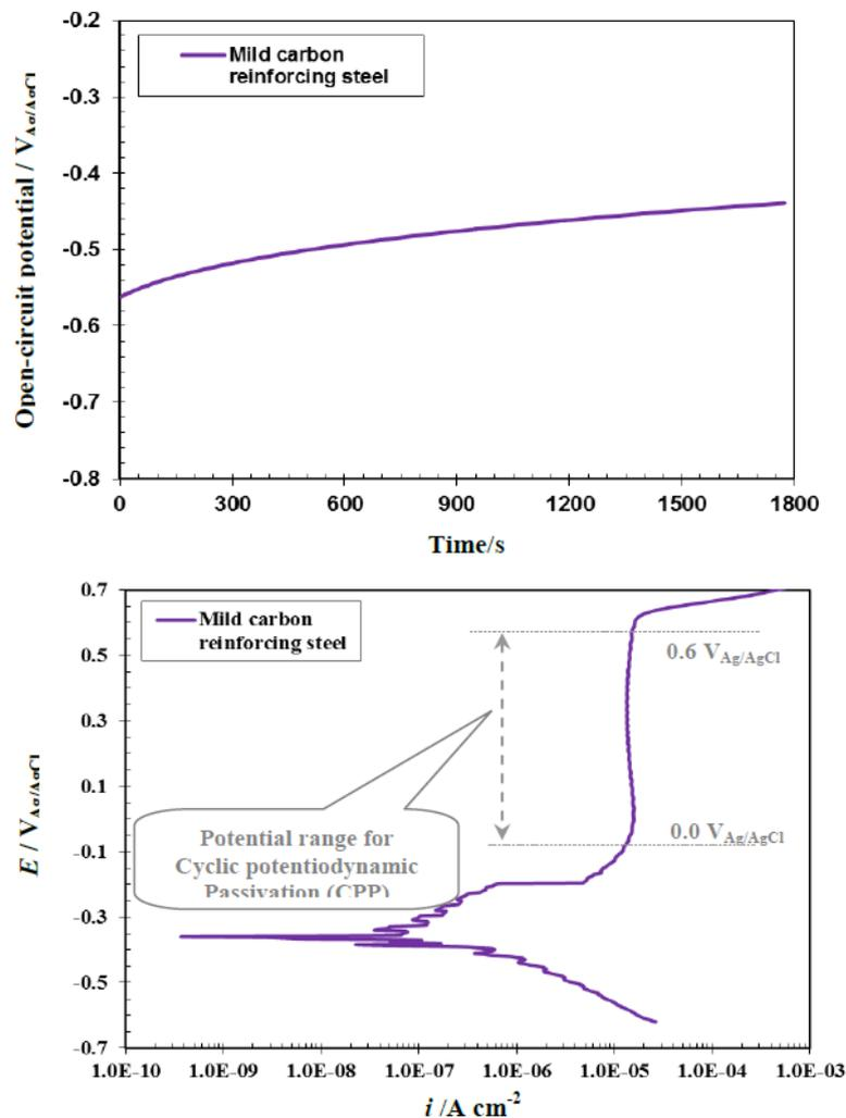
**Fig. 2.** (a) The OCP and (b) potentiodynamic polarization curves of mild carbon reinforcing steel sample in the alkaline media simulating the concrete pore (0.1 M NaOH+0.1 M KOH) solution (scan rate = 1 mVs<sup>-1</sup>)
