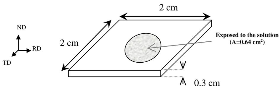
**Fig. 1.** The schematic illustration of the working electrode together with the location of the exposed area of the surface
