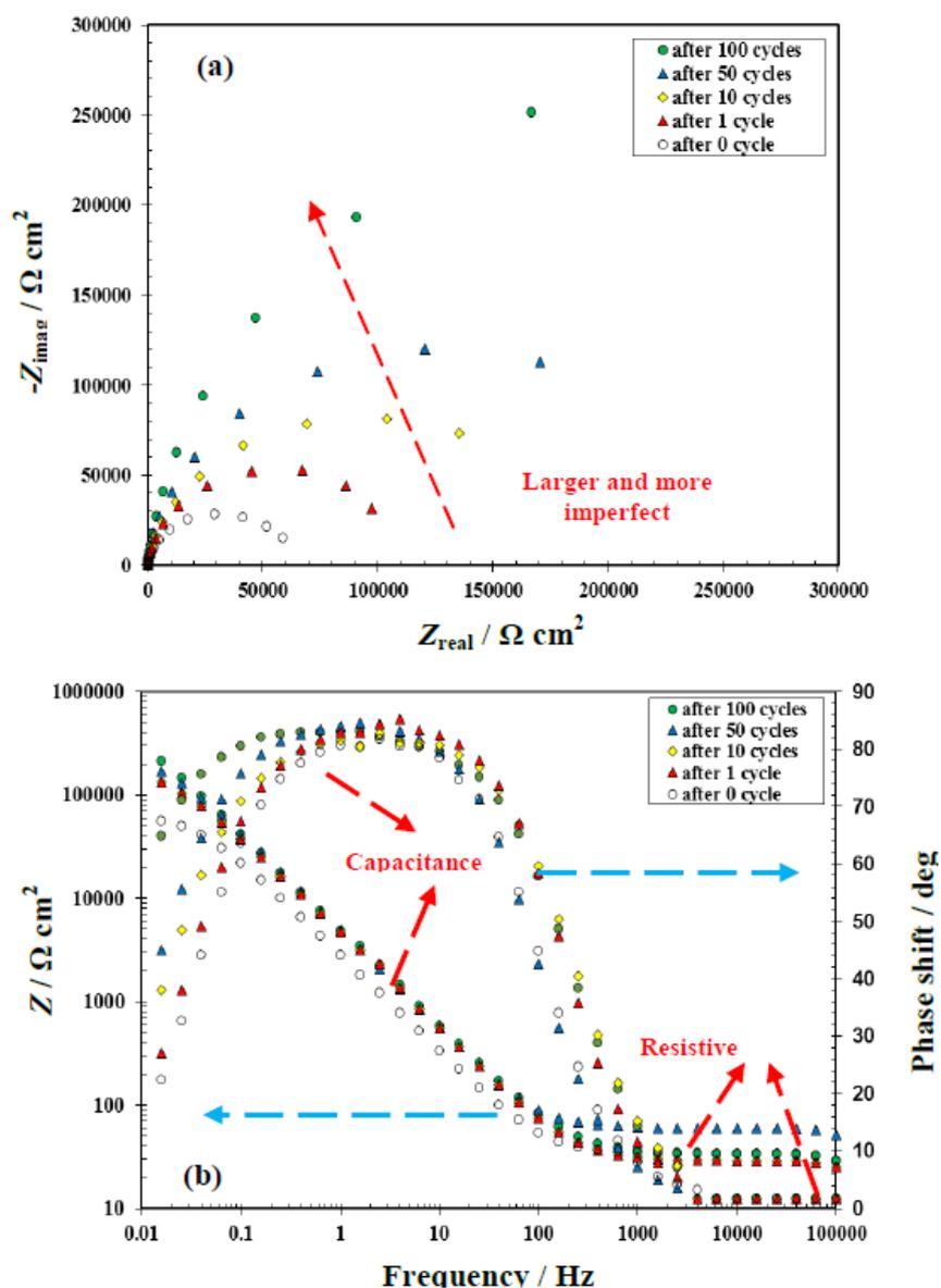
**Fig. 5.** (a) Nyquist and (b) Bode plots of mild carbon reinforcing steel samples obtained after a different number of cycles
