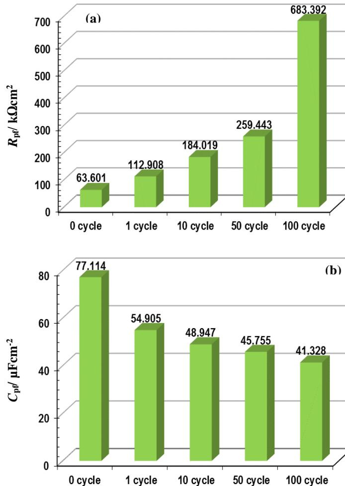
**Fig. 8.** Variations in the (a) passive film resistance and (b) double layer capacitance of mild carbon reinforcing steel samples
