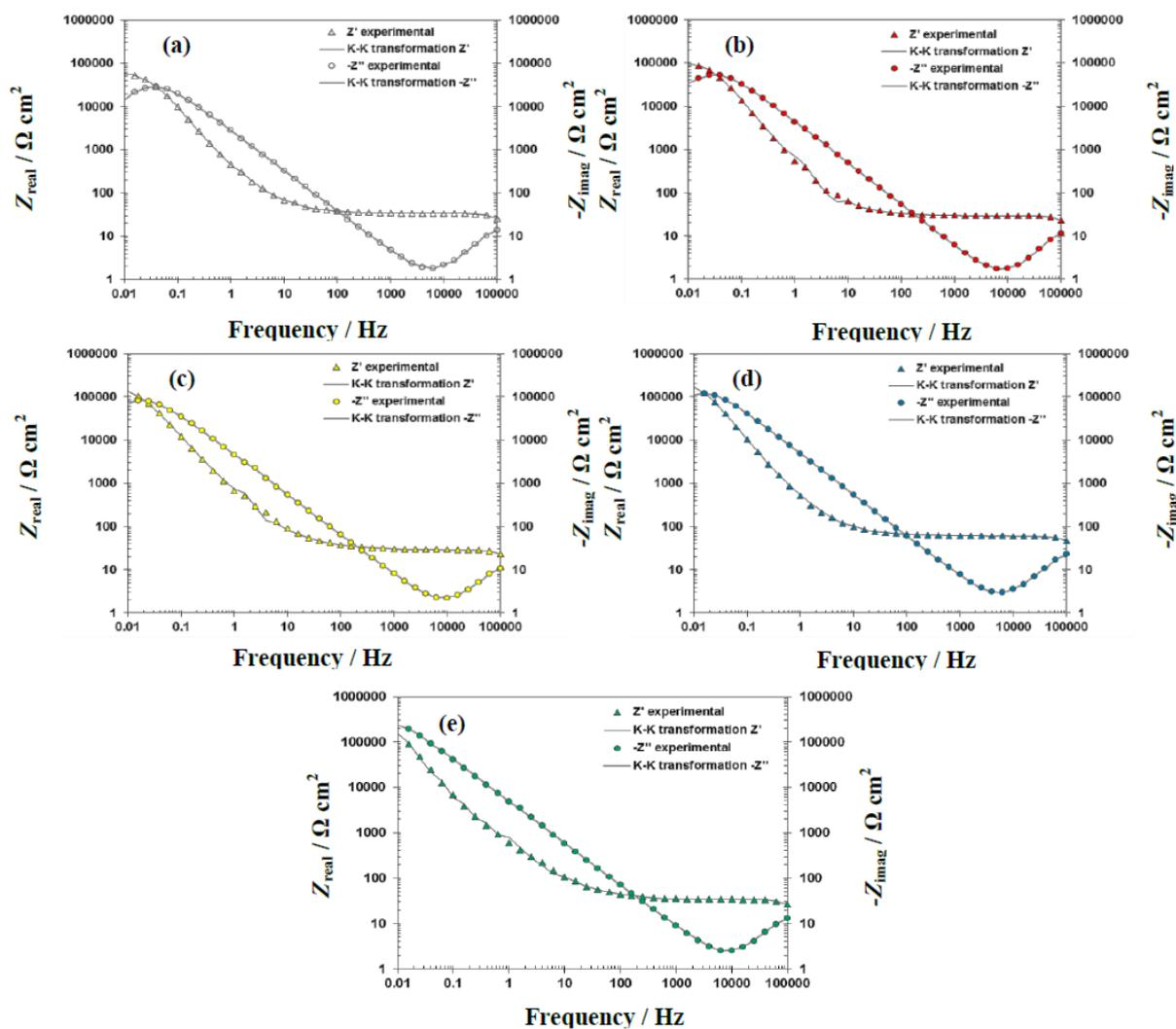
**Fig. 6.** Kramers–Kronig plots of mild carbon reinforcing steel samples obtained after different numbers of cycles, (a) 0 cycle, (b) 1 cycle, (c) 10 cycles, (d) 50 cycles, and (e) 100 cycles
