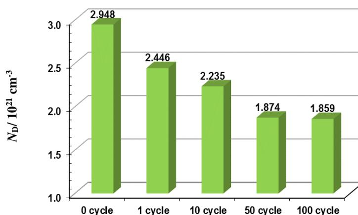
**Fig. 10.** Variations in the donor densities of mild carbon reinforcing steel samples in the alkaline media simulating the concrete pore solution
