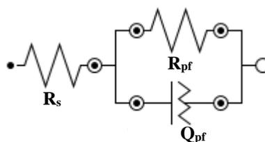
**Fig. 7.** The best equivalent circuit used for modeling of the EIS spectrum
