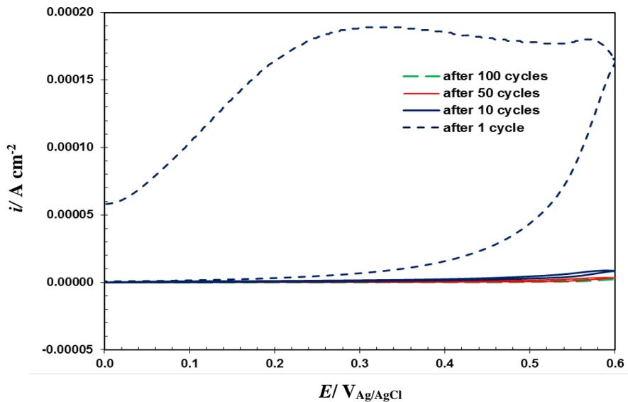
**Fig. 3.** The comparison of CPP plots of mild carbon reinforcing steel samples in the alkaline media simulating the concrete pore solution for a different number of cycles
