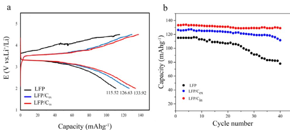
**Fig. 3.** (a) Initial charge-discharge profiles at 0.1 C current rates; (b) Cycling performance LFP, LFP/C<sub>ex</sub> and LFP/C<sub>in</sub> by the Li foil as reference and counter electrode and between 2.5-4.2 V (vs. Li/Li<sup>+</sup>)
