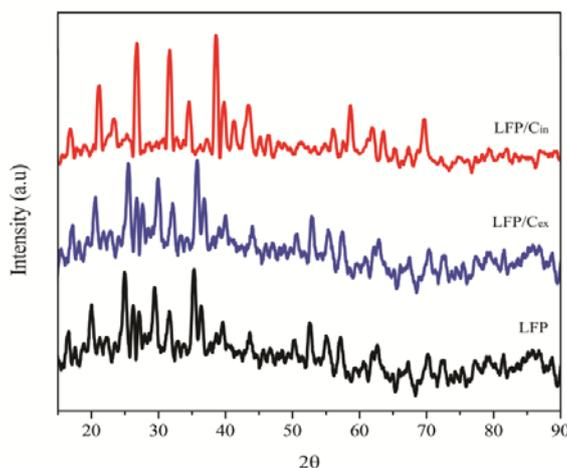
**Fig. 1.** XRD pattern of the as-prepared  $\text{LiFePO}_4$ ,  $\text{LiFePO}_4/\text{C}_{\text{ex}}$ ,  $\text{LiFePO}_4/\text{C}_{\text{in}}$  powders
