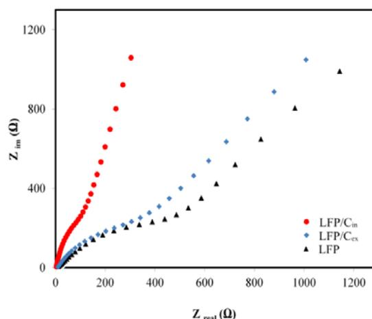
**Fig. 5.** EIS profiles of LFP/ $C_{in}$ , LFP/ $C_{ex}$  and LFP electrode
