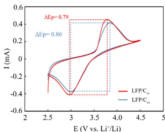
**Fig. 4.** Cyclic voltammograms (CVs) of LFP/C<sub>in</sub> and LFP/C<sub>ex</sub> electrode at scan rate of  $0.5 \text{ mV}\cdot\text{s}^{-1}$
