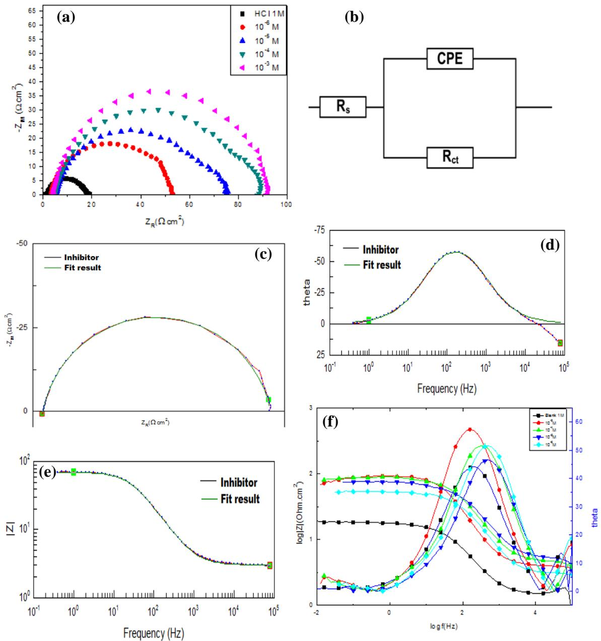
**Fig. 4.** (a) Nyquist plots recorded for mild steel in 1.0 M HCl solutions without and with different concentrations of inhibitor; (b) Equivalent circuit used to simulate the EIS diagram; (c) Fitted Nyquist plot and Bode plot for PZ-1; (d) Fitted phase angle plot; (e) Fitted Bode plot; (f) Bode ( $\log f$  vs.  $\log|Z|$ ) and phase angle ( $\log f$  vs. theta) plots of impedance spectra for mild steel in 1 M HCl in absence and presence of different concentration of inhibitor
