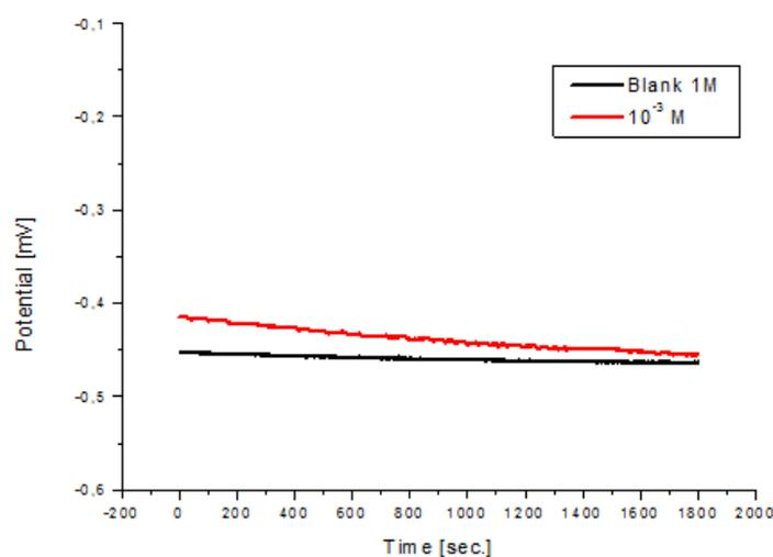
**Fig. 2.** OCP vs. time measurements in absence and presence of optimum concentration of inhibitor
