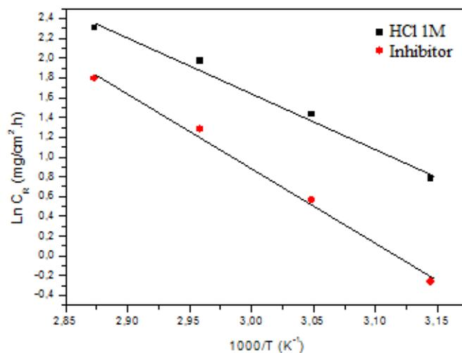
**Fig. 6.** Arrhenius plots of  $\ln C_R$  vs.  $1/T$  for steel in 1.0 M HCl in the absence and the presence of at optimum concentration of inhibitor
