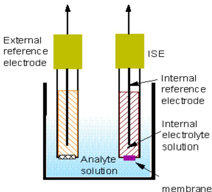
**Fig. 2.** The potentiometric cell used for the determination of sumatriptan using the proposed ion selective electrode method
