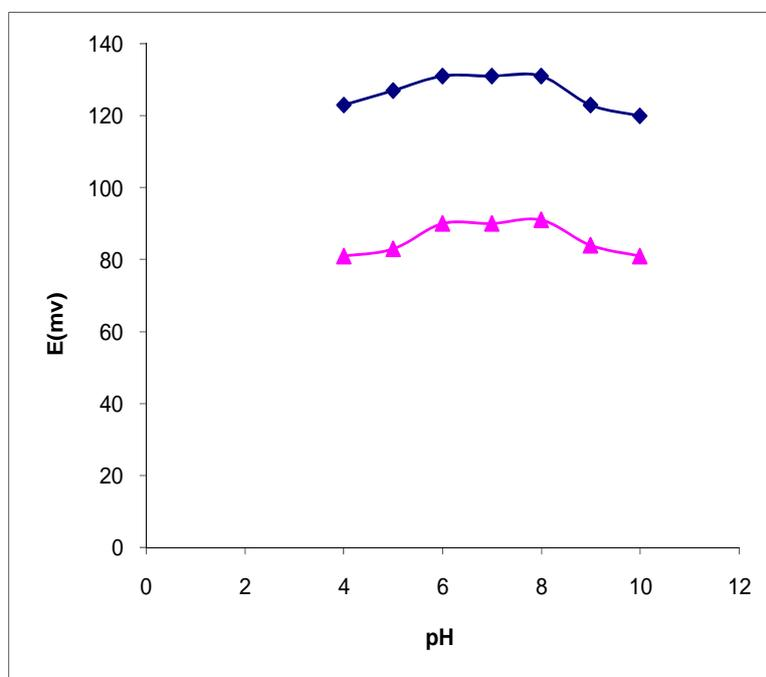
**Fig. 3.** Effect of pH on the response of proposed electrode
