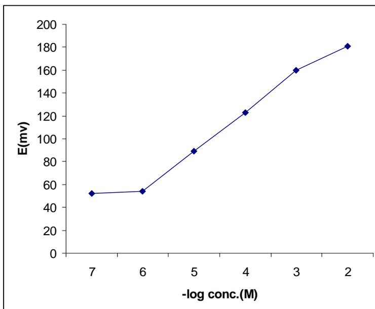
**Fig. 4.** Profile of the potential in mV to -log concentration of sumatriptan using the proposed ion selective electrode method
