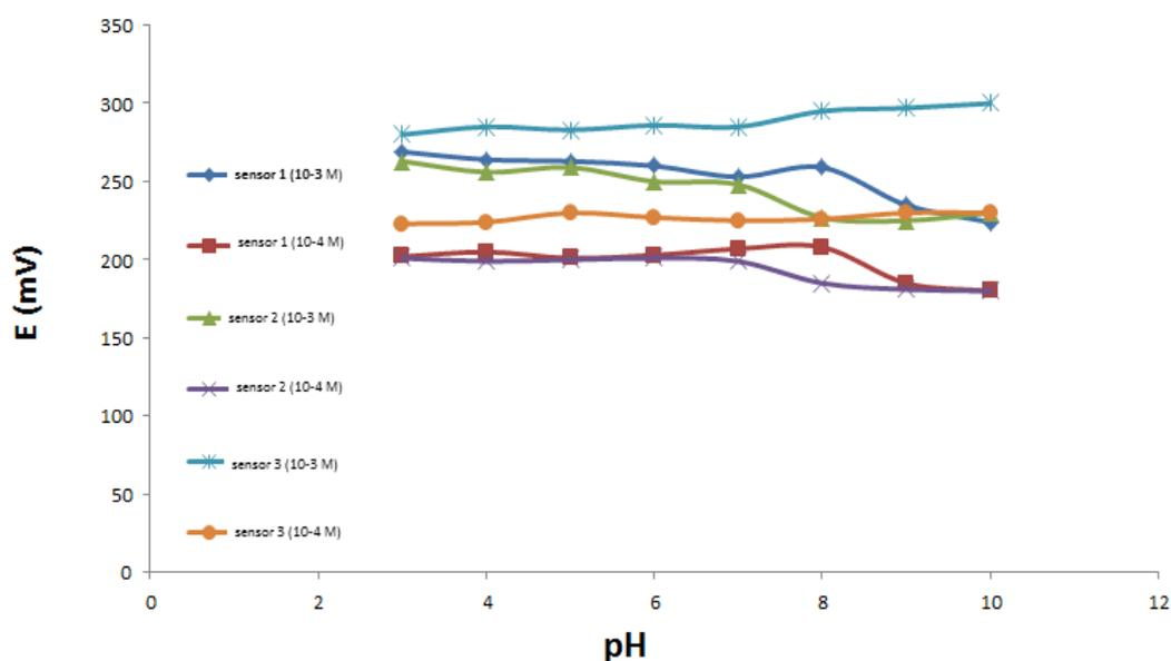
Fig. 7. Effect of pH on the response of the three sensors at  $10^{-3}$  M and  $10^{-4}$  M
