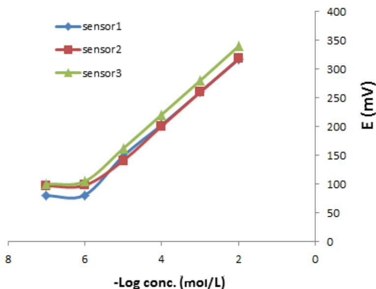
**Fig. 6.** Profile of the potential in mV versus  $-\log$  concentration of TND and CLR in M obtained by using the three proposed electrodes
