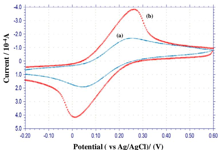
**Fig. 2.** Cyclic voltammograms for 1 mM  $K_3[Fe(CN)_6]$  at (a) bare CPE and (b) NSCPE at 50 mV/s
