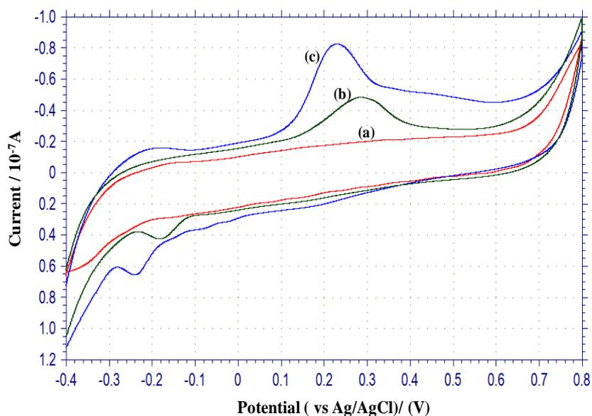
**Fig. 3.** Cyclic voltammogram for (a) 0.2 M phosphate buffer solution of pH 6.0 (without 2-TU) at NSCPE (b) 1 mM 2-TU at unmodified CPE and (c) 1 mM 2-TU at NSCPE
