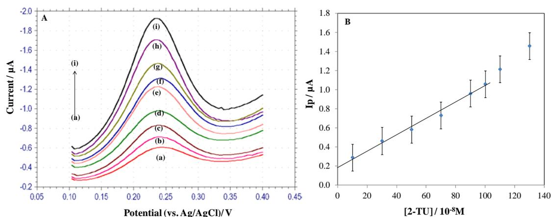
**Fig. 7.** (A) Differential pulse voltammograms at NSCPE at different concentration of 2-TU solution: (a) 10, (b) 30, (c) 50, (d) 70, (e) 90, (f) 100, (g) 110, (h) 130 and (i)  $150 \times 10^{-8}\text{M}$ ; (B) Plot of peak current against the concentration of 2-TU
