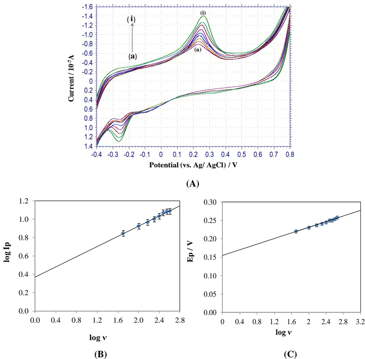
**Fig. 5.** (A) Cyclic voltammograms of 1.0 mM 2-TU in buffer solution of pH 6.0 at scan rates of (a) 50, (b) 100, (c) 150, (d) 200, (e) 250, (f) 300, (g) 350, (h) 400 and (i) 450 mV/s; (B) Relationship between logarithmic peak current and logarithmic scan rate; (C) Linear relationship between peak potential and logarithmic scan rate
