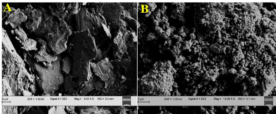
**Fig. 1.** SEM images of (A) CPE and (B) NSCPE
