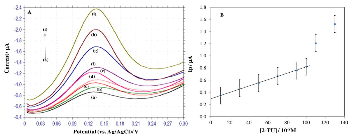
**Fig. 8.** (A) Square wave voltammograms at NSCPE at different concentration of 2-TU solution: (a) 10, (b) 30, (c) 50, (d) 70, (e) 90, (f) 100, (g) 110, (h) 130 and (i)  $150 \times 10^{-8}\text{M}$ ; (B) Plot of peak current against the concentration of 2-TU
