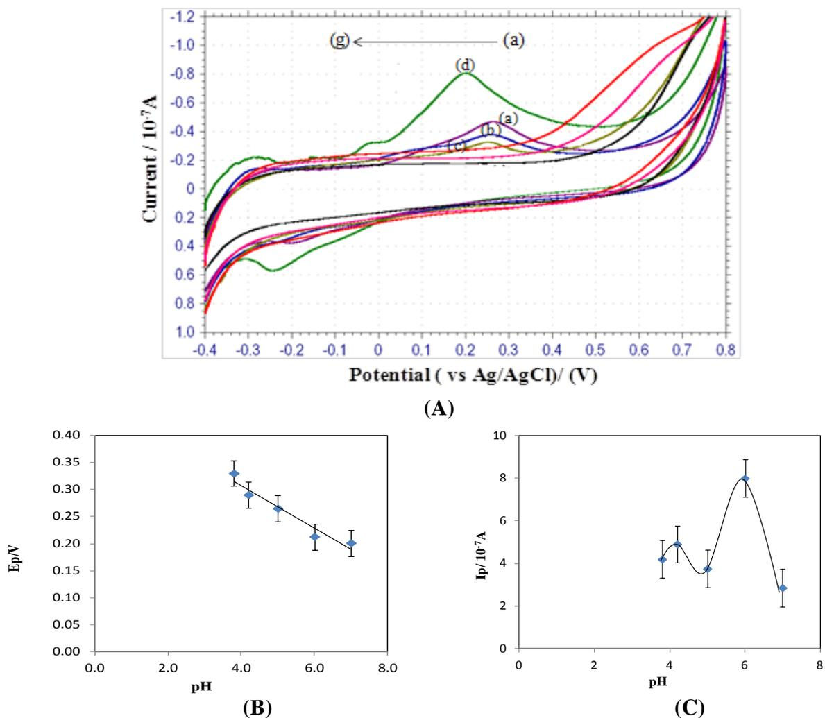
**Fig. 4.** (A) Influence of pH on the shape of the oxidation peak for 1 mM 2-TU in 0.2 M phosphate buffer solution at (a) pH 3.8, (b) pH 4.2, (c) pH 5.0, (d) pH 6.0, (e) pH 7.0, (f) pH 8.0 and (g) pH 9.2 at NSCPE, 50mV/s scan rate; (B) Variation of peak potential  $E_p$  (V) with pH for 1.0 mM 2-TU at NSCPE; (C) Variation of peak current of 1.0 mM 2-TU (at NSCPE) with pH
