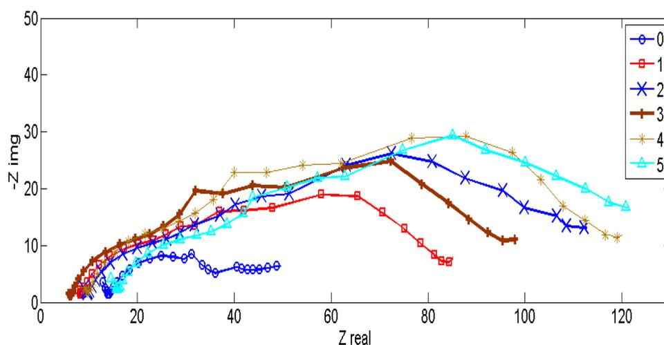
**Fig. 2.** Nyquist plots of EIS for zinc in 4 M NaOH in presence variety values of P123 0: blank, 1:75, 2:150, 3:300, and 4:450, 5:600 ppm P123
