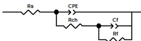
**Fig. 3.** Equivalent circuit applied for fitting of the impedance spectra
