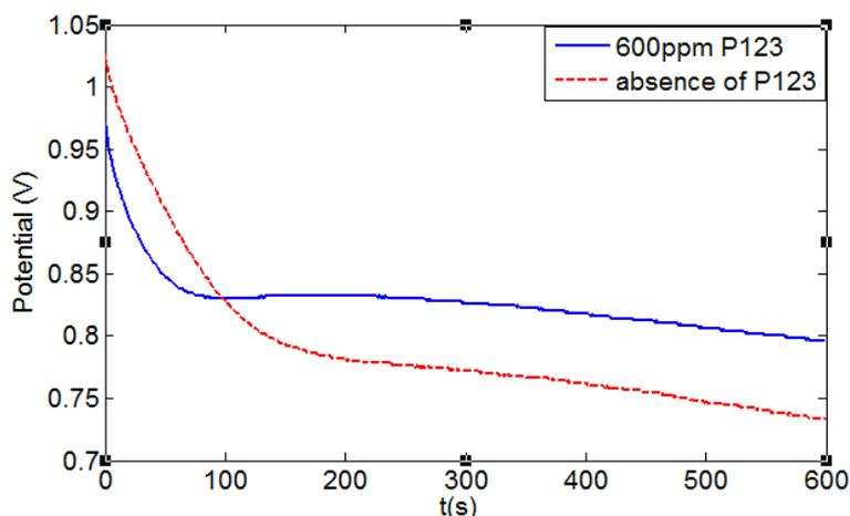
**Fig. 5.** the discharge cycles for Zn/CuO battery with and without P123
