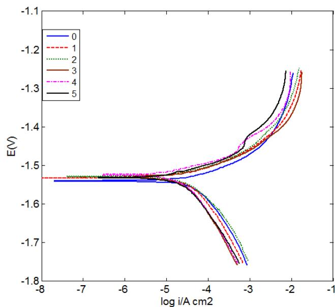
**Fig. 1.** The potentiodynamic polarization curves of Zn electrode in a 4.0 mol L<sup>-1</sup> NaOH solution presence variety values of P123 0: blank, 1:75, 2:150, 3:300, and 4:450 and 5:600 ppm P123
