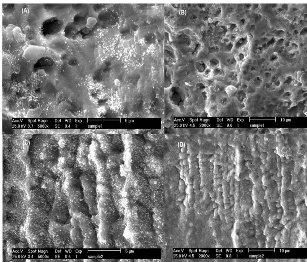
**Fig. 4.** The SEM images of the zinc electrode surfaces with (A and B) and without (C and D) the inhibitor
